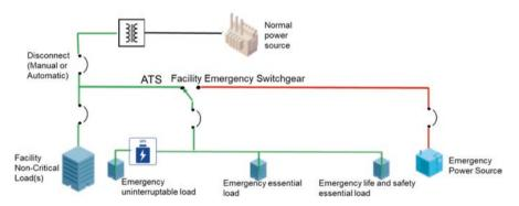
Fig. C.1 Schematic of the one-line diagram for a notional facility
