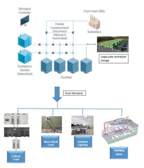
Fig. F.16 Microgrid with centralized emergency generators and a centralized storage
