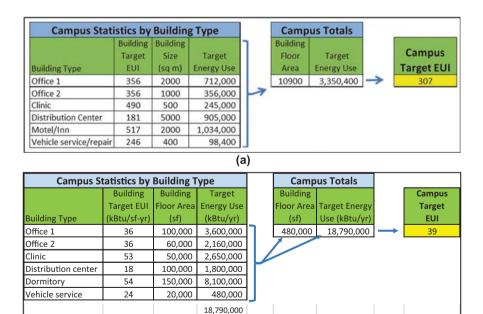
Fig. 4.1 Example of determination of an energy use target for a campus. (a) Systeme Internationale (SI) units. (b) IP units
