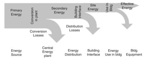
Fig. 3.5 Energy supply chain from primary energy to its use inside a building. (Zhivov et al. 2015)
