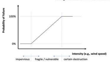
Fragility Curve in Concept: Maps Failure Probability to Various Damage Intensities From the Scenario...
