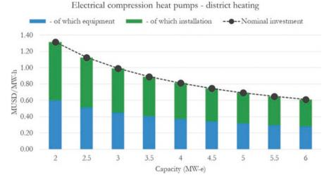
Fig. F.45 Nominal investment of electrical compression heat pumps-district heating
