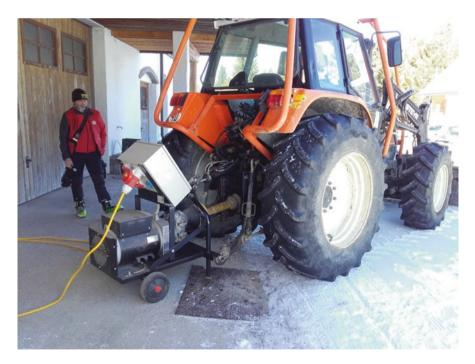
**Fig. B.7** Tractor providing power to a mountain resort during 3-hour blackout. This is a typical mobile backup method used in agricultural and sparsely populated areas (February 2020, Sommeralm in Austria. Source: AEE INTEC)
