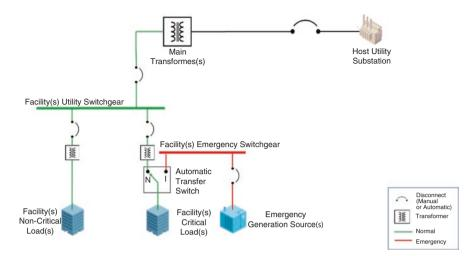
Fig. 7.9 Emergency generator serving mission-critical facility load
