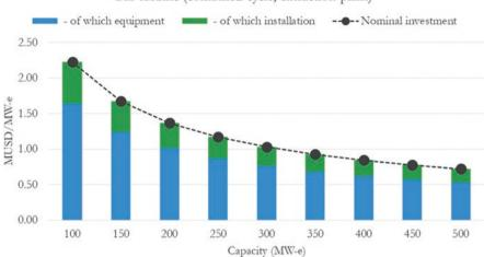
Gas turbine (combined cycle, extraction plant)
