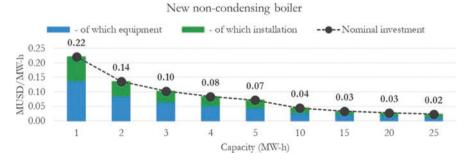
Fig. F.37 Nominal investment by capacity of new non-condensing natural gas boiler
