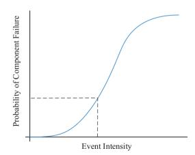
From the probability of failure determined from fragility curves for a designbased threat (event), the resulting probability of component failure (given the event occurrence is above the threshold) indicates that the reliability of the system for that event should therefore be evaluated.
