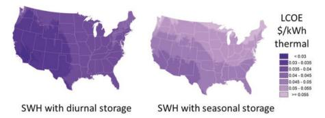
Fig. G.7 LCOE of solar water heating systems varies from less than \$0.03/kWh in the best parts of the sunny Southwest to over \$0.055 in the Northeast and western Washington state
