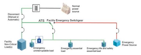
Fig. 5.1 Schematic of the one-line diagram for a notional facility
