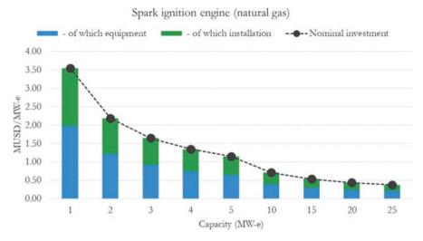
Fig. F.2 Nominal investment by capacity for a spark ignition engine using natural gas
