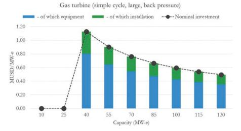
Fig. F.6 Nominal investment for a simple cycle gas turbine (large back-pressure)
