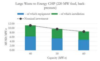
Fig. F.14 Nominal investment for a large waste-to-energy CHP (220 MW feed, back-pressure)
