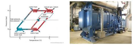
Fig. F.46 Absorption heat pump
