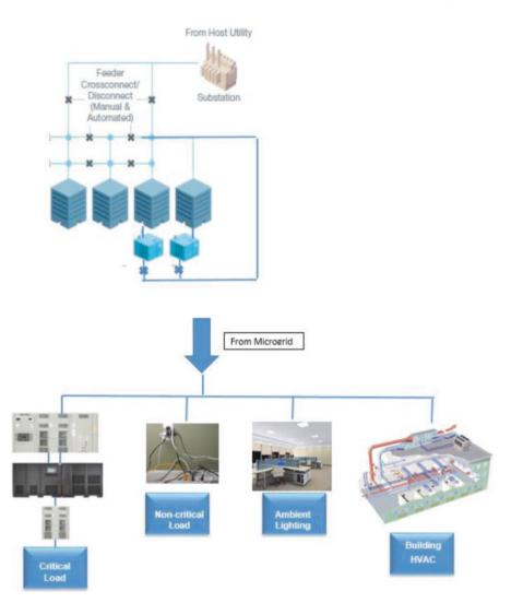
Fig. F.21 Microgrid with decentralized emergency generators
