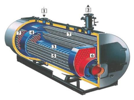
Fig. F.35 Natural gas boiler
