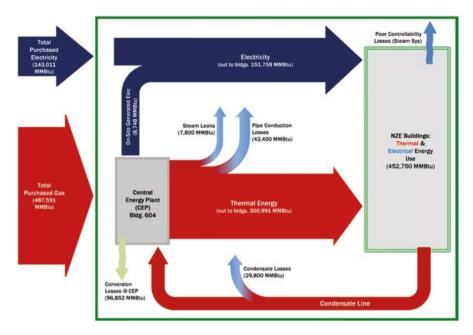
Fig. 3.4 Schematic of Baseline energy uses and wastes at a net-zero energy (NZE) area of one military installation. (Zhivov et al. 2015)
