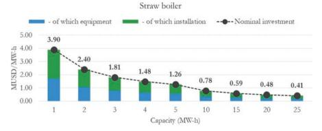
Fig. F.40 Nominal investment by capacity for a straw boiler
