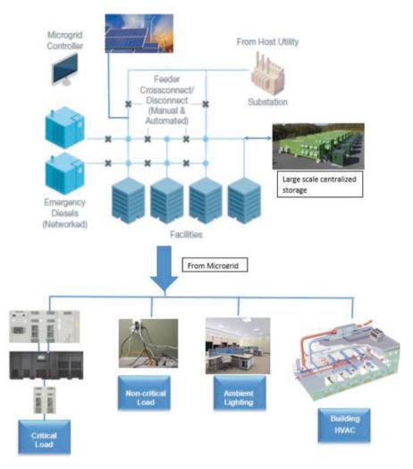
Fig. F.18 Microgrid with centralized emergency generators, RE sources, and a centralized storage
