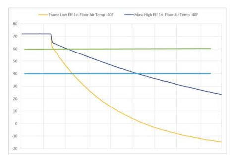
Fig. 5.19 Comparison of indoor air temperature decay in low-efficiency frame building vs. high-efficiency mass building with a heating system failure at outdoor air temperature of -40 °F (-40 °C)
