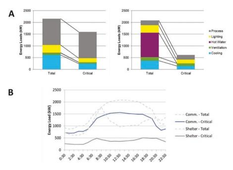
Fig. 3.6 Total and critical electrical demands: (a) total and critical electrical demand load for a data center (left) and a dormitory (right) and (b) critical electrical demand hourly profiles for communications and shelter over a 24-h period
