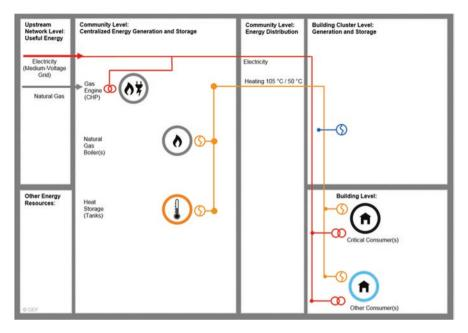
Fig. E.1 Thermal energy system architecture
