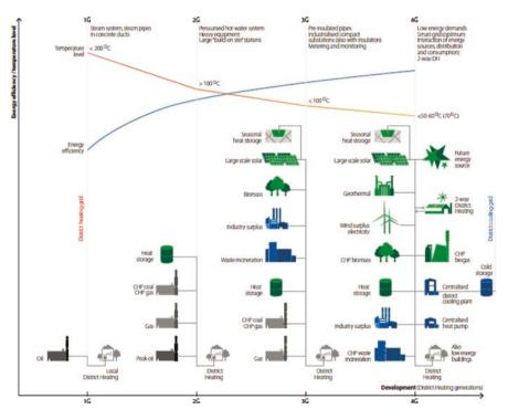
Fig. 7.1 Four generations of thermal district systems. (Reproduced with permission from www.4dh.dk)
