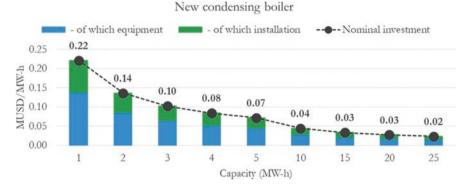
Fig. F.36 Nominal investment by capacity of new condensing natural gas boiler
