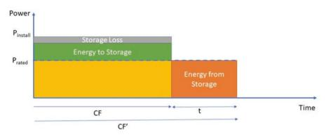
Fig. G.1 Graphical representation of power into storage due to  $P_{install}$ > $P_{rated}$  and resulting hours of energy storage, t
