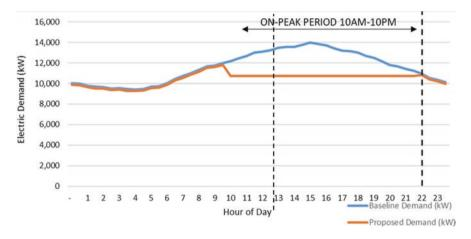
Fig. 1.2 During a peak shaving event, the demand, as seen by the utility, is actively managed by the DERs
