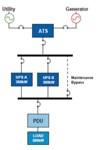
Fig. C.4 Parallel redundant (N+1) UPS configuration. (McCarthy and Avelar 2016)
