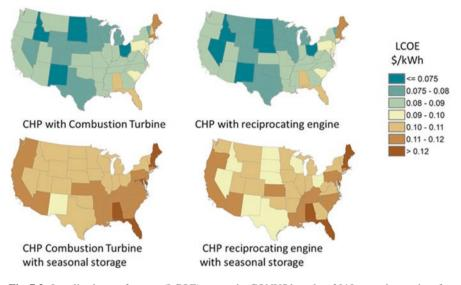
Fig. 7.3 Levelized cost of energy (LCOE) across the CONUS based on 2018 natural gas prices for CHP systems based on combustion turbine and reciprocating engine and with/without seasonal thermal storage
