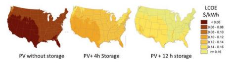
Fig. G.3 LCOE across the Continental United States (CONUS) for photovoltaic systems including 4 hours and 12 hours of battery storage. Costs in sunny areas are on the order of \$0.06/kWh without storage and up to \$0.16/kWh in less sunny areas with 12 hours of battery storage
