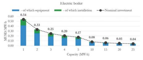
Fig. F.41 Nominal investment by capacity for an electric boiler
