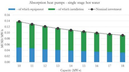
Fig. F.48 Nominal investment absorption heat pumps-single-stage hot water
