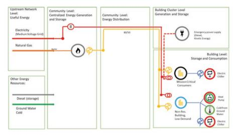
Fig. B.5 Energy system architecture of the University Campus Technik in Innsbruck (AUT). The system is of type 1.3.4
