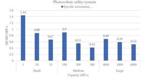
Fig. F.22 Nominal investment for a small, medium, and large residential photovoltaic system
