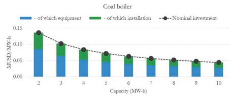
Fig. F.43 Nominal investment by capacity for a coal boiler
