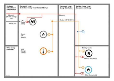
Fig. 7.13 Thermal energy system architecture
