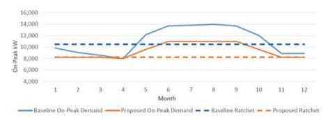
Fig. I.1 Resilient ECMs can use their DERs to lower peak demand and ratchet charges to significantly save energy and provide savings in an ESPC
