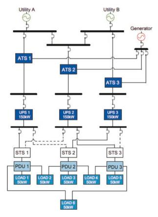
Fig. C.5 Distributed redundant "catcher" UPS configuration. (McCarthy and Avelar 2016)
