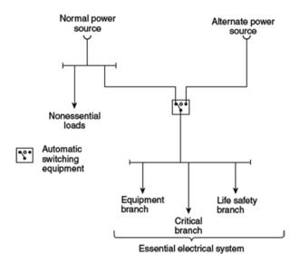
Fig. C.9 Example of a hospital one-line traditional diagram. (Courtesy NFPA 70 [2020])
