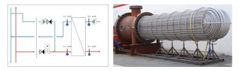
Fig. F.73 Heat exchanger station and bundle-type heat exchanger
