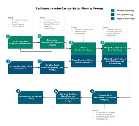
Fig. 3.1 Integration of Energy Systems Resilience Analysis into Energy Master Plan
