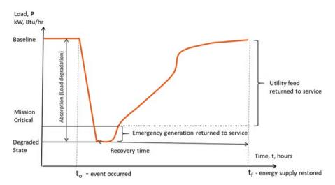
Fig. 5.6 Stepped recovery of power system assets
