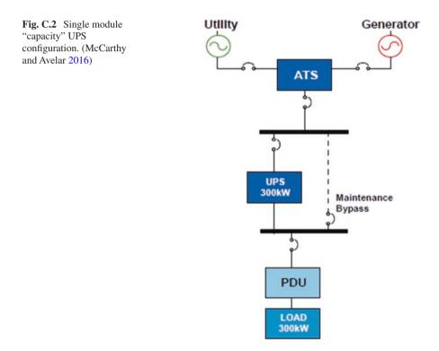
Most "*N*" system configurations, especially under 100 kW, are placed in buildings with no particular concern for the configuration of the overall electrical systems in the building. In general, building electrical systems are designed with an "N" configuration, so an "N" UPS configuration requires nothing more than that to feed it. A common single module UPS system configuration is shown in Fig. C.2.
