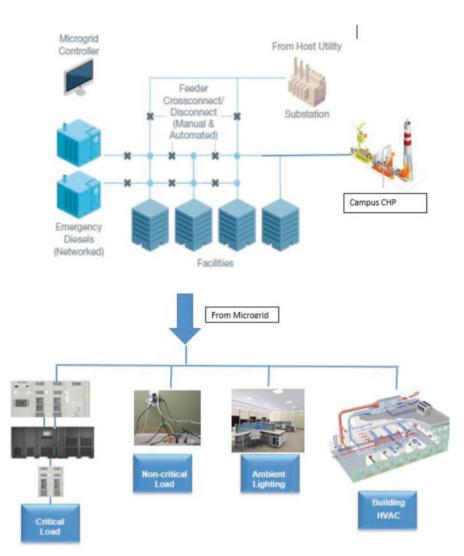
Fig. F.17 Microgrid with centralized emergency generators and CHP plant
