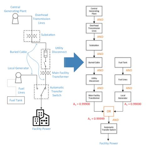
Fig. 5.10 Reliability block diagram for a typical distribution system
