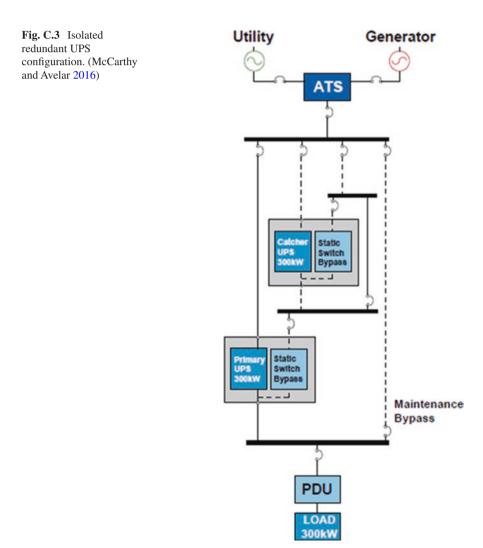
The secondary UPS can also be used to extend the run time of the primary UPS, switching from primary to secondary as the power delivery of the primary is consumed. Additional UPS capability is available for unexpected generator shutdown.
