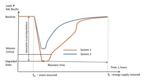
Fig. 5.4 Two systems with different absorption
