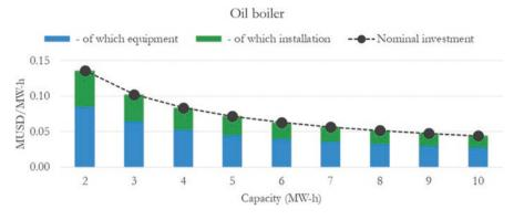
Fig. F.44 Nominal investment by capacity for an oil boiler
