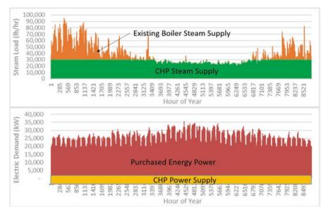
Fig. I.3 CHP resilient solutions generate savings for an ESPC by offsetting heat (steam) and electrical purchases
