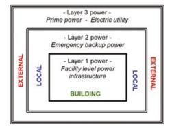
that resides inside the facility. Common components are an uninterruptable power supply (UPS) and an automatic transfer switch (ATS). Layer one backup power is the shortest duration of electrical power capacity of the three layers. The power delivery capacity can typically be from several minutes to several hours.
