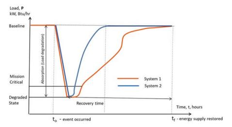
Fig. 5.5 Two systems with different recovery times
