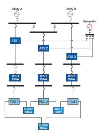
Fig. C.7 Tri-redundant UPS configuration (no STS). (McCarthy and Avelar 2016)
