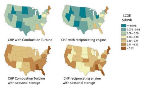
**Fig. G.6** LCOE across the CONUS based on 2018 natural gas prices for combustion turbine combined heat and power systems based on combustion turbine and reciprocating engine and with/ without seasonal thermal storage. Costs vary from less than \$0.075/kWh in Western states where natural gas is least expensive and over \$0.11/kWh in states with higher gas costs in the Northeast. With seasonal storage, the cost varies from \$0.09/kWh to over \$0.12/kWh
