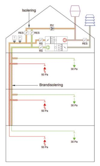
Fig. F.70 Central ventilation with heat recovery
