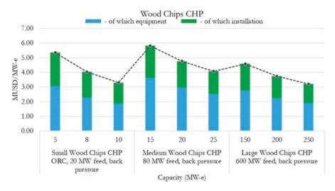
Fig. F.9 Nominal investment for a wood chips CHP (20, 80, 600 MW feed, back-pressure)
