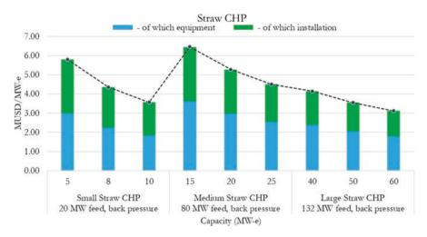
Fig. F.11 Nominal investment for straw CHP (20, 80, 132 MW feed, back-pressure)
