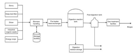
Fig. F.86 Biogas plant
