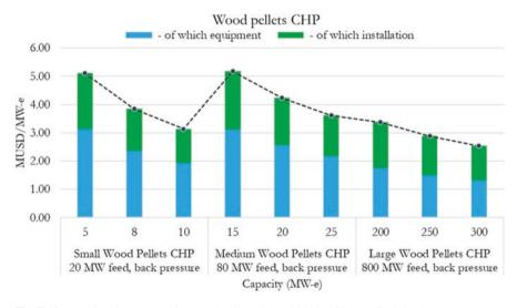
Fig. F.10 Nominal investment for wood pellets CHP (20, 80, 800 MW feed, back-pressure)
