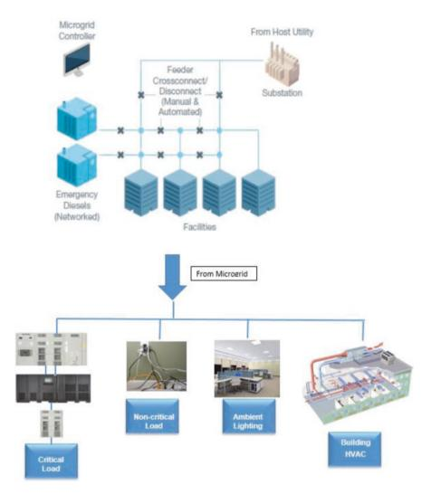
Fig. F.19 Microgrid with centralized emergency generators
