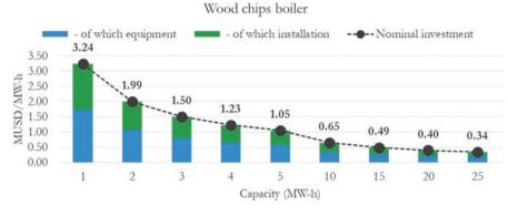
Fig. F.39 Nominal investment by capacity for a wood chips boiler
