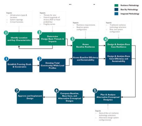
Fig. ES.1 Integration of energy systems resilience analysis into energy master plan
