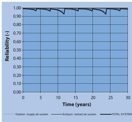
**Figure 21. Comparison of the reliability of a mechanical ventilation system with heat recovery and average quality level with a poor maintenance level.**
