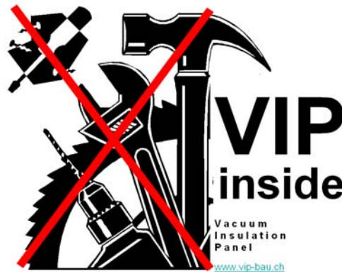
Figure 17: Draft sketch for an adhesive warning label to mark VIP panels and building components containing VIP.
