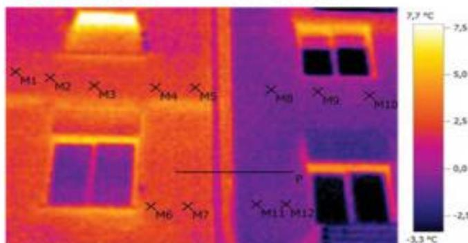
Figure 23: Thermography comparing insulated and not insulated facade.
