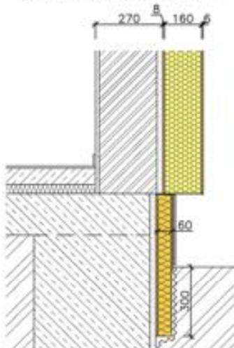
Figure 7: Base of the exterior wall after renovation. Added EPS thermal insulation (beige) is covered by acrylic plaster. The plinth is insulated by XPS (orange), covered by ceramic tiles.
