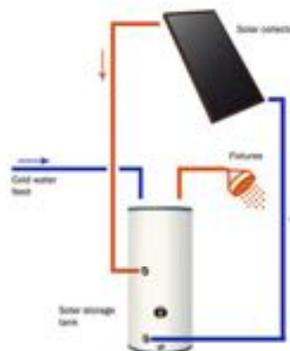
Figure 12: Schematic of the solar water heating system.
