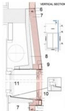
Figure 14: Construction detail D2 & D3. Vertical window section.
