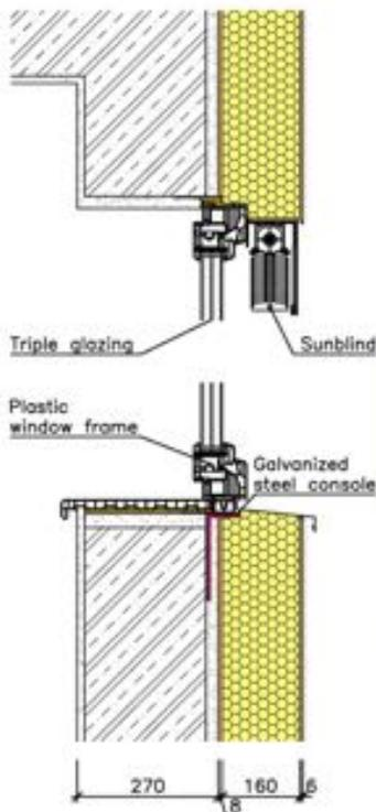
Figure 12: Cross section of the exterior wall and window. Window frame installed on galvanized steel consoles (red) protruding to new EPS thermal insulation layer (beige).
