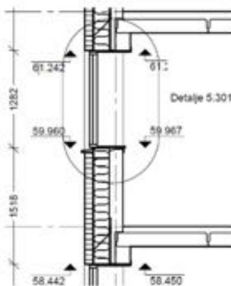
Figure 6 : Wall section: 190 mm new insulation material plus exterior solid standard bricks. Windows – plastic, triple-glazed energy glass.
