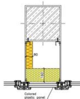
Figure 15: Detail of installation of plastic panel in front of the load-bearing reinforced concrete column. EPS thermal insulation (beige) is installed from the interior side. Acoustic insulation made of mineral wool (orange) is also visible.
