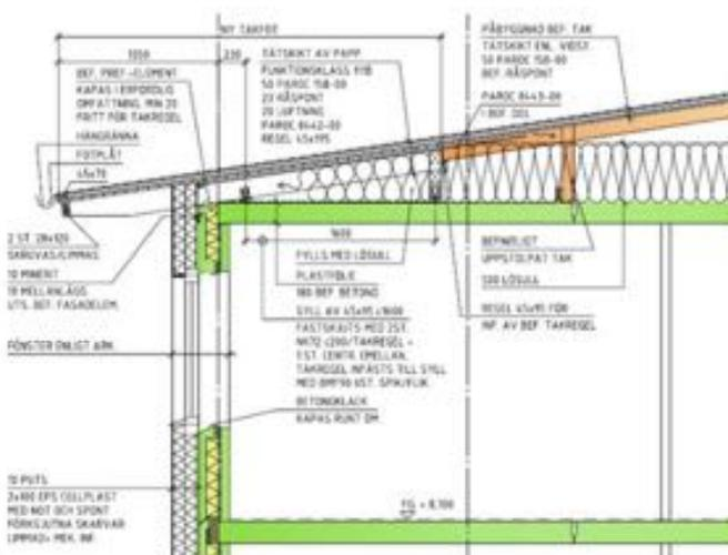
Figure 6: Cross section of exterior wall and roof construction.
