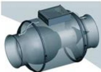
Figure 19: LeanVent damper in closed position - schematic
