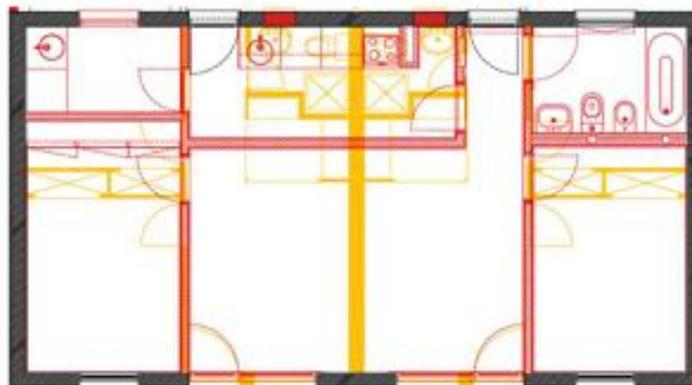
Figure 5: Renovation plans (in yellow demolitions and in red new elements)
