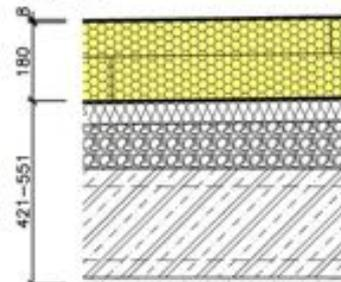
Figure 10: Renovation of the roof. Additional EPS thermal insulation (beige) and modified (SBS) bituminous sheets (black) with mineral granules.
