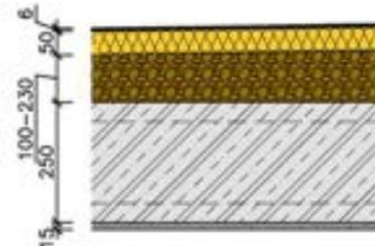
Figure 9: Original roof's composition. Reinforced concrete panels (grey) covered by gravel sloping layer (brown) and EPS thermal insulation (beige). Waterproofing and covering layer was made of bituminous sheets (black) with mineral granules.
