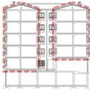
Figure 6: Section, thermal envelope
