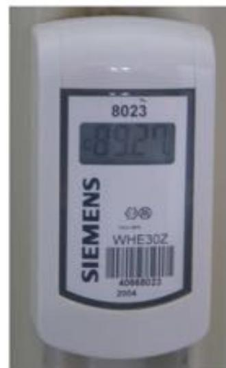
Figure 24: The electronic heat cost allocator
