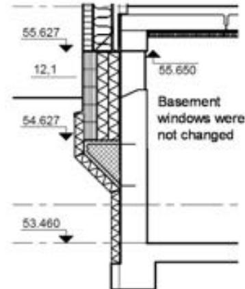
Figure 10: The external insulation is continued to the base of the building to reduce/avoid thermal bridges
