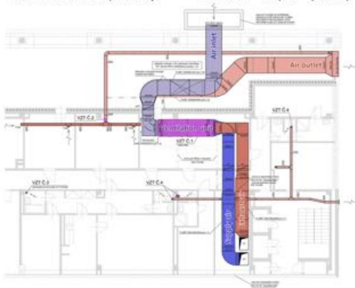
Figure 19: part of the ground plan of the mechanical ventilation in the basement of kitchen and cafeteria block. The ducts are highlighted by colors for better understanding.
