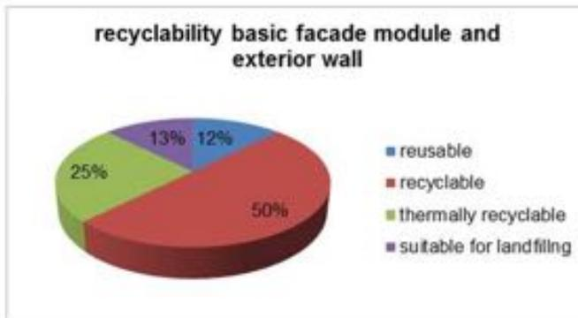
Figure 21: recyclability of device layers in the basic façade module and wall
