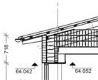
Figure 15: Section showing added roof insulation – new total: 435 mm
