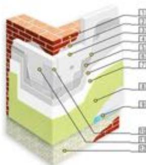
Figure 24: Exterior thermal composite system insulation.
