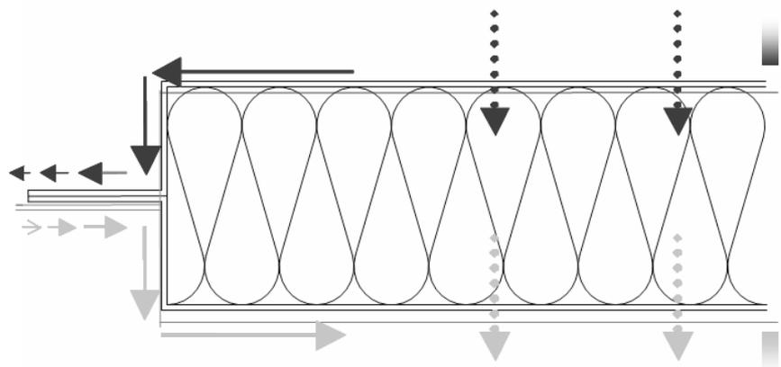
Figure 4: Schematic representation of a cold bridge caused by the VIP envelope.
