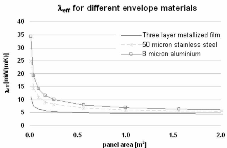
Figure 5: Thermal bridge effect of different envelope materials on overall conductivity ( $\lambda_{eff}$ ) of a panel with center-of-panel conductivity ( $\lambda_{cop}$ ) of  $4 \cdot 10^{-3}$  W/(m·K).
