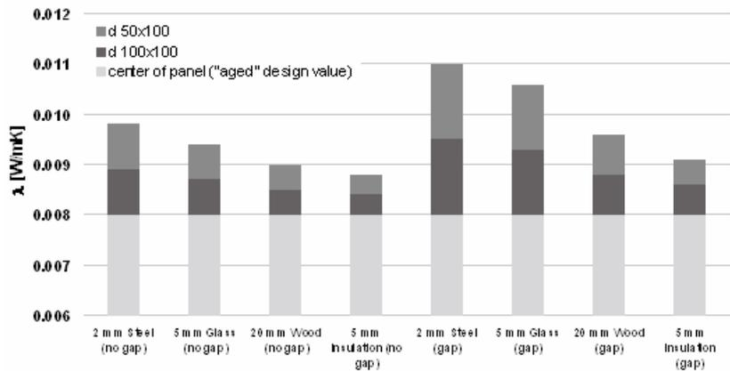
Figure 6: Thermal bridge edge effect of different adjacent materials on overall conductivity ( $\lambda_{eff}$ ) of a panel with MF-envelope and a center-of-panel conductivity of  $8 \cdot 10^{-3}$  W/(m·K). "d 100x100" is the increase for a panel of 100x100 cm<sup>2</sup> compared to  $\lambda_{cop}$  and "d 50x100" is the increase for a panel of 50x100 cm<sup>2</sup> compared to the larger format.
