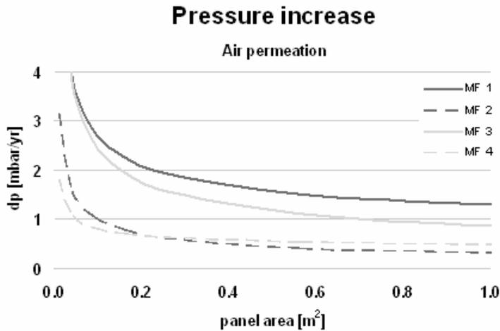
Figure 2: Edge effect on internal pressure increase by air permeation through four different metallized films.
