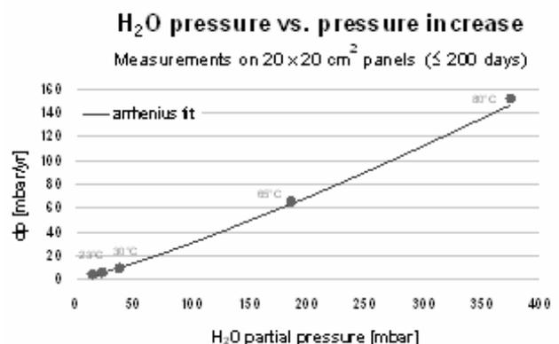
Figure 3: Internal pressure increase caused by water vapour permeation is proportional to the differences in the partial pressures inside and outside the panel. The measurements were done at room temperature after cooling down the samples for some hours.
