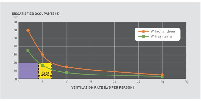
An example of test results, in which the performance of the tested air cleaner is equivalent to 3 l/s per person of clean air, which is called the clean air delivery rate (CADR). Source: Adapted from ICIEE.DTU
