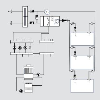
A typical configuration of a centralised HVAC system (heat source, water and air transport, heat emission). Source: EBC Working Group on HVAC Energy Calculation Methodologies for Non-residential Buildings
