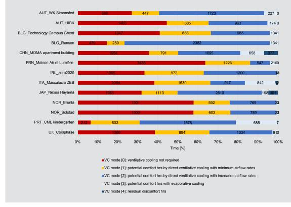
An outcome of the tool, the ventilative cooling (VC) potential of the project case studies divided into the different ventilative cooling modes. Results differ even for buildings within the same climate because of their different usage characteristics. Source: EBC Annex 62
