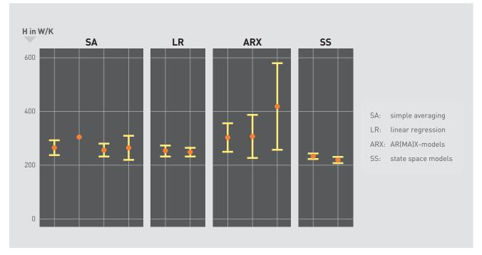
Early results based on in-use data for different methods to determine the actual heat loss coefficient (H) for a poorly insulated dwelling in Loughborough, UK. Since a wide spread in the results has been observed, the project is investigating possible causes in detail including the impact of pre-processing the data, selection of data subsets, impact of internal and solar heat gains, and so on. Source: Adapted from EBC Annex 71
