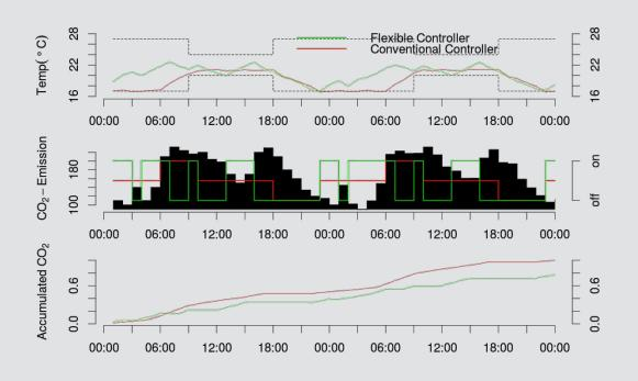
Top plot: The room temperature in a building is controlled by a penalty-aware controller (green line), or a conventional controller (red line). Both controllers are restricted to stay within the dashed lines.
