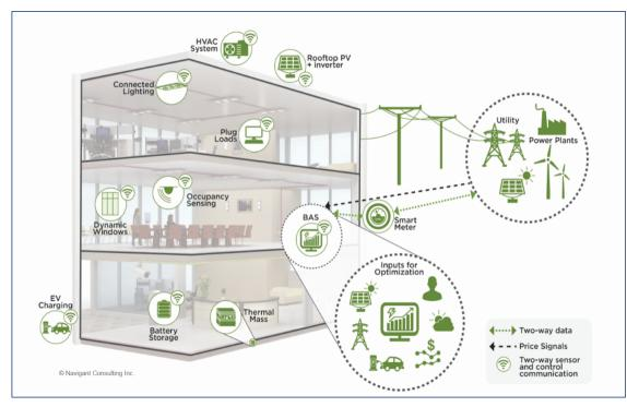
Example of a Grid-interactive Efficient Building (GEB) communicating with the utility.
