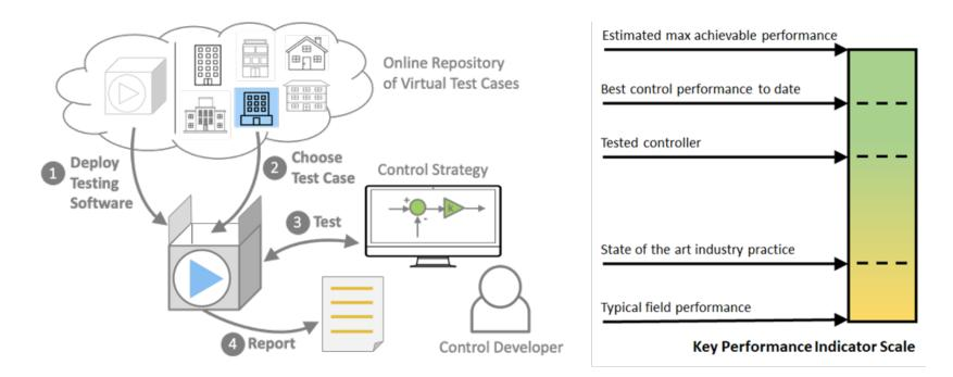
The BOPTEST (Building Operations Testing) Framework is a set of simulated buildings and a standard API for manipulating their sensor and actuator "control points" for comparing and benchmarking the performance of control and FDD algorithms.
