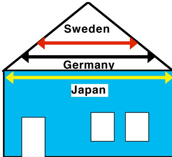
Figure 1. Different definitions of attic floor area
