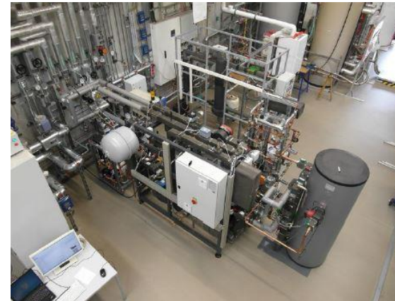
Decentral feed-in (between supply and return flow)
