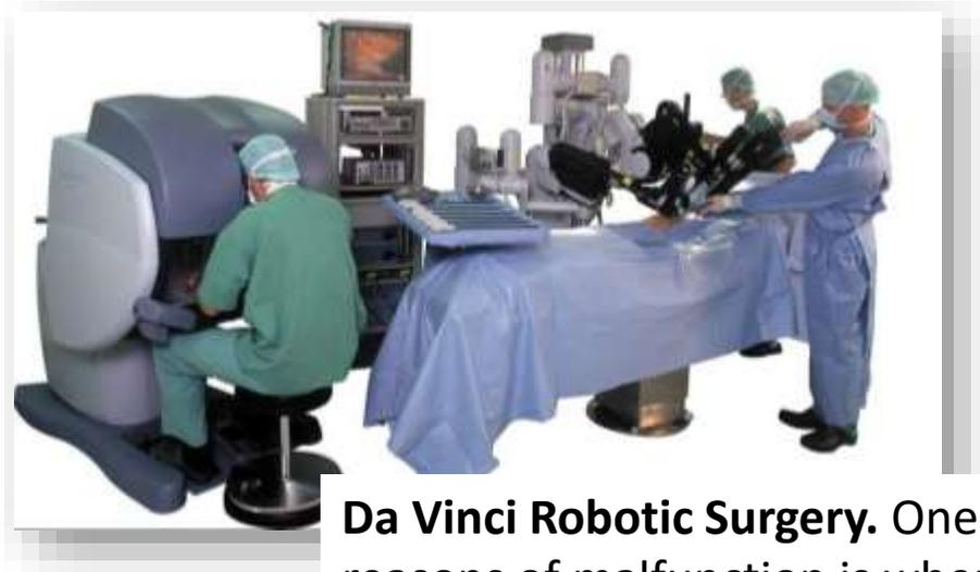
**Da Vinci Robotic Surgery.** One of main reasons of malfunction is when power supply voltage is out of range.
