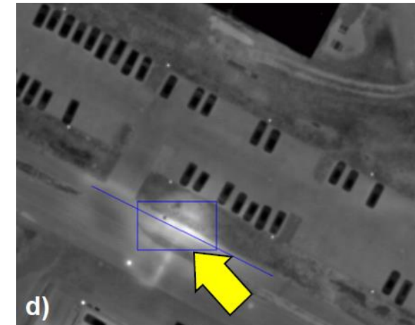
c) and b) Thermographic imaging of a leakages Source: Termisk Systemteknik
