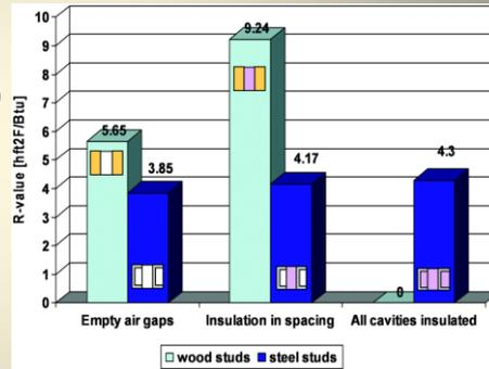
Calculated clear wall R-values for wood and steel framed walls
