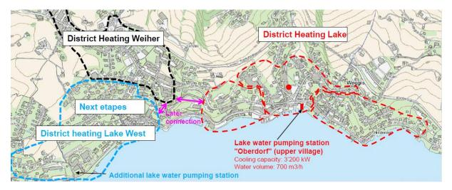
Figure 1. Schematic view of the different stages of the district heating networks in Weggis (Source: Corporation Weggis).
