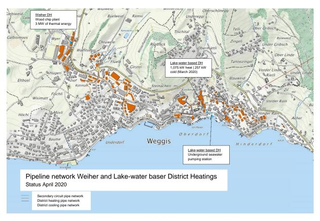
Figure 2. Schematic view of the buildings connected in April 2020 and of the existing pipeline network (Source: Corporation Weggis).
