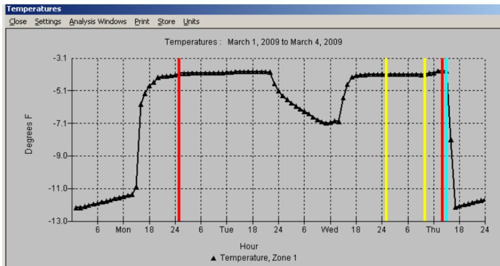
Figure 24. Evolution of temperatures during a PSTAR test
