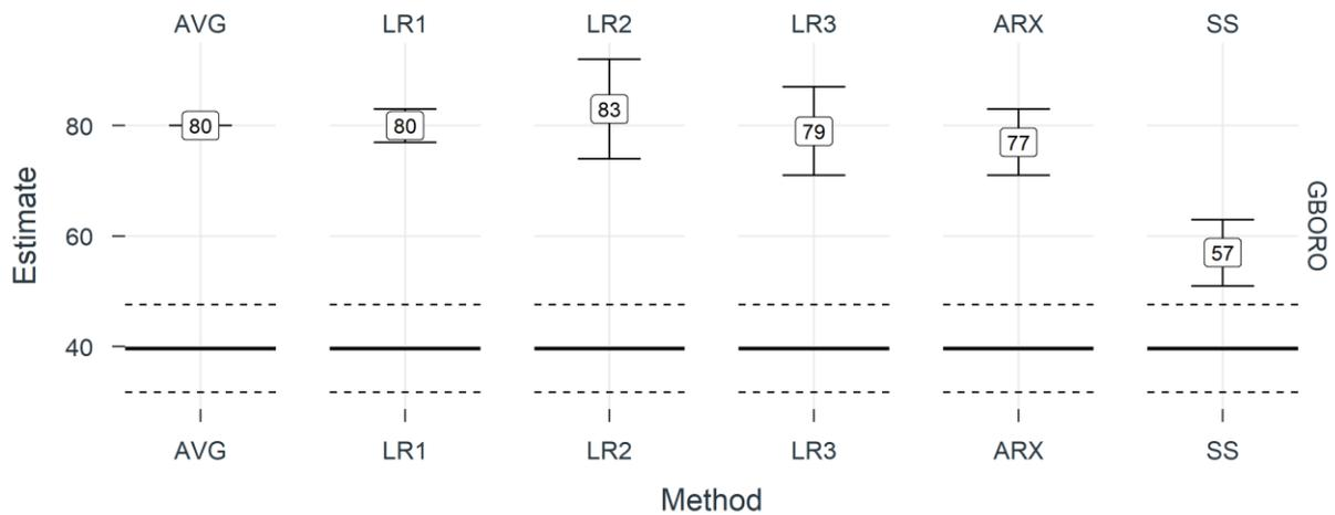
Figure 17. Results for optimal combination of approaches for Gainsborough. The calculated reference value for HTC is indicated as a horizontal thick line, and a 20% deviation above and below as dashed lines.
