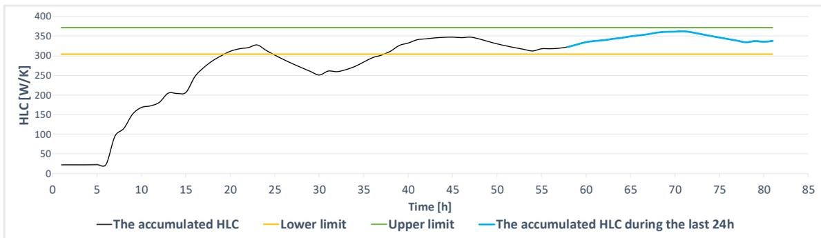
Figure 28. Example of the evolution of the accumulated Heat Loss Coefficient for a cold and cloudy 82 hour period for a whole building.
