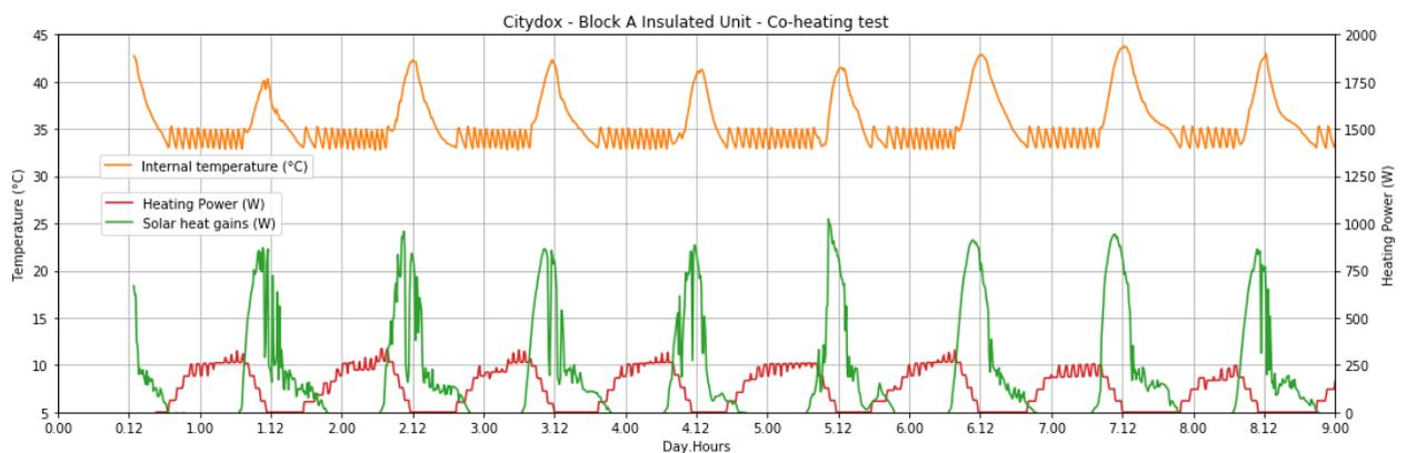
Figure 26. Time series chart of power input, solar heat gains and internal temperature for a typical CAM(B)BRIDGE test
