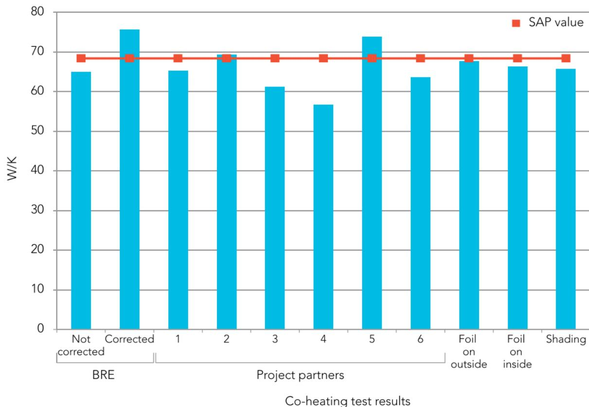
Figure 3. Results of a campaign of coheating test carried out on the same property by different researchers (Butler & Dengel, 2013)
