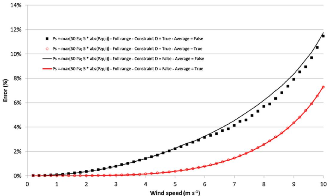
Figure 5. An example of the maximum error found due to wind speed. (Carrié & Leprince, 2016)
