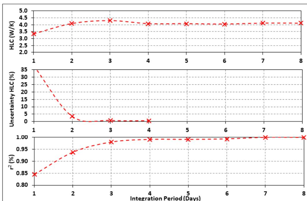
Figure 29. Dynamic Integrated Method. HTC and validity indicators for different integration periods.
