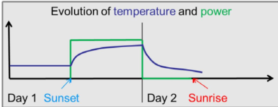
Figure 21. Time series chart of power input and internal temperature for a typical QUB test
