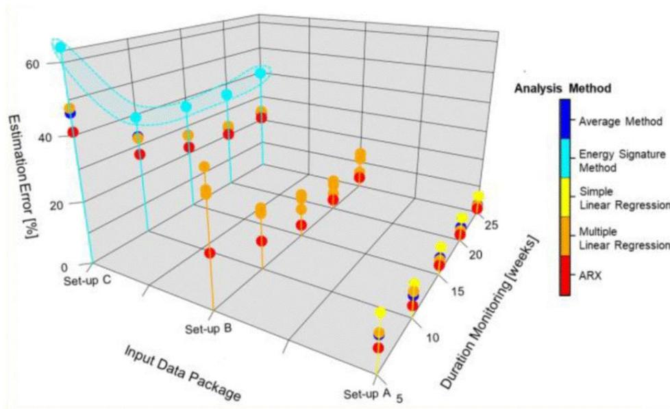
Figure 15. 3-dimensional decision matrix, presenting expected estimation monitoring error for different statistical methods, considering (predefined) data packages and monitoring time.
