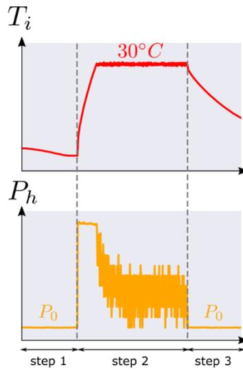
Figure 22. A typical testing cycle for the ISABELE protocol (Thébault & Bouchié, 2018)
