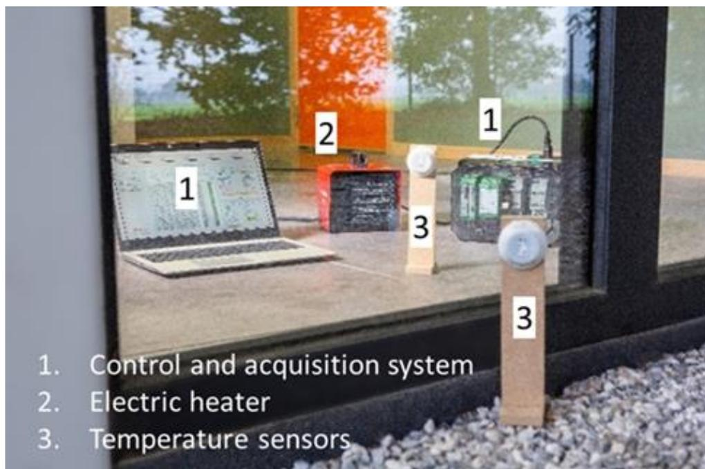
Figure 32. Equipment used in CoDY Test
