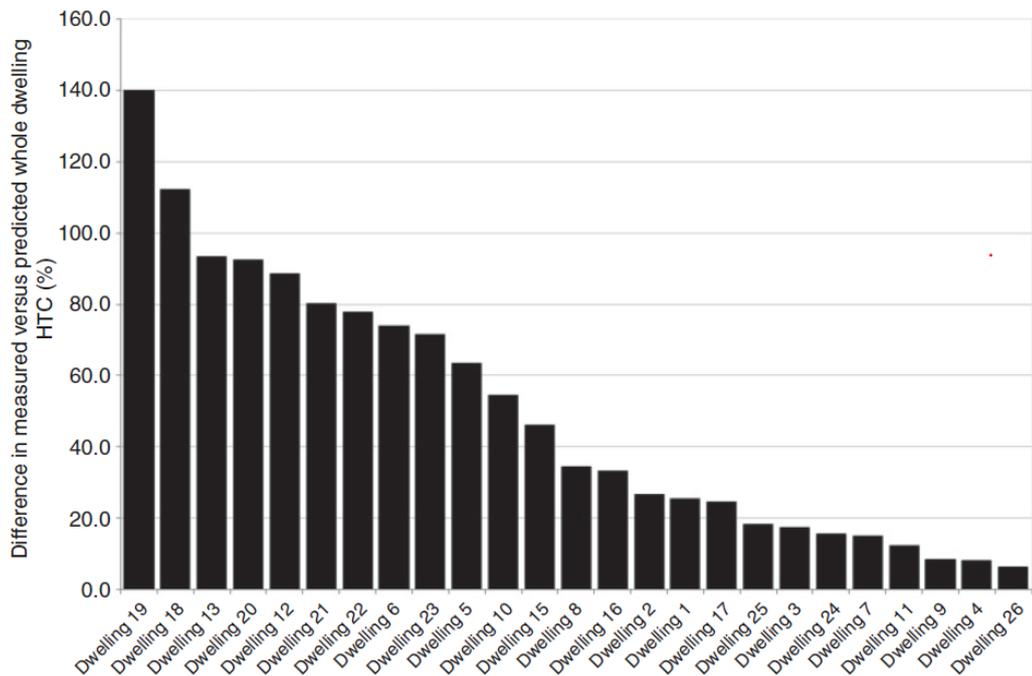
Figure 1. Results from a campaign of HTC (Heat Transfer Coefficient) measurement, illustrating the EPG in a sample of new build homes in the UK (D Johnston et al., 2015).
