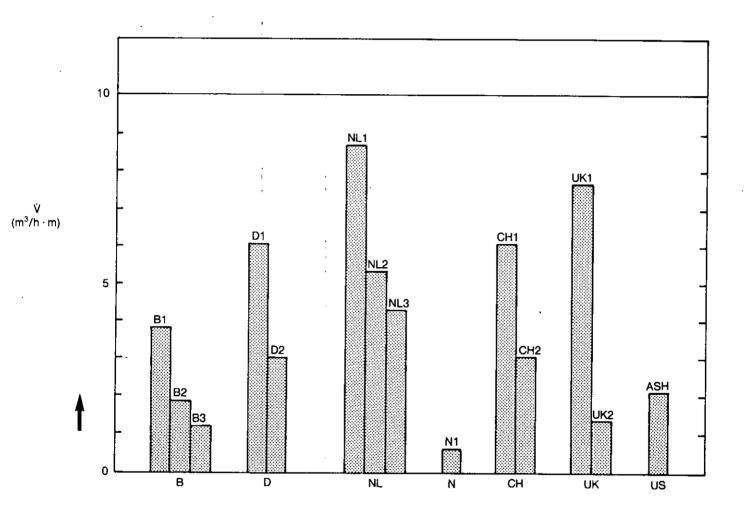
V: maximum air leakage per m¹ crack at 50 Pa pressure difference N.B.: maximum air leakage rates at pressure differences other than 50 Pa have been transformed to 50 Pa, using the relation: V(50) = V(P1)\*(50/P1)<sup>n</sup>; in all cases here n=2/3
