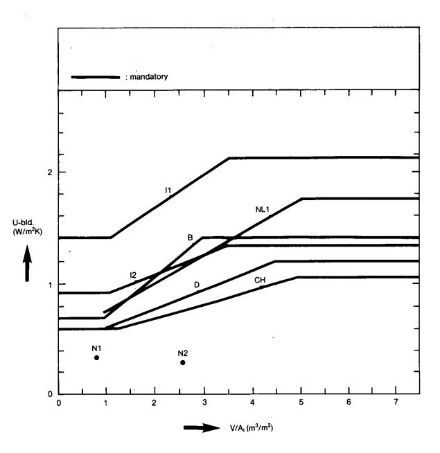
U-bld.: maximum mean U-value of the building V/A<sub>t</sub>: ratio of building volume and total heat loss area
