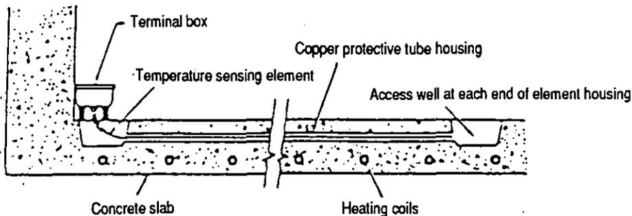
Fig. 4.10 An Example of Burying a Sensor into the Ground or a Concrete Slab
