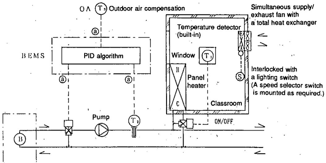
Fig. 9.1 Schema of Temperature and Ventilation Control
