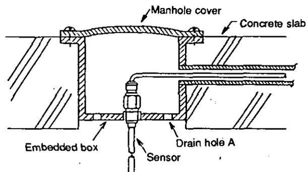
Fig. 4.9 A Mounting Example Inside a Manhole
