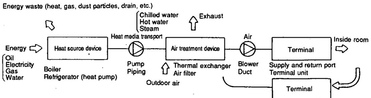
Fig. 4.2 Basic Airconditioning Equipment Configuration JN 2)
