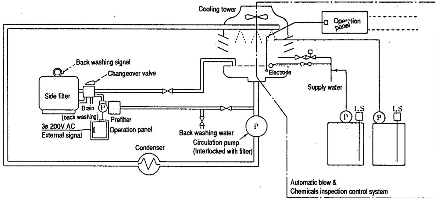
Fig. 5.1 An Example of Automatic Cooling Water Control System
