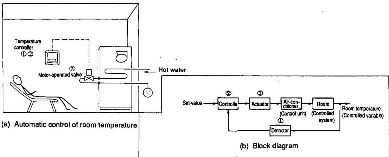
Fig. 2.1 An example of Control Systems (Feedback system) <sup>JN 12)</sup>
