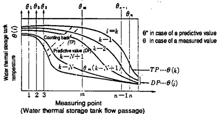
(d) Water thermal storage tank temperature profile and its calculation
