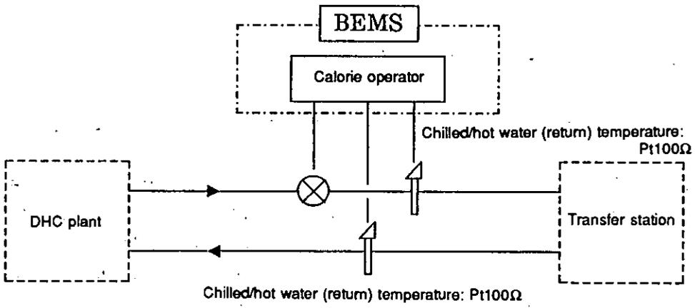
Fig. 9.14 Heat Flow Measurement in a District Cooling/Heating, Chilled/Hot Water Transfer Station Facility
