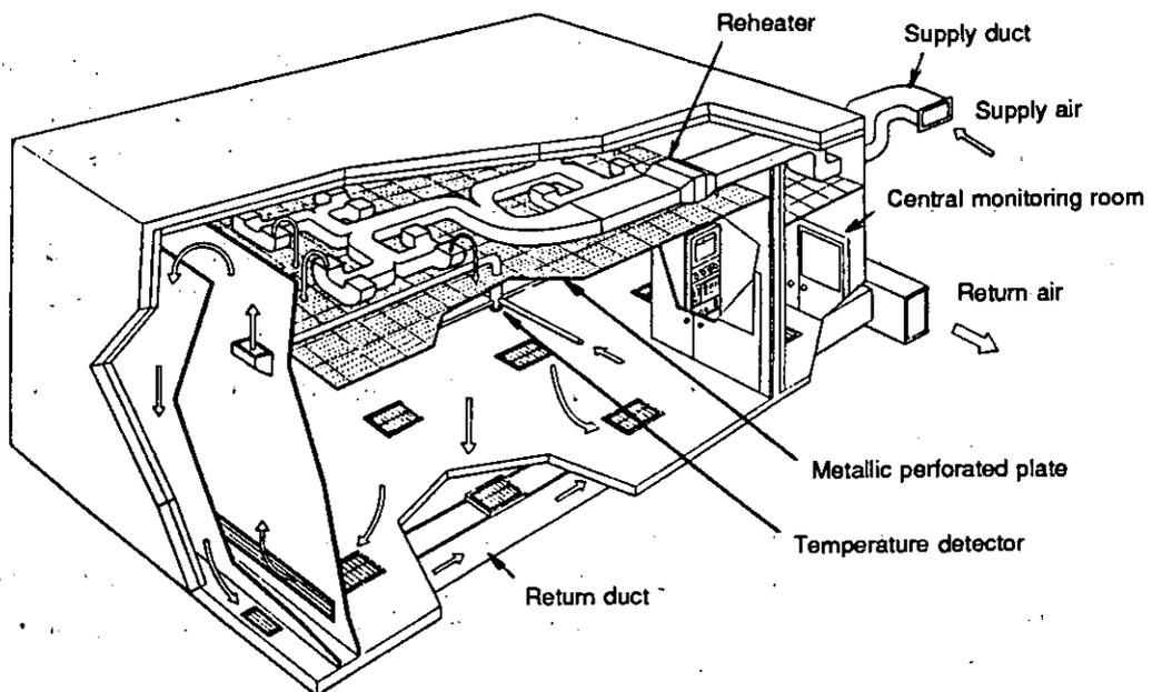
Fig. 9.8 Sectional Perspective Drawing of Thermostatic Room <sup>JN 6)</sup>
