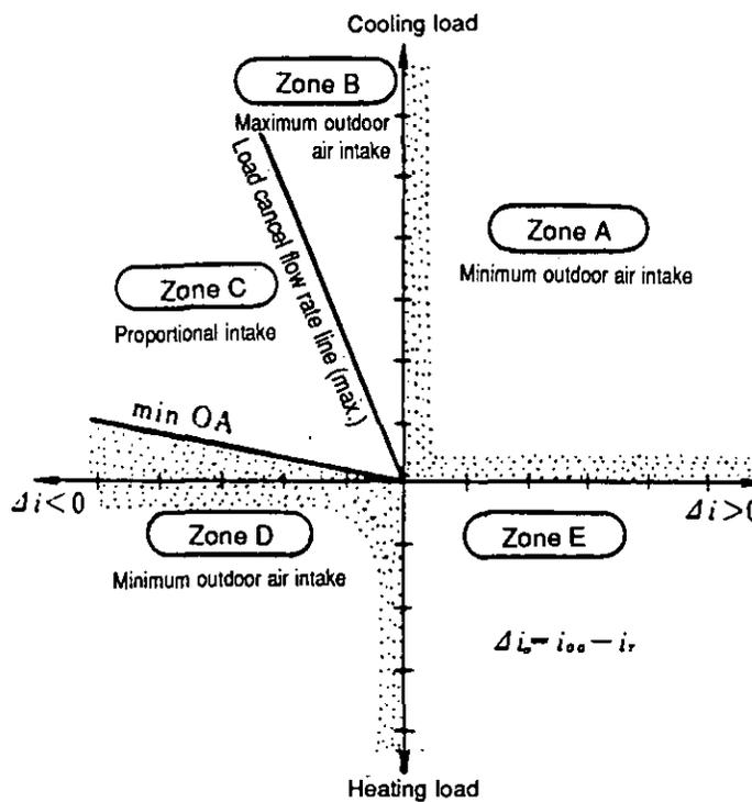
Fig. 4.7 Outdoor Air Intake Strategy in Airconditioning <sup>JN 2)</sup>
