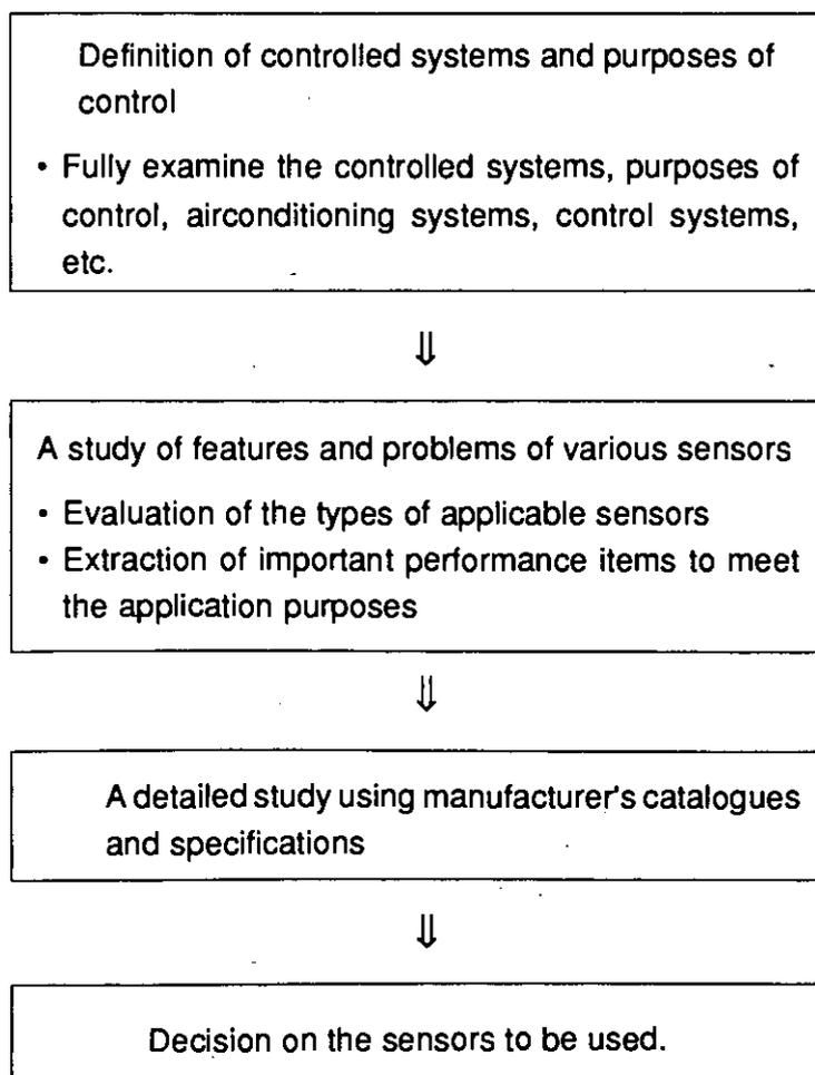
Fig. 4.3 Sensor Selection Procedure
