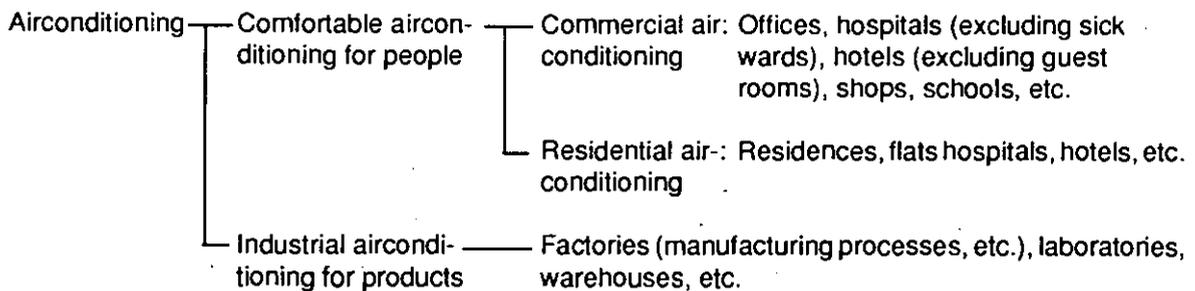
Fig. 4.1 Classification of Airconditioning
