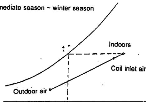
No cooling signal is issued, if the dew-point temperature of the coil inlet air is lower than a set point variable.
