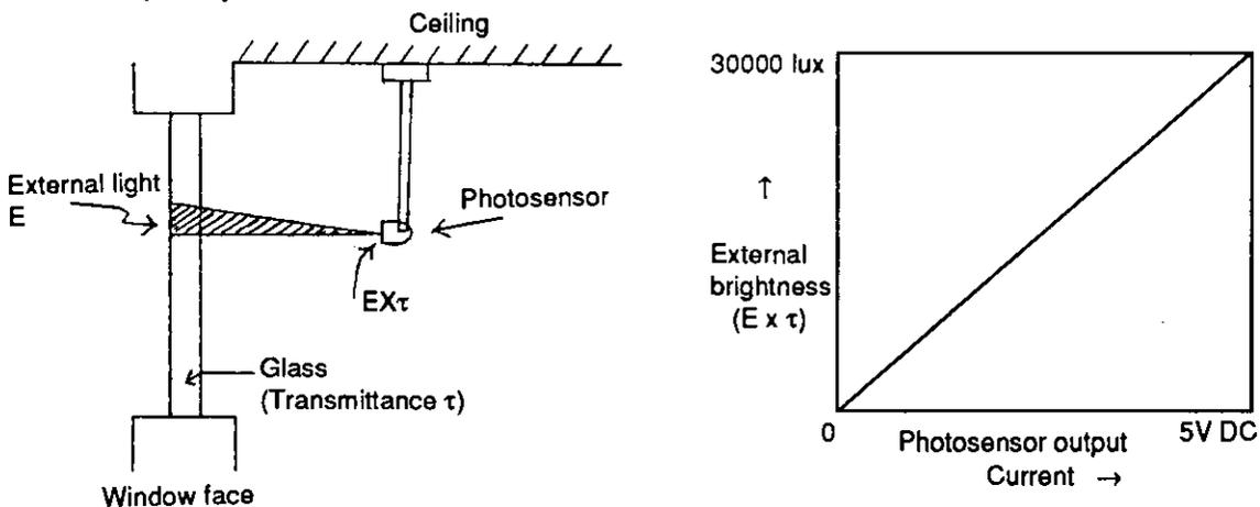
\* Light is converted into a current through an internal photocoupler of the photosensor.
