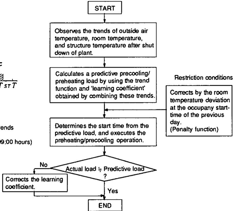
(b) Outlined optimization flow of preheating/precooling operation
