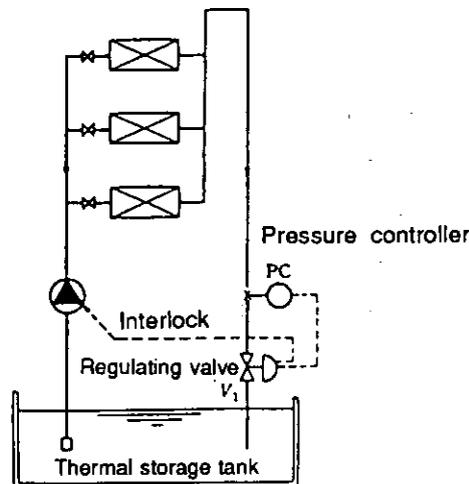
Fig. 4.14 Return Water Pressure Control <sup>JN20)</sup>
