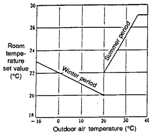
Fig. 4.3 Outdoor Air Temperature Compensation Schedule <sup>JN 32)</sup>
