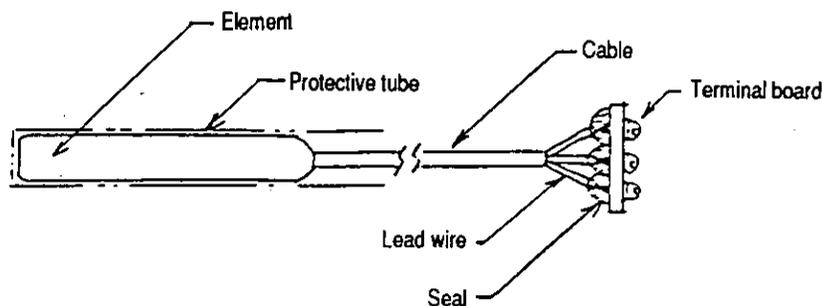
Fig. 4.6 Example of a Sealed Sensor Terminal Ass'y
