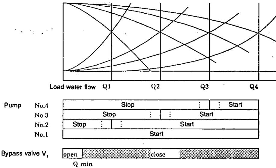
Fig. 9.6 Pump Characteristics and Sequence Control
