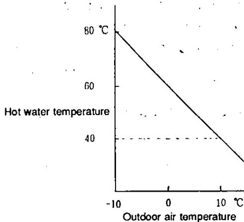
Fig. 9.2 Outdoor Air Temperature Compensation Example
