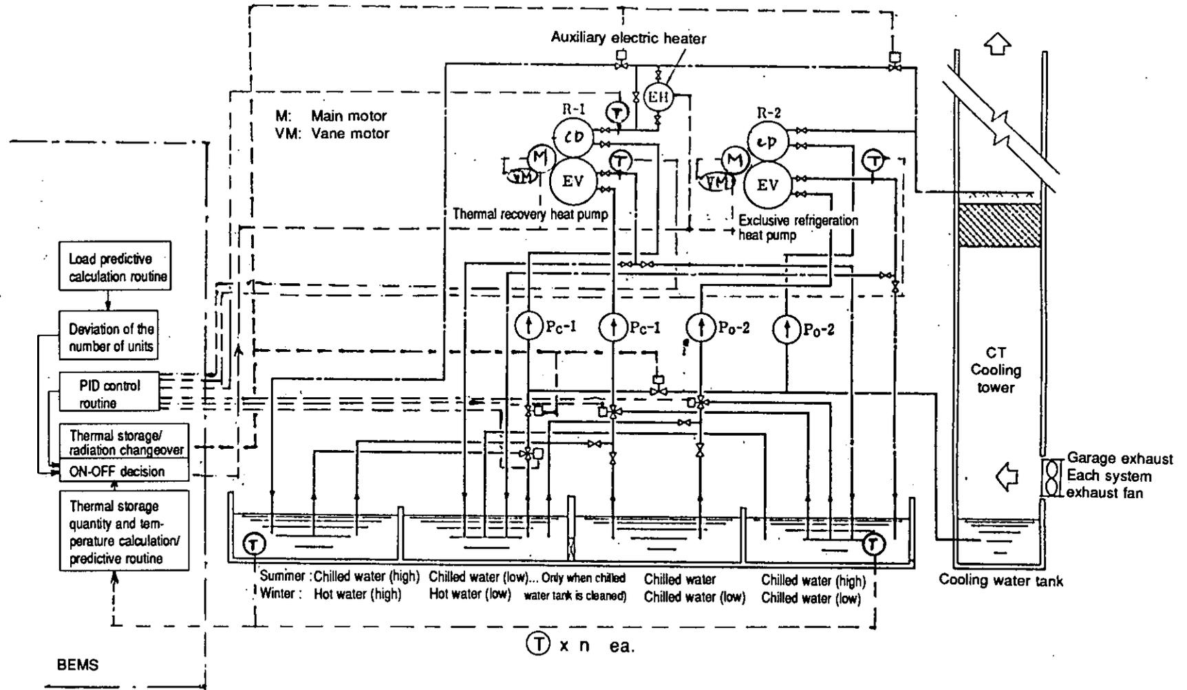
Fig. 9.12 Heat Pump Sequence Control Block Diagram
