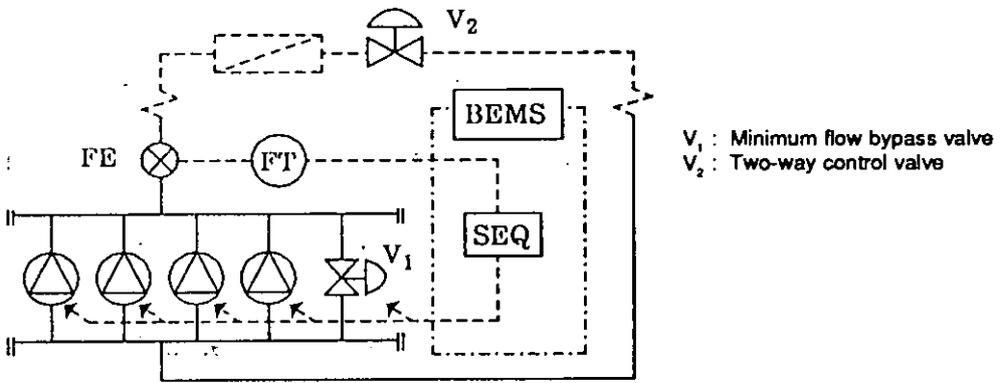
Fig. 9.5 Sequence Control Diagram
