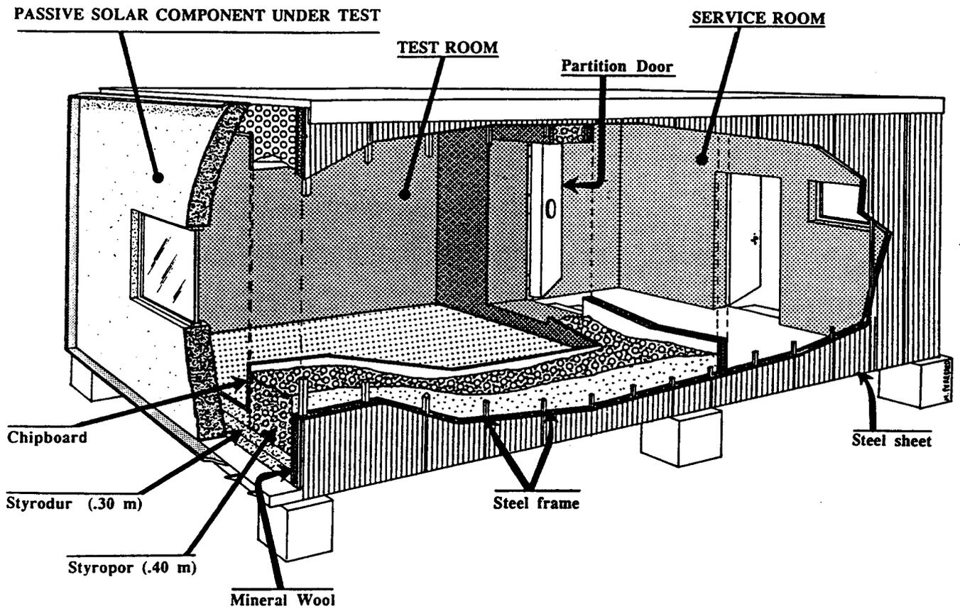
Fig. 8. Sketch of the PASSYS test cell
