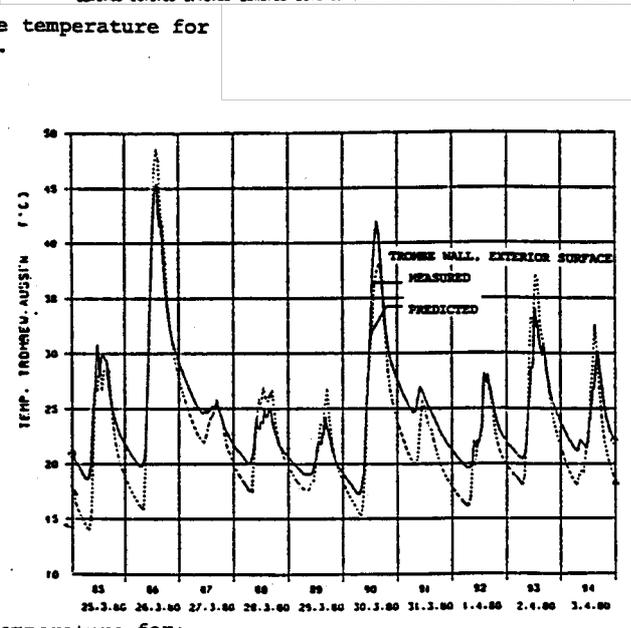
Fig. 5 Trombe Wall Cell Predictions for BFEP and SERIRES
