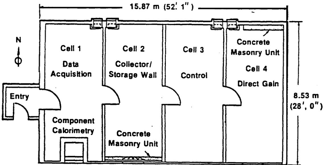
Fig. 14. Floor plan of the NBS passive solar test building
