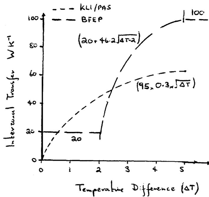
Fig. 3 Inter-zonal Conduction Modes Invented for the Los Alamos Cells
