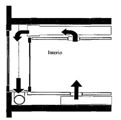
Figure 6.3 Schematic diagram of an 'active window' system
