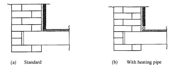
Figure 5.4 Junction between masonry wall with internal insulation and timber floor
