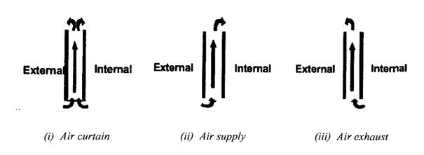
Figure 6.2 Possible air flow arrangements in an active envelope
