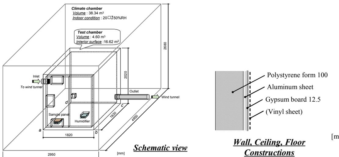
**Figure 2. Experimental set-up used in Common Exercise 2.**
