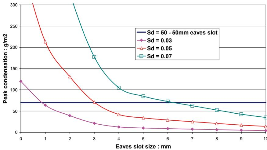
Figure 5 . peak accumulated condensate as a function of eaves gap and underlay resistance.
