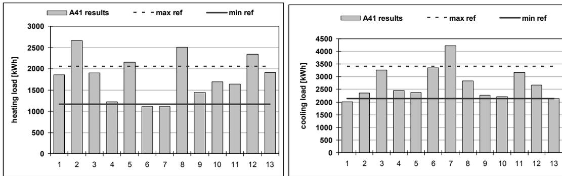
**Figure 1. A comparison of annual net energy demand for heating and cooling for heavyweight structure building between various models in Common Exercise 0. The dotted and the full lines give the simulated maximum and minimum values from Annex 21.**
