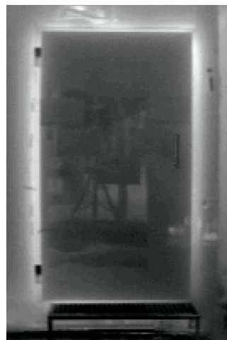
Figure 3.2c. Infrared picture of the test cell door.
