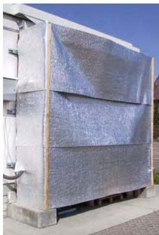
Figure 4.1a. Photograph of test toom with external chamber.
