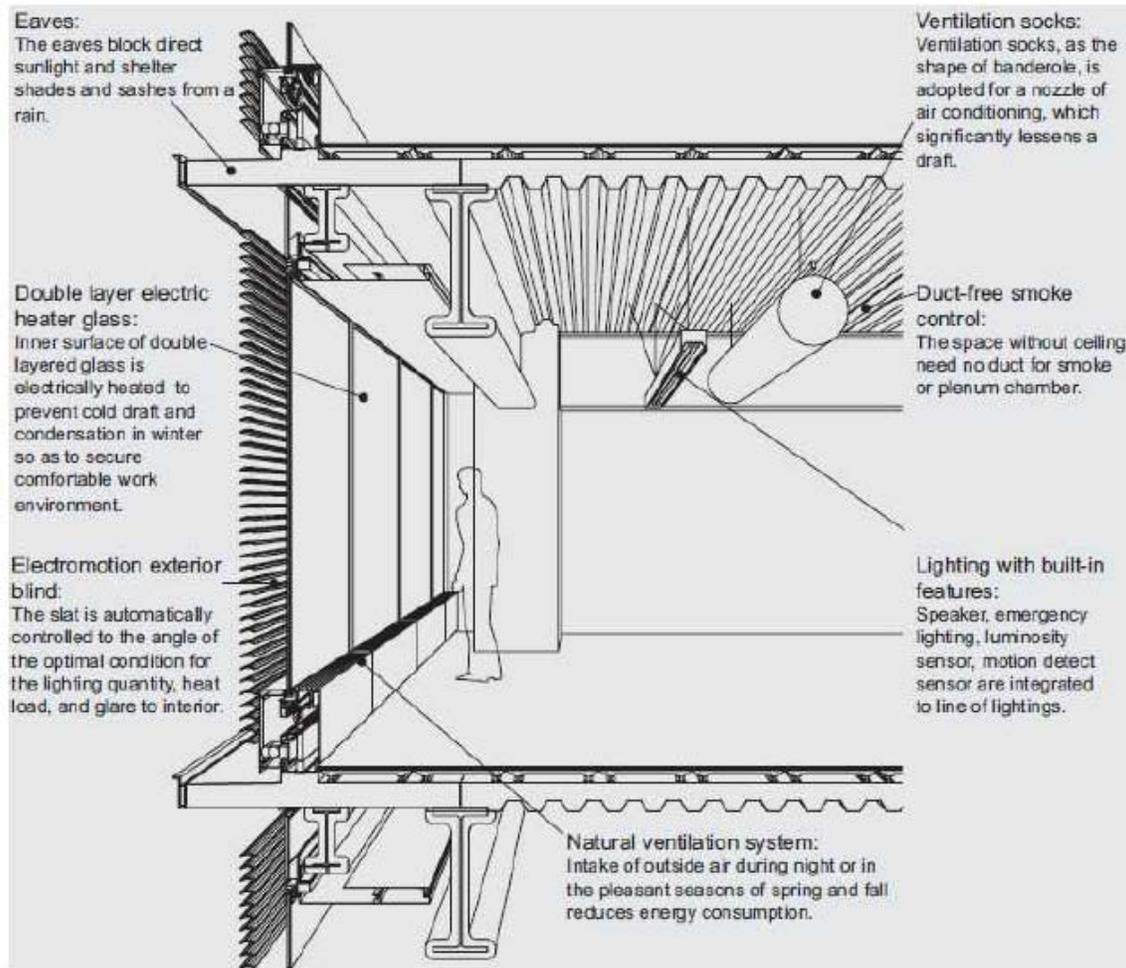
This window system can achieve the energy saving while securing the view and the open plan in response to the change of outside environments of shooting and the outside temperature, etc.
