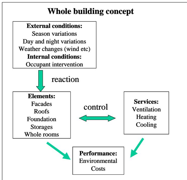
Illustration of the integration between building elements, indoor and outdoor conditions, controls, and performance (Illustration: Åsa Wahlström).
