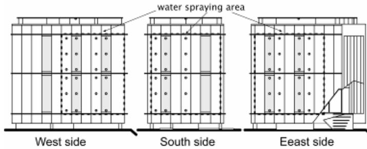
East-south view of the experimental building and west, south and east view of it. The outer surfaces of the exterior walls and glass panes were all coated with photo-catalytic material. Water was sprayed on the wall and glass surfaces at west, south and east.
