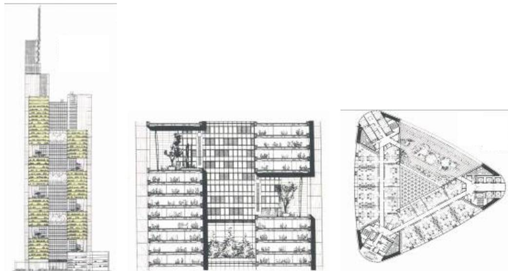
The illustration shows a typical office floor, a vertical section of the building and a segment of the vertical section. This gives an idea of how the atrium and the winter-gardens are placed in the building. The atrium is placed as a vertical core in the centre of the building, connecting the four storey winter-gardens and ensuring ventilation. [Need permission](#)
