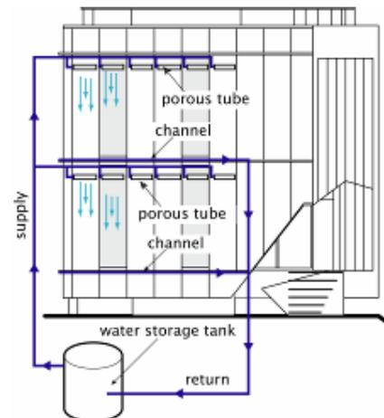
Water spraying system installed at the experimental building. The same water supply and return system shown above was also installed at the east, south and west facade.
