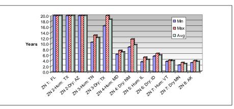
Figure 6.43. Spray foam estimated payback for high, low and medium energy rates.
