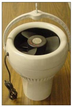
Figure 7.42. A destratification fan.
