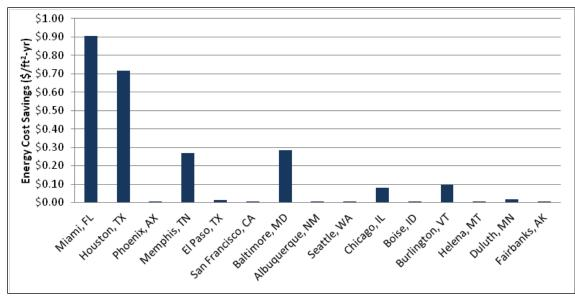
Figure 4.80. Annual energy cost savings for reheat using condenser waste heat.
