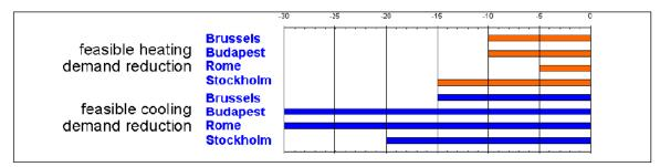
Figure 6.153. Reduced heating and cooling demands predicted from use of external blinds (ESSO Study 9).
