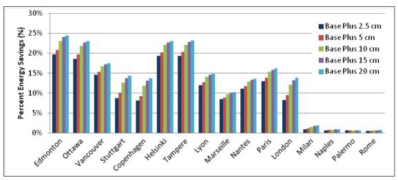
Figure 4.91. Percent energy savings for wall insulation and reduced infiltration over the no-insulation baseline – International locations.
