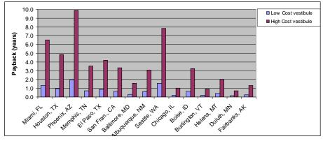
Figure 6.162. Estimated payback for high and low cost dormitory vestibules in the United States.
