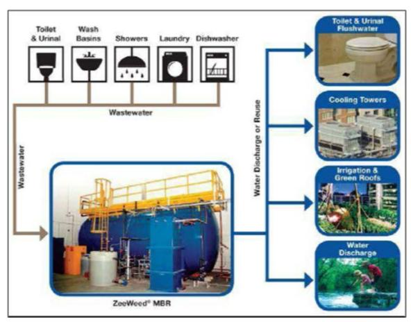
Figure 7.151. ZeeWeed membrane bioreactors (MBRs) treat all grey and black water.
