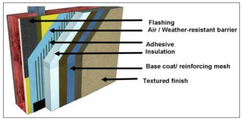
Figure 6.171. EIFS construction with drainage.
