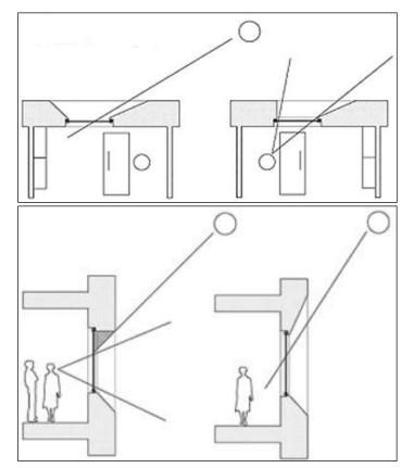
Figure 7.11. Schemes showing the effectiveness of the tilted sides of the windows.
