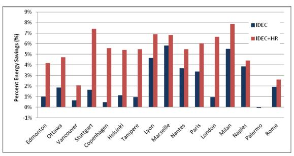
Figure 4.266. Percent energy savings for indirect evaporative cooling and indirect evaporative cooling with heat recovery – International locations.
