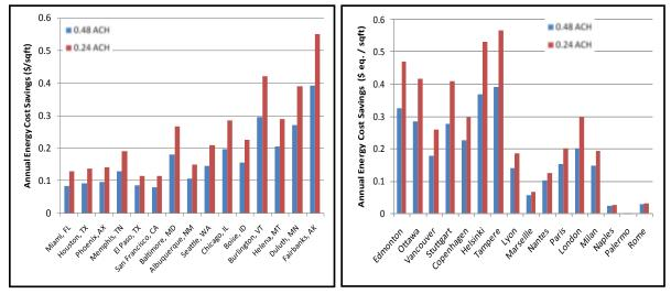
Figure 6.121. Annual energy cost savings per unit area for US (left) and International (right) locations.
