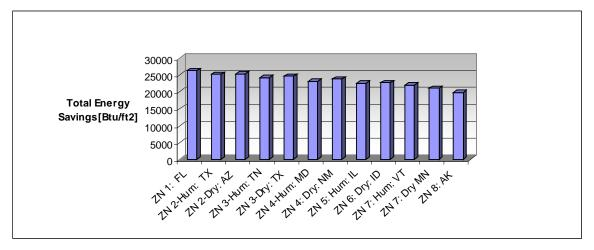
Figure 6.90. Estimated net energy savings for a 10% reduction in electric equipment use.
