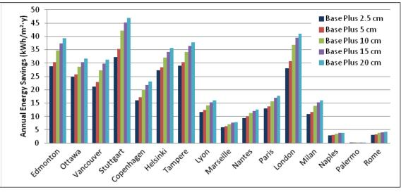
Figure 4.8. Energy savings for wall insulation and reduced infiltration over the Standard 90.1-1989 baseline - international locations.
