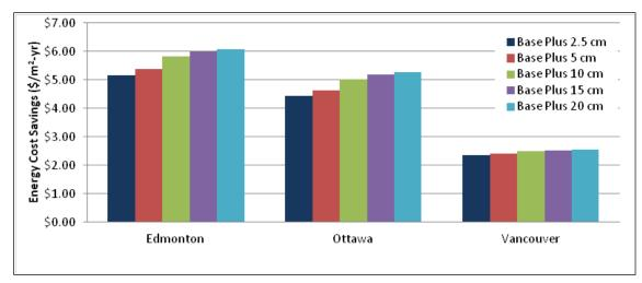
Figure 4.203. Energy cost savings for wall insulation and reduced infiltration over the noinsulation baseline – Canadian locations.
