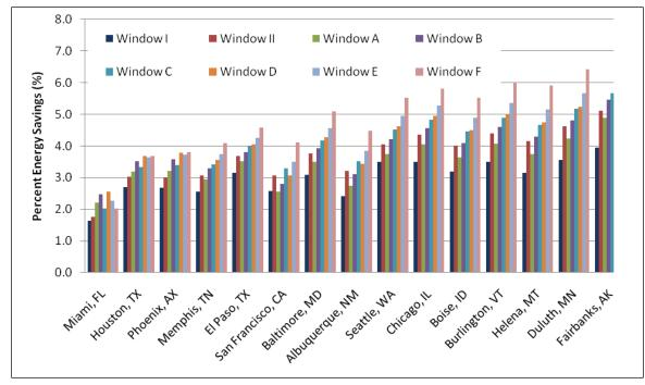
Figure 6.137. Percent of energy savings for modeled barracks facility in 15 US locations.
