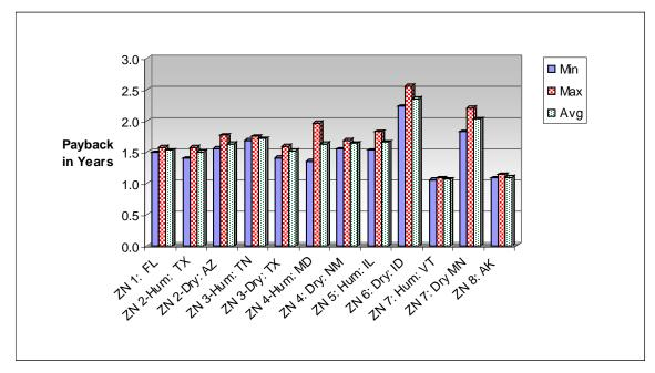
Figure 6.87. Estimated payback for 2% electric equipment use.
