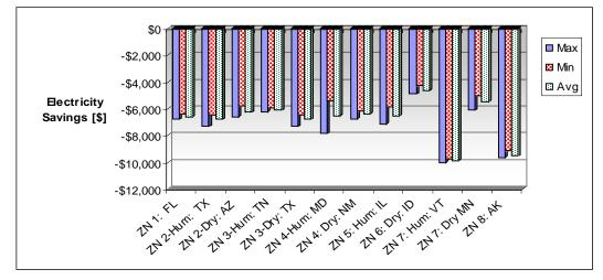
Figure 6.37. Increase in annual electrical fan power for ventilation only building.
