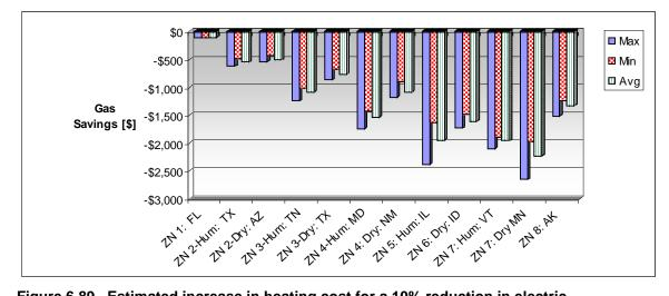
Figure 6.89. Estimated increase in heating cost for a 10% reduction in electric equipment use.
