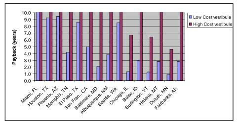
Figure 6.158. Estimated payback for high and low cost office vestibules in the United States.
