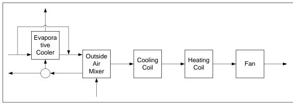
Figure 4.152. Schematic of the indirect evaporative cooling model (credit: Kyle Benne).
