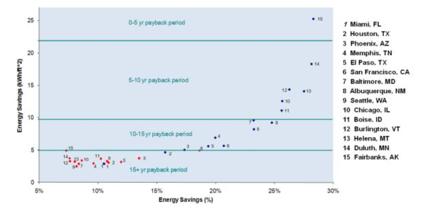
Figure 6.131. Comparison of SPB periods for Baselines 1 (Red) and 2 (Blue) with 4-in. thickness (US locations).
