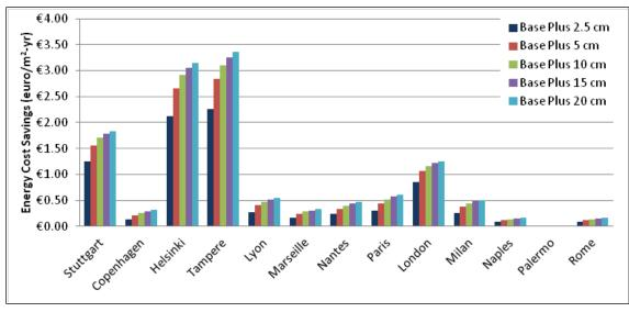
Figure 4.21. Energy cost savings for increased roof insulation and reduced infiltration over the Standard 90.1-1989 baseline – European locations.
