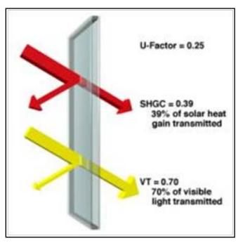
Figure 6.136. Critical window performance parameters.
