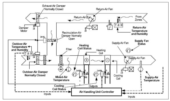
Figure 7.153. Air handler showing the sensor locations.
