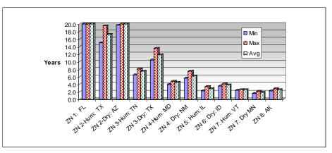
Figure 6.42. Radiant barrier estimated payback for high, low and medium energy rates.
