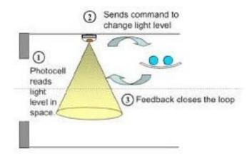
photo courtesy of automatedbuildings.com Figure 6.182. Closed loop control system.
