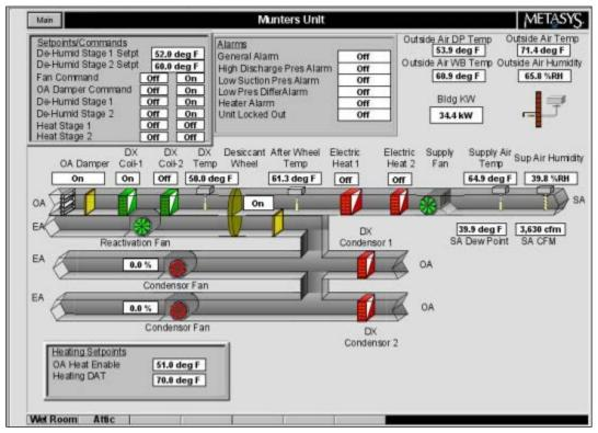
Figure 7.70. Screen capture of Bldg. 637 DX/desiccant DOAS unit schematic.
