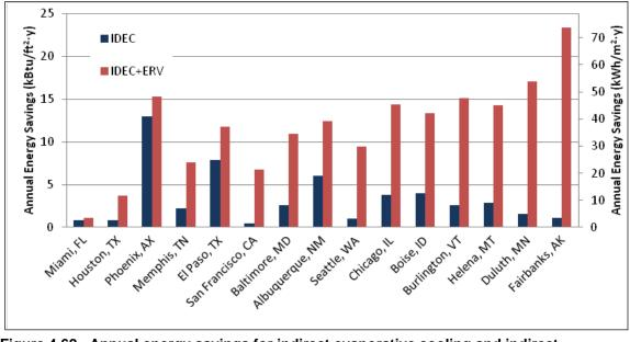
Figure 4.62. Annual energy savings for indirect evaporative cooling and indirect evaporative cooling with energy recovery.
