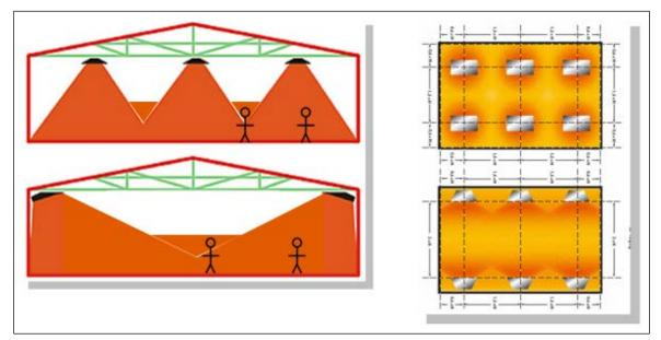
Figure 7.20. Interior versus perimeter placement.
