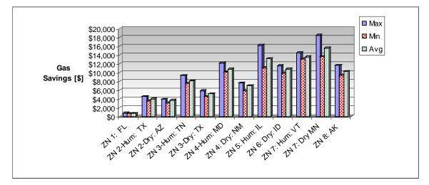
Figure 6.65. Estimated annual gas savings for high temperature radiant system.
