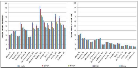
Figure 6.175. SPB period for baselines 1 (left) and 2 (right) with drainage system installation.
