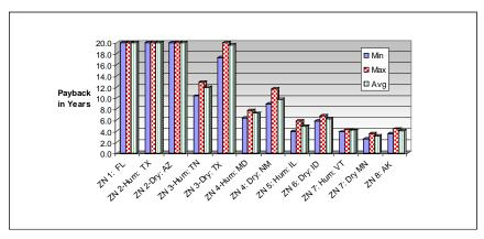
Figure 6.30. Estimated payback from installation of dock seals.
