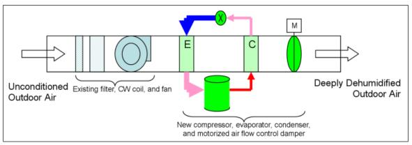
Figure 7.62. DOAS system schematic.
