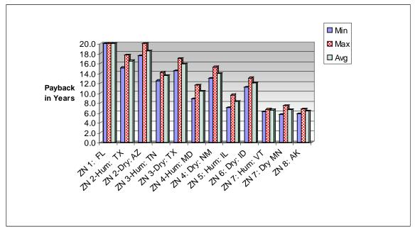
Figure 6.99. Estimated payback for 5% reduction in air flow rate.
