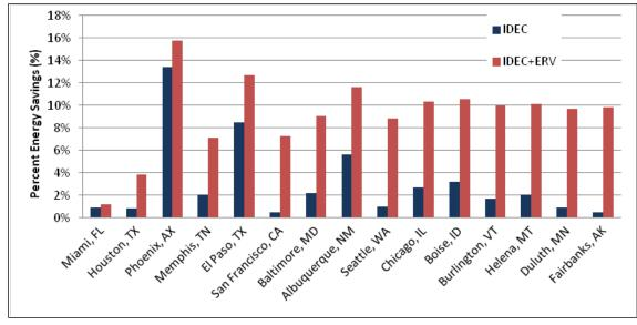
Figure 4.61. Percent energy savings for indirect evaporative cooling and indirect evaporative cooling with energy recovery.
