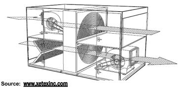
Figure 6.35. ERV with supply exhaust fans.
