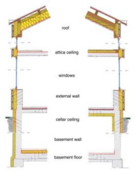
Figure 6.123. Example of building insulation in Berlin. Two different applications of insulation material (marked in yellow) in the roof are: (left) all insulation in the roof (heated attic); (right) one insulation layer above the attic ceiling, another insulation layer in the below the rafters (attic as a buffer zone). The basement insulation on left includes radiant floor heating whereas on the right the insulation layer is under the basement ceiling (unheated basement).
