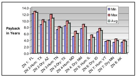
Figure 6.51. Estimated simple payback for boom system.
