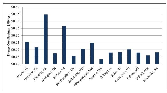
Figure 4.272. Annual energy cost savings for hybrid evaporative cooling.
