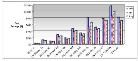
Figure 6.45. Estimated annual radiant barrier gas savings.
