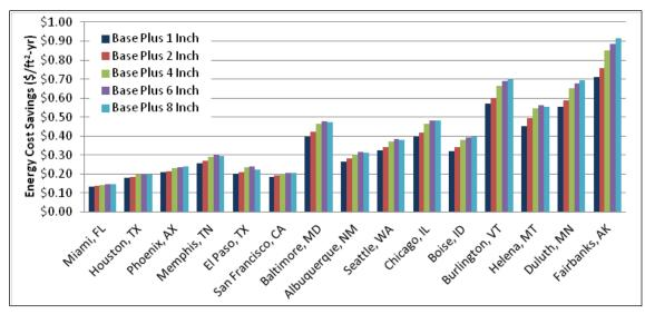
Figure 4.86. Energy cost savings for wall insulation and reduced infiltration over the noinsulation baseline.
