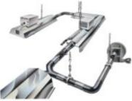
Figure 6.62. Radiant gas fired heating system.
