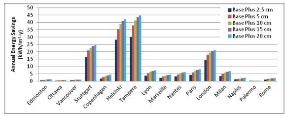
Figure 4.19. Energy savings for increased roof insulation and reduced infiltration over the Standard 90.1-1989 baseline – international locations.
