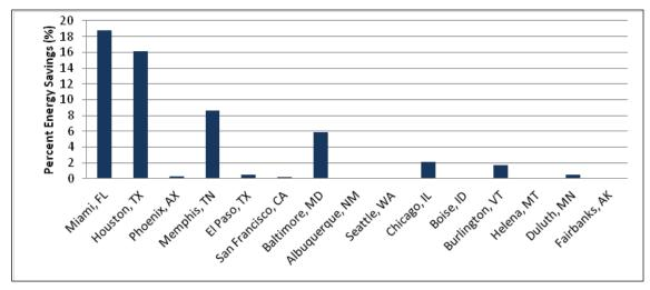
Figure 4.78. Percent energy savings for reheat using condenser waste heat.
