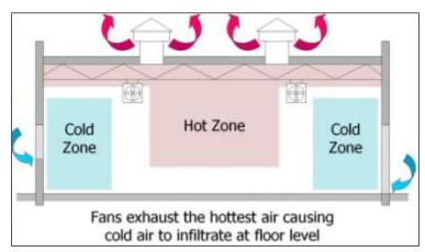
Figure 7.137. Destratification improves comfort while reducing heat losses.
