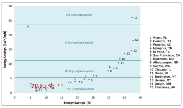
Figure 6.176. Comparison of SPB periods for baselines 1 (Red) and 2 (Blue) with 4-in (~102-mm). thickness, US Locations.
