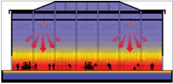
Figure 7.19. How radiant heats at ground level.
