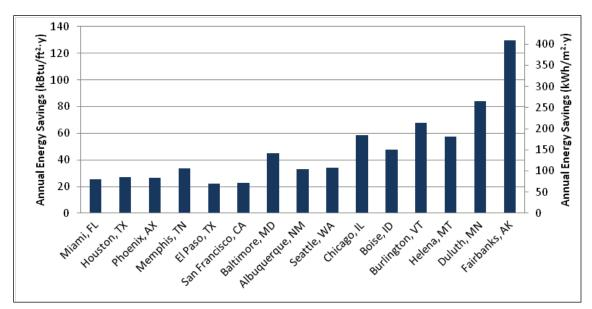
Figure 4.70. Annual energy savings for DOAS with radiant heating and cooling.
