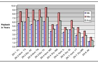
Figure 6.108. Estimated payback based on a 10 workstation system.
