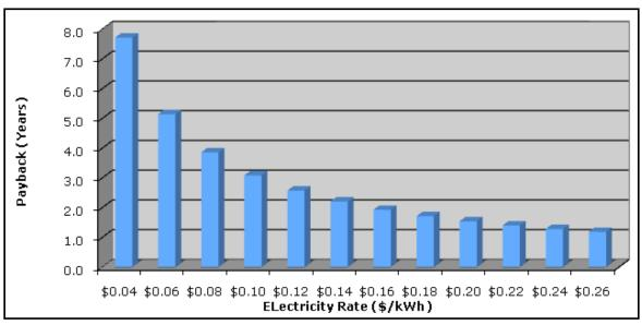
Figure 6.84. Spectrally enhanced lighting simple payback.
