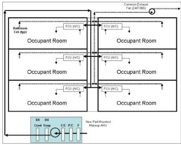
Figure 7.63. New DOAS system configuration (elevation view).
