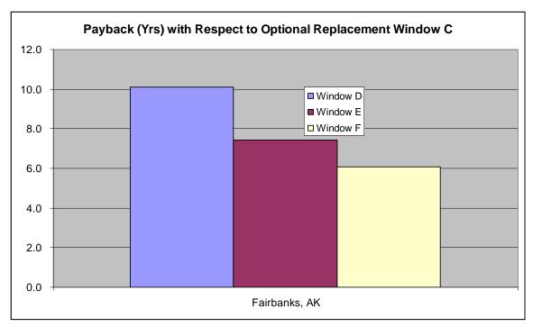
Figure 6.142. Modeled payback results of upgrading to premium quality replacement windows from current baseline quality replacement windows (Zone 8) for a *major renovation or repair project.*
