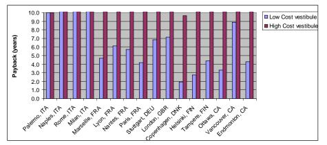
Figure 6.163. Estimated payback for high and low cost dormitory vestibules in Europe and Canada.
