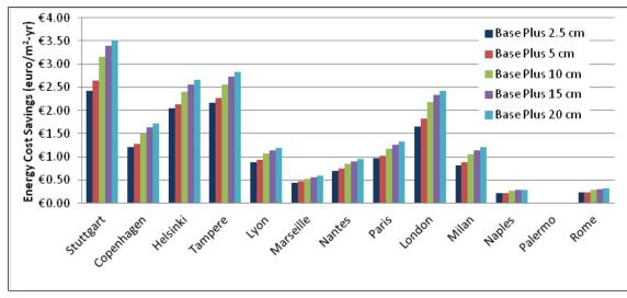
Figure 4.10. Energy cost savings for wall insulation and reduced infiltration over the Standard 90.1-1989 baseline - European locations.
