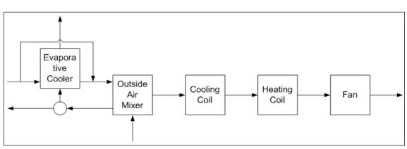
Figure 4.60. Schematic of the indirect evaporative cooling model (credit: Kyle Benne).
