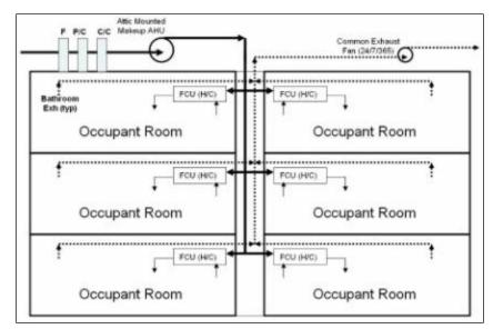
Figure 7.61. Original system configuration (elevation view).
