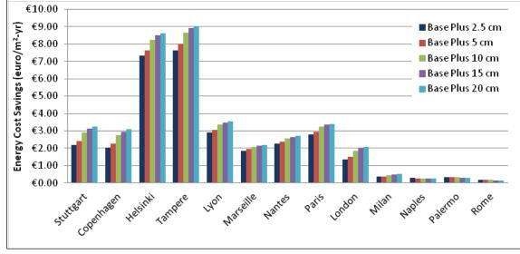
Figure 4.94. Energy cost savings for wall insulation and reduced infiltration over the noinsulation baseline – European locations.
