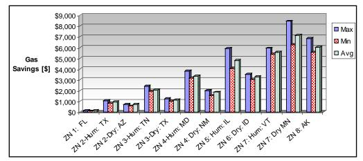
Figure 6.25. Estimated annual gas savings for system achieving 25% reduction of ventilation flow rate.
