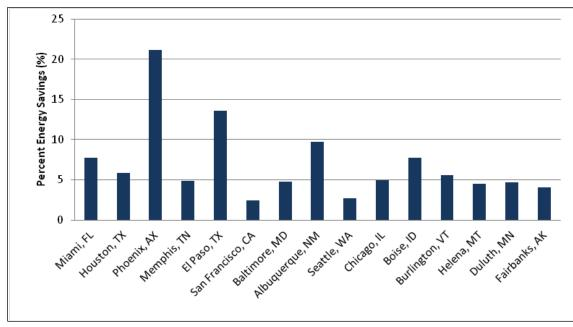
Figure 4.64. Percent energy savings for hybrid evaporative cooling.
