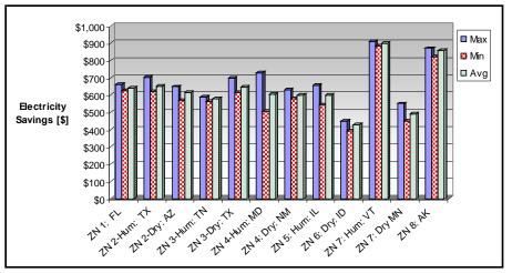
Figure 6.52. Estimated annual electricity savings for rail or boom system.
