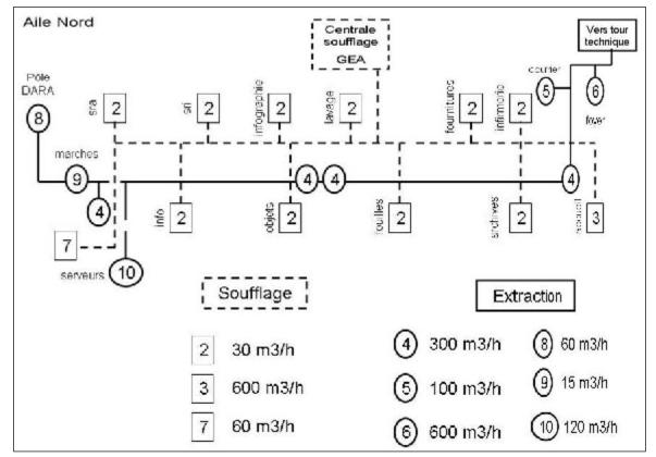
Figure 7.85. Ventilation system configuration (first floor north).
