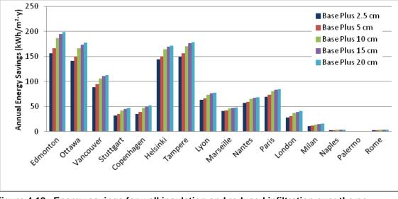
Figure 4.12. Energy savings for wall insulation and reduced infiltration over the noinsulation baseline- international locations.
