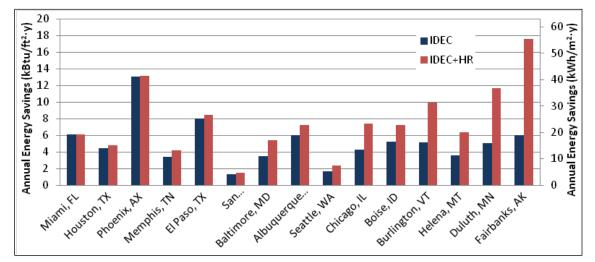
Figure 4.264. Annual energy savings for indirect evaporative cooling and indirect evaporative cooling with heat recovery.
