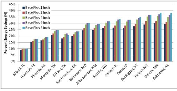
Figure 4.194. Percent energy savings for wall insulation and reduced infiltration over the no-insulation baseline.
