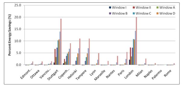
Figure 6.138. Percent of energy savings for modeled barracks-type facility in Canadian and European locations.
