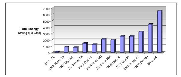
Figure 6.58. Estimated total energy savings for high speed roller doors.
