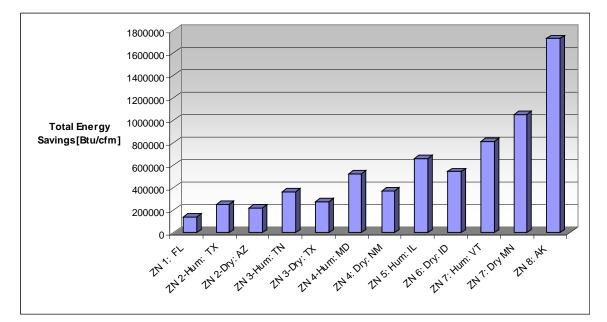
Figure 6.98. Estimated annual energy savings per cfm reduction in air flow rate.
