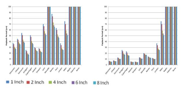
Figure 6.132. SPB period in years for EIFS with drainage system – international sites.
