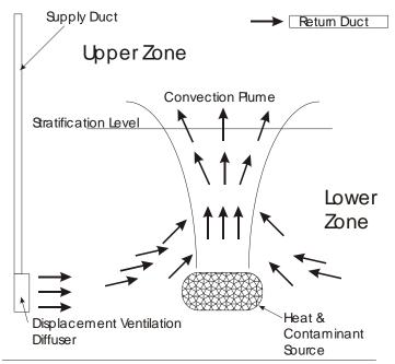
Figure 6.19. Displacement ventilation concept.
