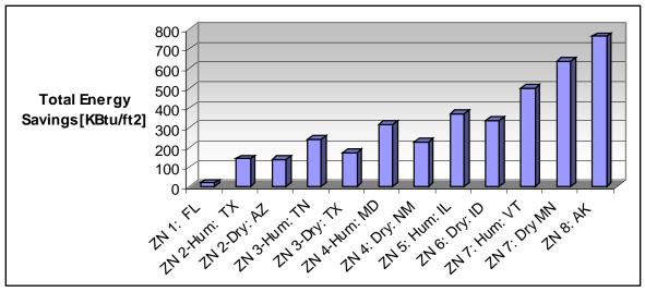
Figure 6.82. Transpired solar wall total annual energy savings per square foot of collector area.
