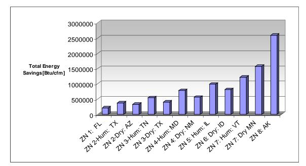
Figure 6.71. Annual energy savings (Btus) per cfm reduction in the outside air flow rate.
