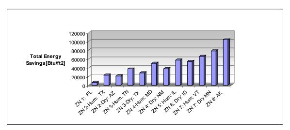
Figure 6.66. Estimated total annual energy savings per square foot for radiant system.
