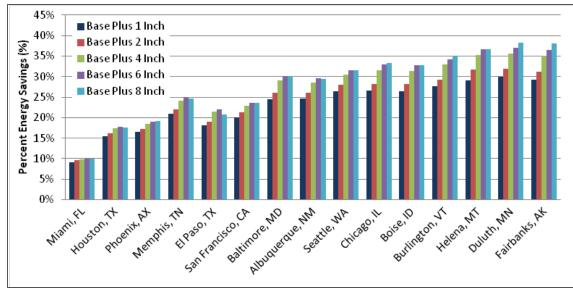
Figure 4.84. Percent energy savings for wall insulation and reduced infiltration over the no-insulation baseline.
