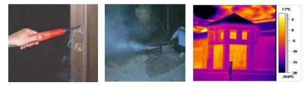
Figure 6.118. Smoke pencil (left) and theatrical fog (center) for leakage pathways; infrared thermography (right) for heat.
