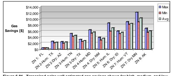
Figure 6.81. Transpired solar wall estimated gas savings shown for high, medium, and low energy rates.
