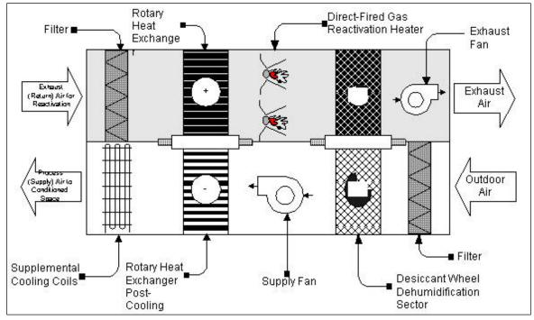
Figure 7.161. Schematic of the two-wheel desiccant system.
