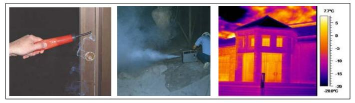
Figure 6.165. Smoke pencil (left) and theatrical fog (center) for leakage pathways; infrared thermography (right) for heat.
