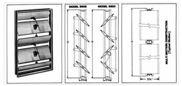
Figure 6.67. HVAC control dampers.
