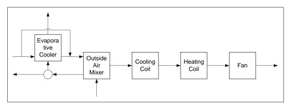
Figure 4.262. Schematic of the indirect evaporative cooling model (credit: Kyle Benne).
