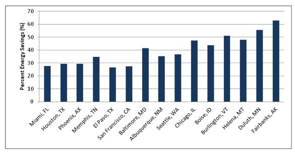
Figure 4.69. Percent energy savings for DOAS with radiant heating and cooling.
