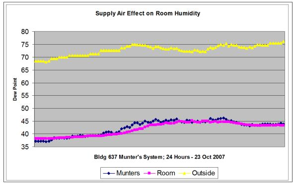
Figure 7.74. Modules A and B; effect of dry outdoor air on occupant room DPTs.
