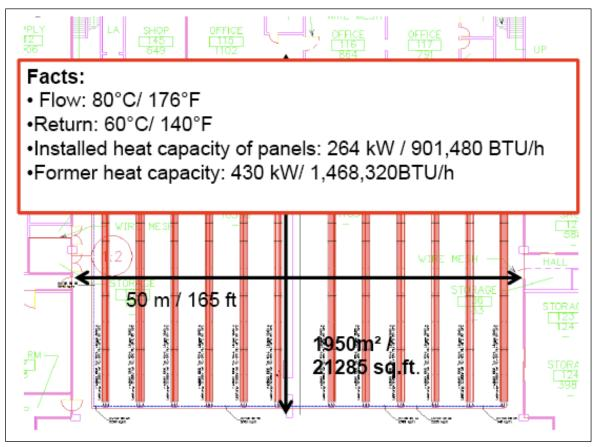
Figure 7.106. Schematic of Hangar 5807-1/2.
