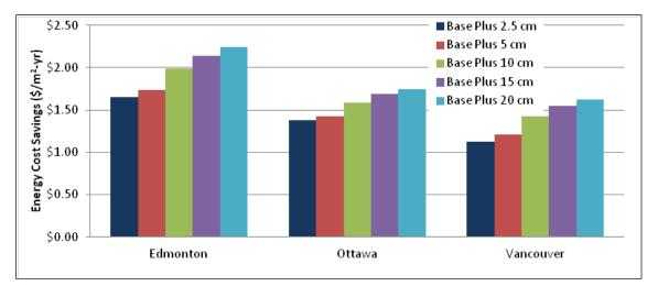
Figure 4.9. Energy cost savings for wall insulation and reduced infiltration over the Standard 90.1-1989 baseline - Canadian locations.
