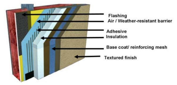
Figure 6.124. EIFS construction with drainage.
