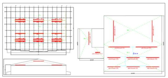
Figure 7.99. Layout of heater placement in Hangar 2310 and warehouse in Kaiserslautern.
