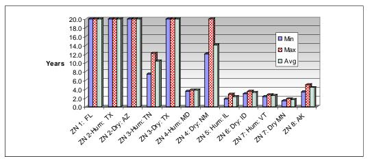
Figure 6.36. Estimated payback for installation of rotary heat exchanger.
