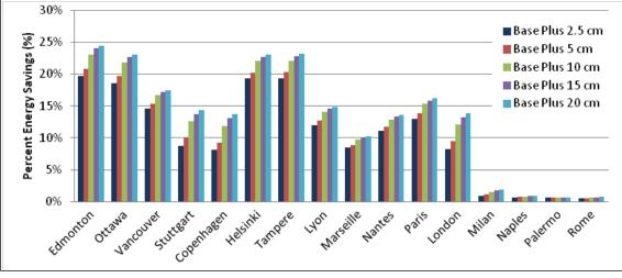
Figure 4.201. Percent energy savings for wall insulation and reduced infiltration over the no-insulation baseline – International locations.
