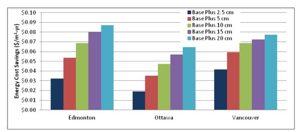
Figure 4.20. Energy cost savings for increased roof insulation and reduced infiltration over the Standard 90.1-1989 baseline – Canadian locations.
