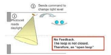
photo courtesy of automatedbuildings.com Figure 6.181. Open loop control system.
