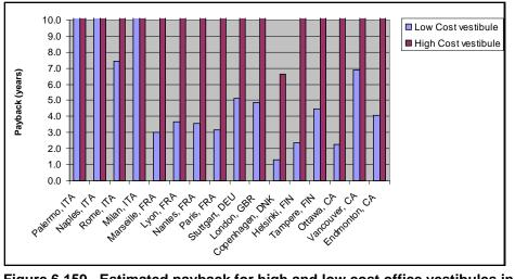
Figure 6.159. Estimated payback for high and low cost office vestibules in Europe and Canada.
