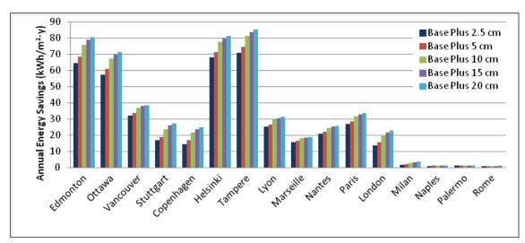
Figure 4.202. Energy savings for wall insulation and reduced infiltration over the noinsulation baseline – international locations.
