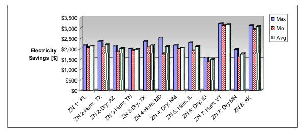
Figure 6.64. Estimated annual electric savings for high temperature radiant system.
