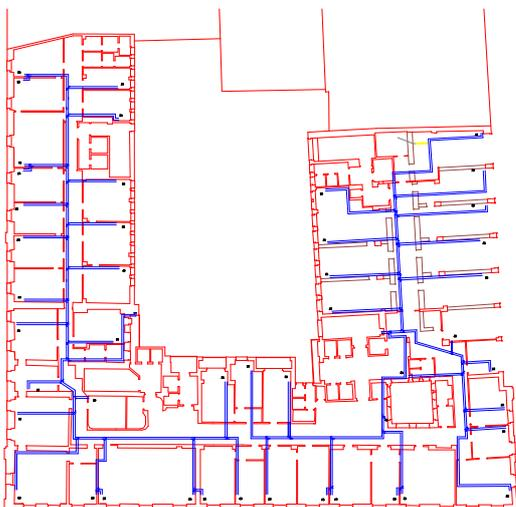
Lay-out of the refrigerant fluid tubes connecting the internal units.
