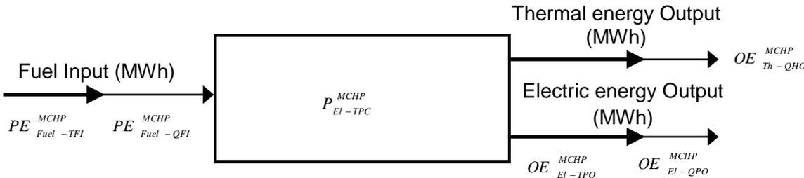
**Fig. 33: Energy flows for the application of CHPQA methodology**
