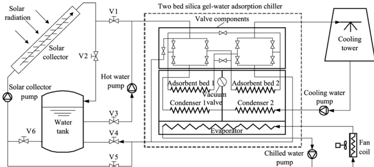
Fig. 24: Schematic diagram of a solar-powered adsorption cooling system
