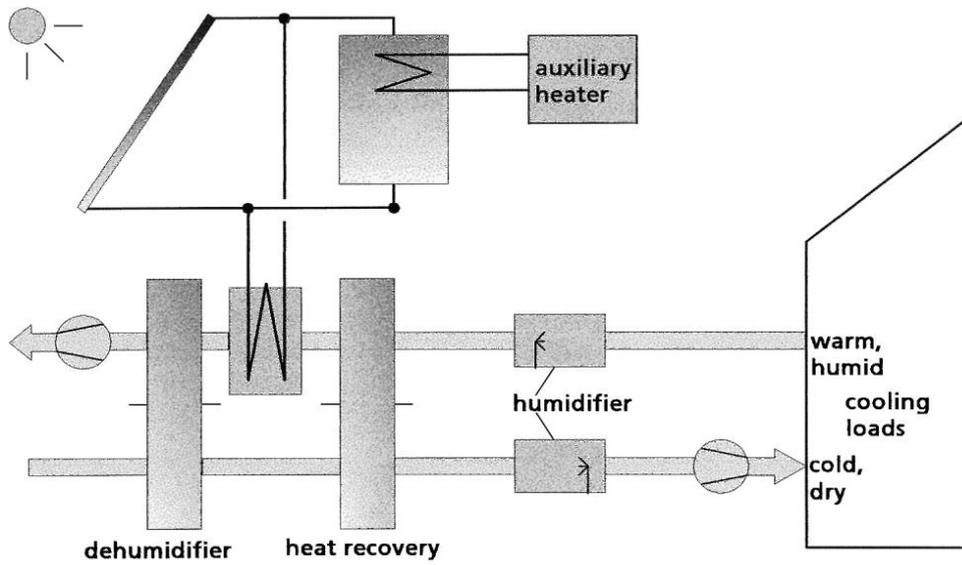
Fig. 28: Schematic representation of a solar desiccant cooling cycle.
