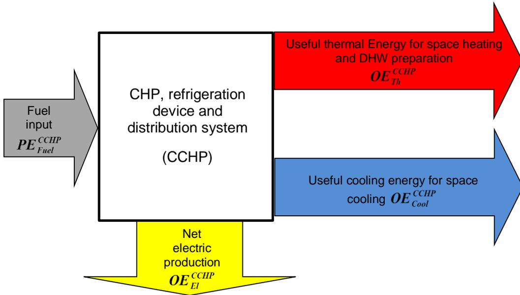
Fig. 31: Energy flows for the application of technical form n. 21T of the AEEG
