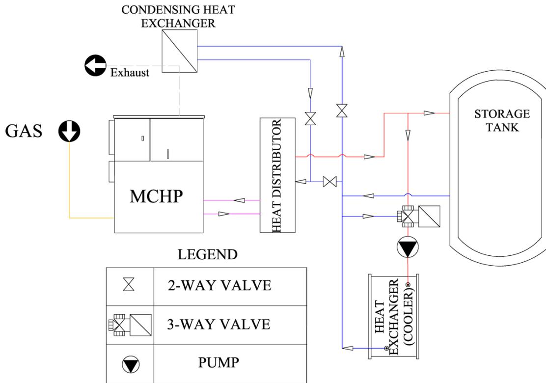
**Fig. 13: The hydraulic setup for the tests according to DIN 4709**
