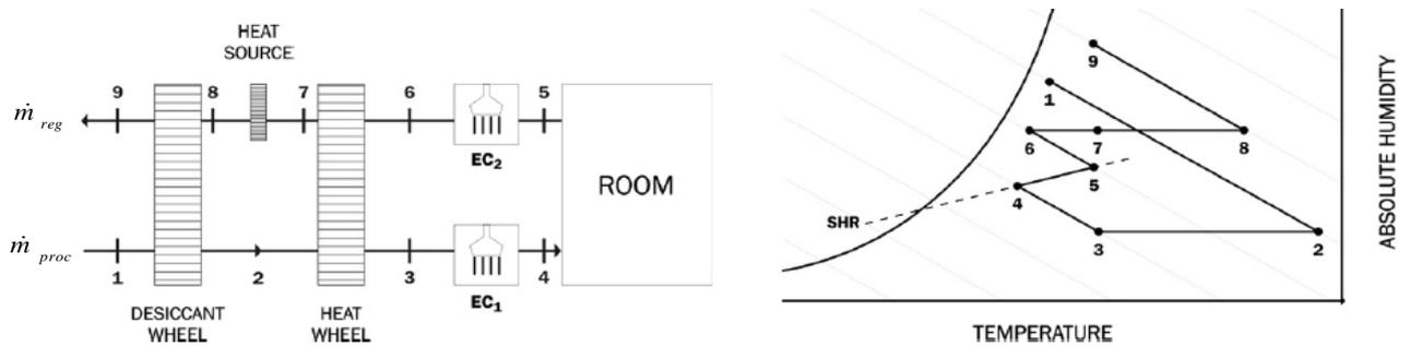
Fig. 25: Schematic representation of a desiccant cooling cycle.
