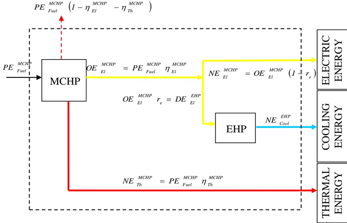
Fig. 20: Energy flows of the MCHP/EHP system in summer operation.
