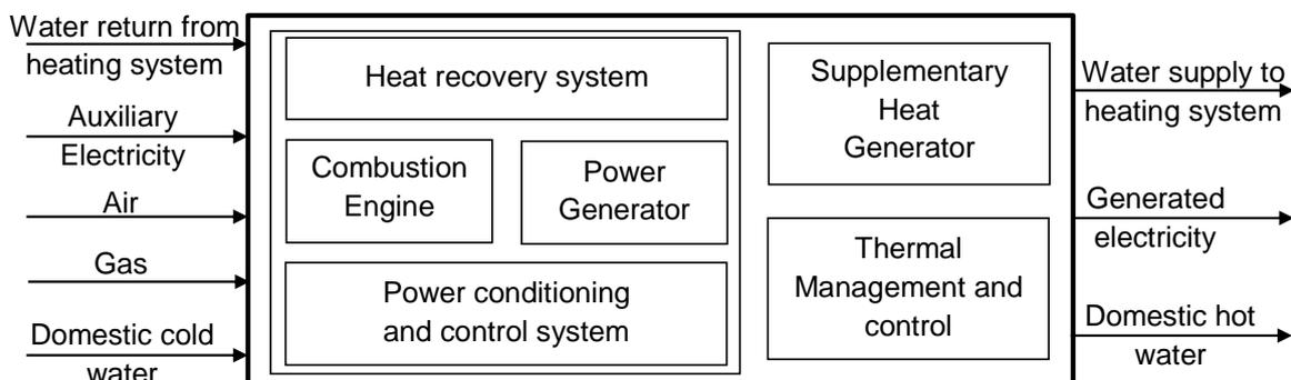
Fig. 9: Typical set-up for an internal combustion engine MCHP appliance
