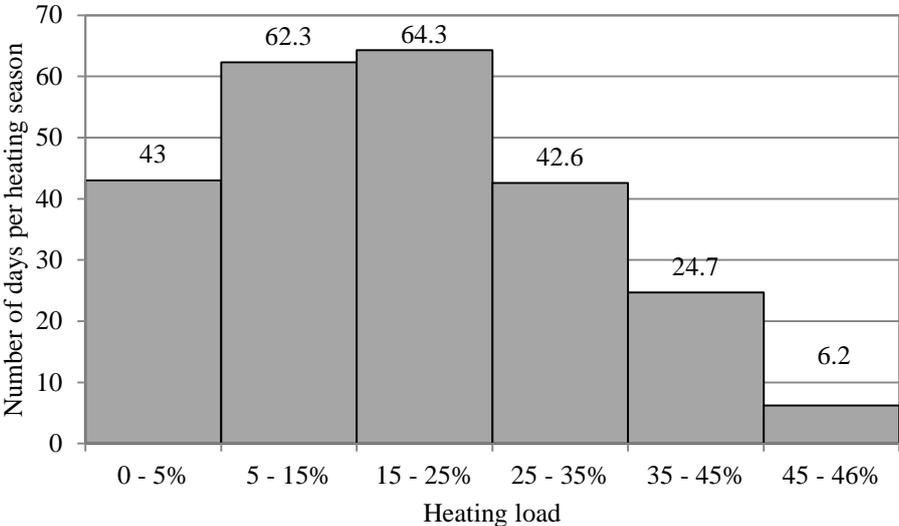
Fig. 34: Load profile for the space heating and hot water for regime three (PSR = 1.5) [58]
