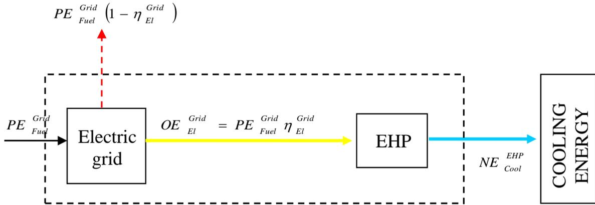
Fig. 21: Energy flows of the EHP system powered from the electric grid during summer operation.
