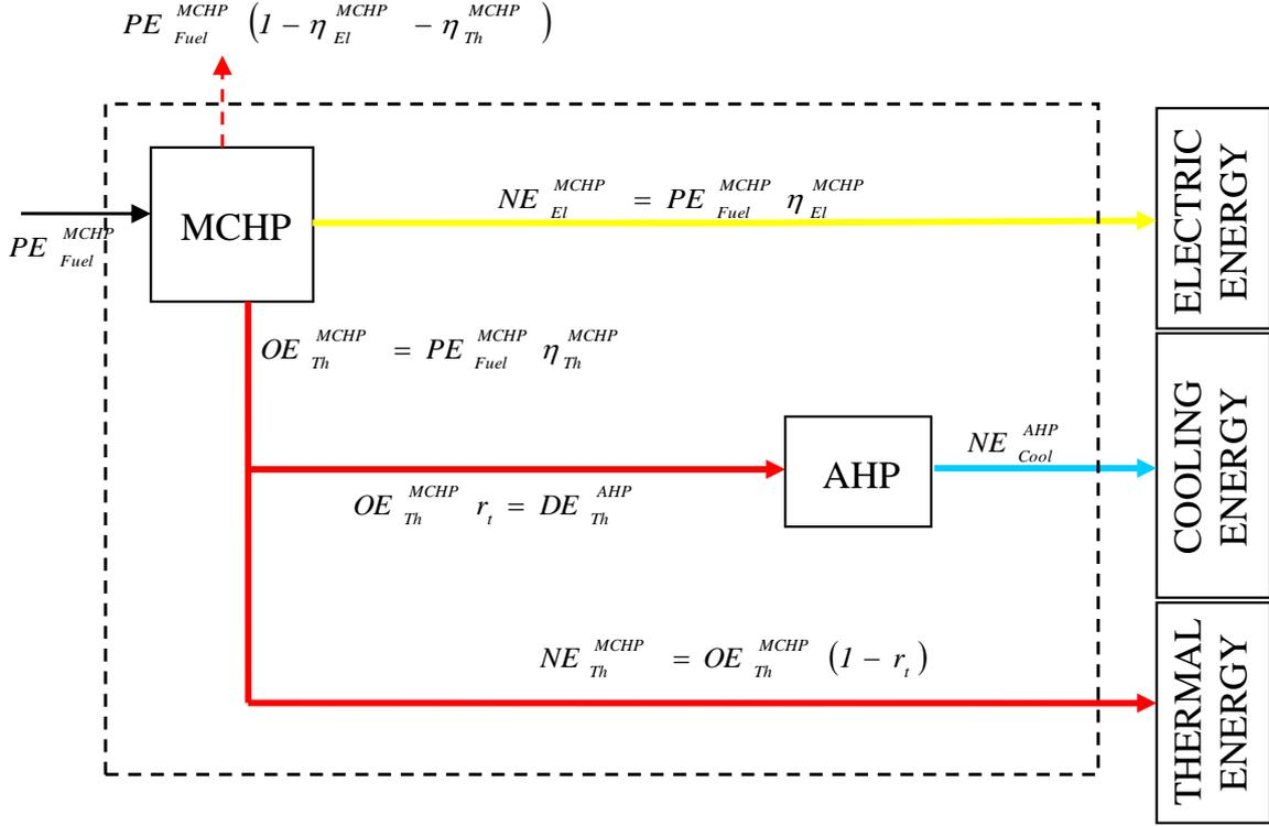
Fig. 22: Energy flows of an MCHP/AHP system during summer operation.
