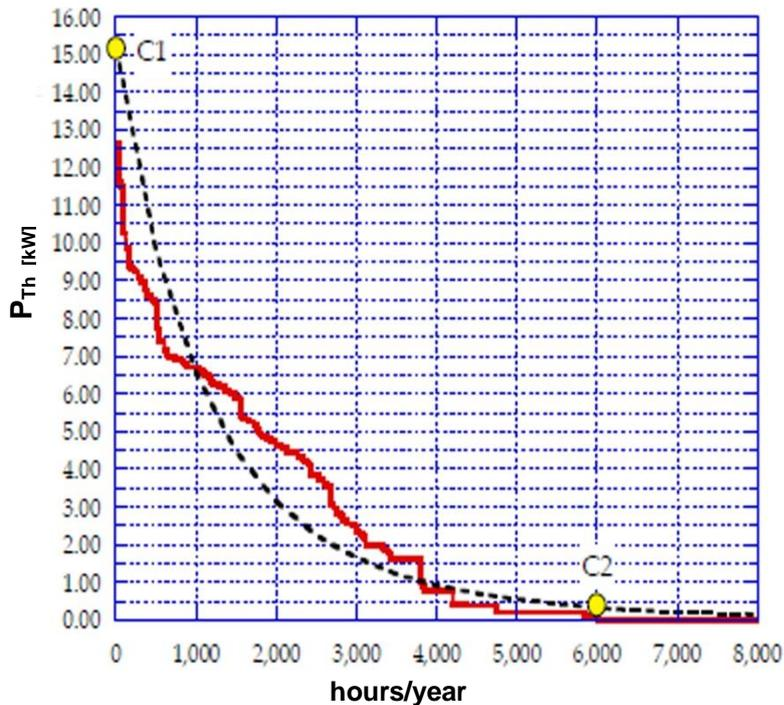
Fig. 4: Actual and modelled monotonic thermal demand curves for a residential user.
