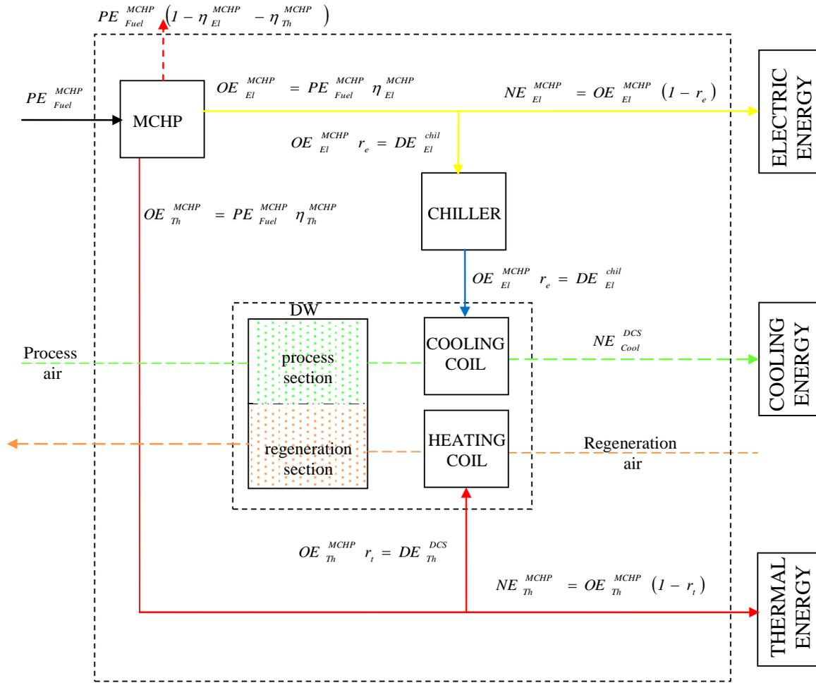
Fig. 27: Energy flows of an MCHP/HVAC-DW system.
