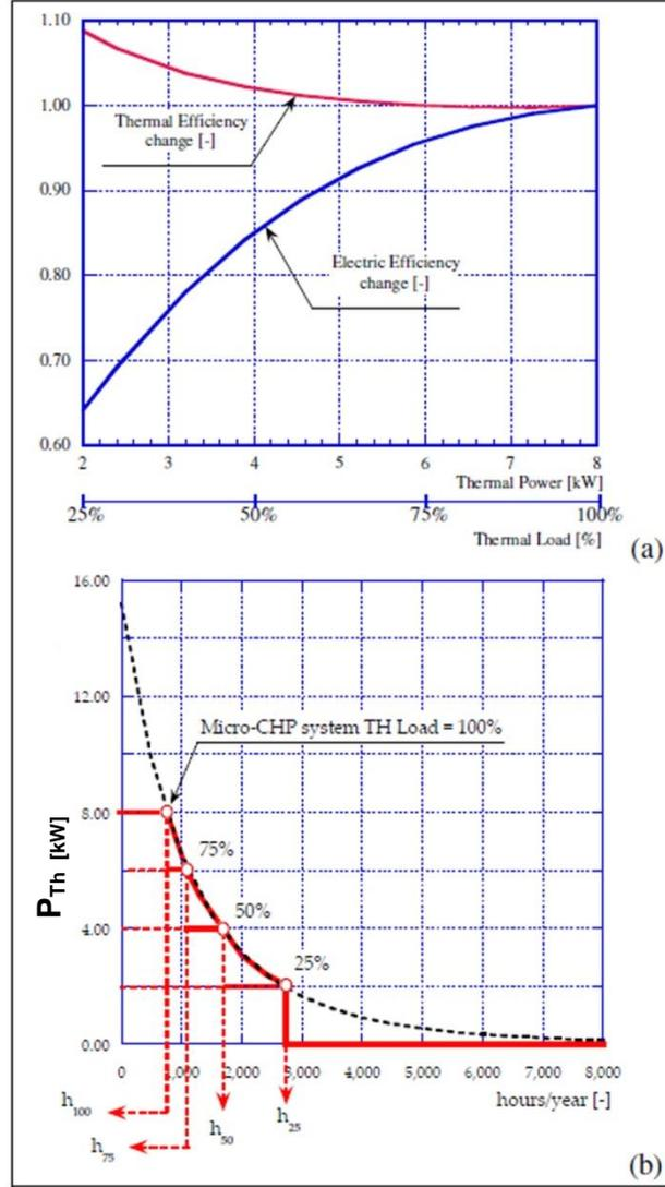
Fig. 5: MCHP part-load performance curves (a) and significant operating points (b)
