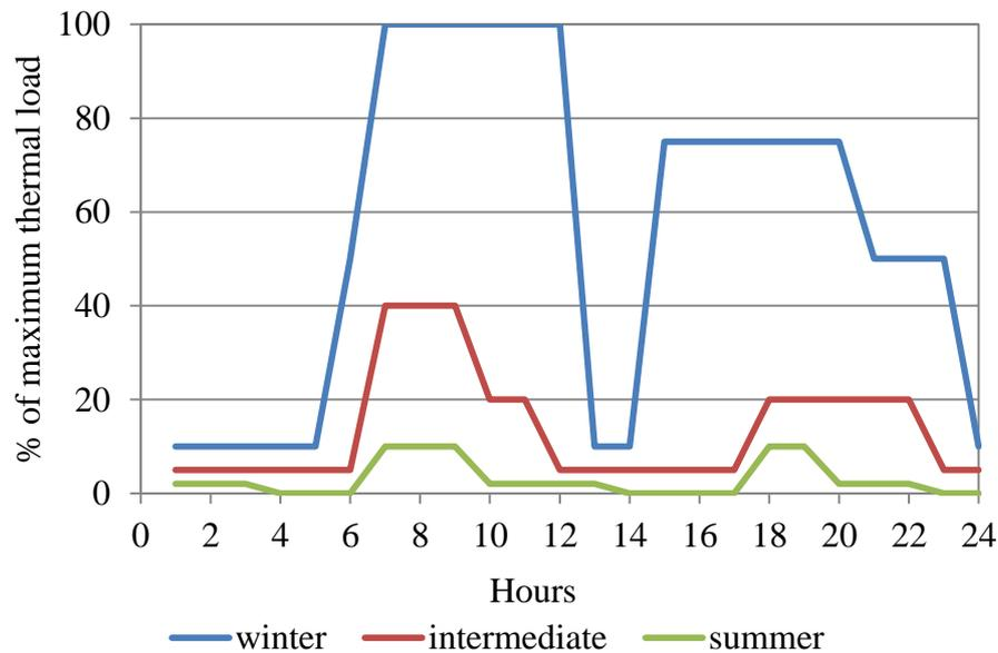
Fig. 2: Thermal-load profile for the three day types
