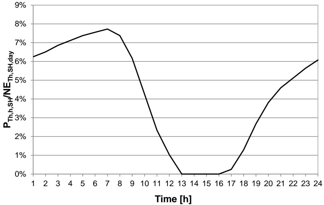
Fig. 7: Thermal-load profile for space heating requirements (Milan – October)
