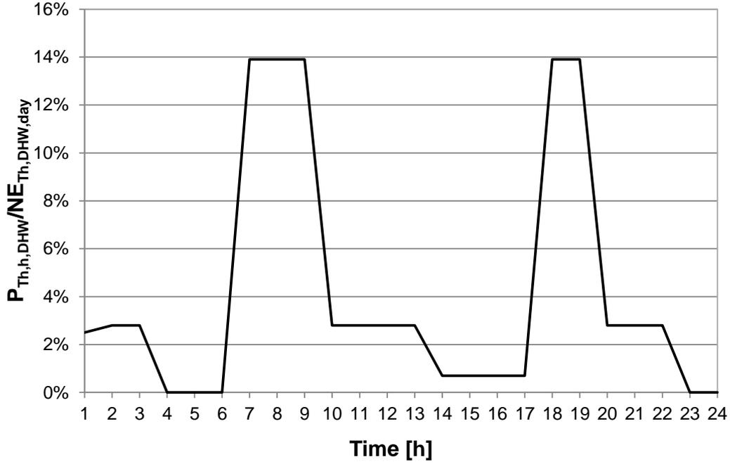
Fig. 6: Domestic hot water load profile as defined by UNI/TS 11300-4
