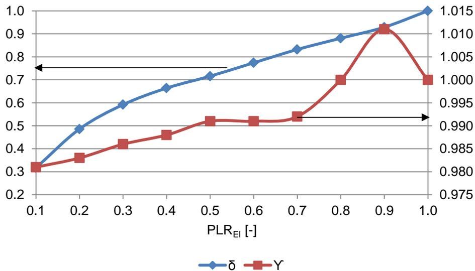
Fig. 8: Normalized performance curves for internal combustion engine-based CHPs
