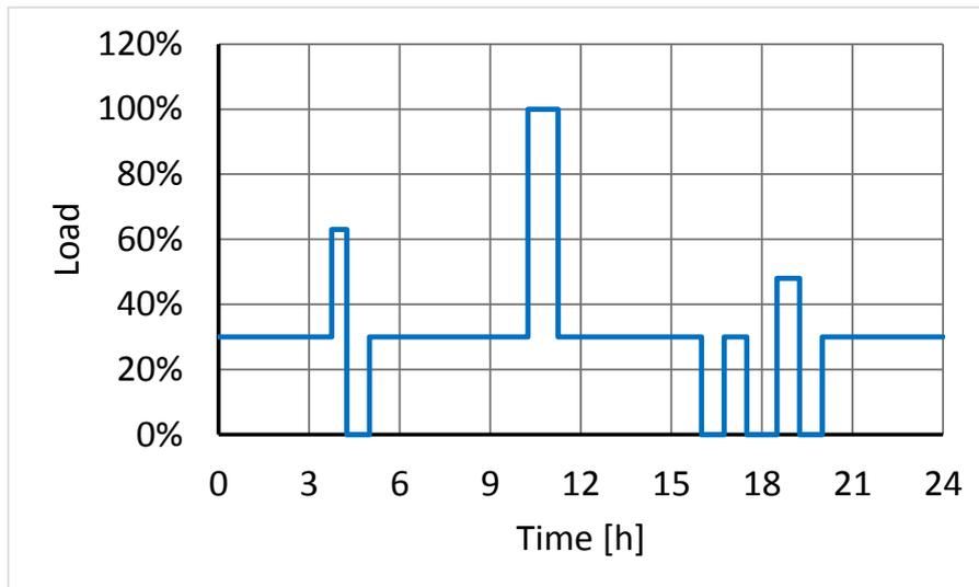
Fig. 11: DIN 4709 Thermal-Load Profile – X is the time [h] and Y is the ratio between thermal output and rated output [%]
