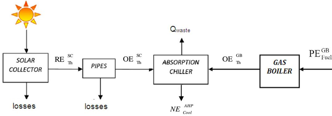
Fig. 23: Diagram illustrating the energy flows of a solar/gas absorption cooling plant.
