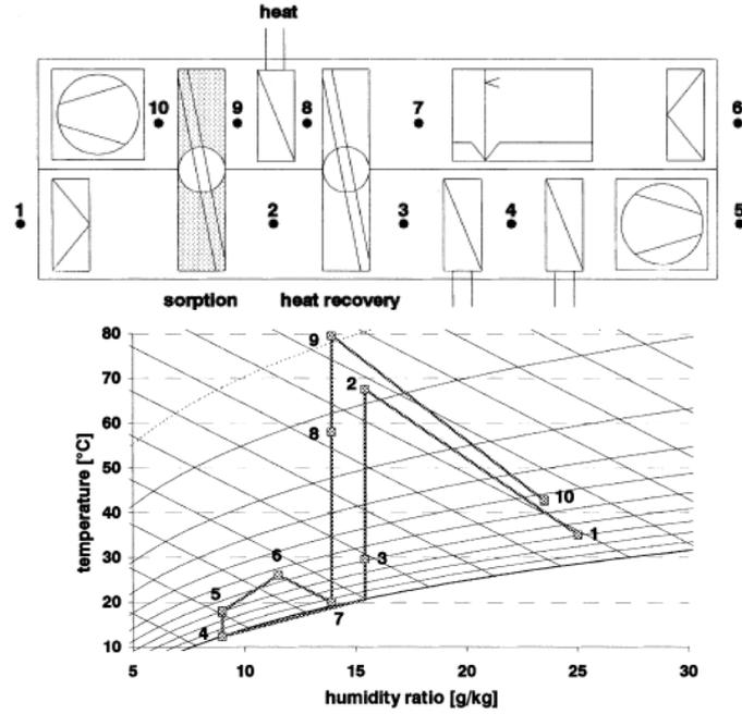
Fig. 26: Standard cycle with an additional cooling-coil behind a heat recovery wheel
