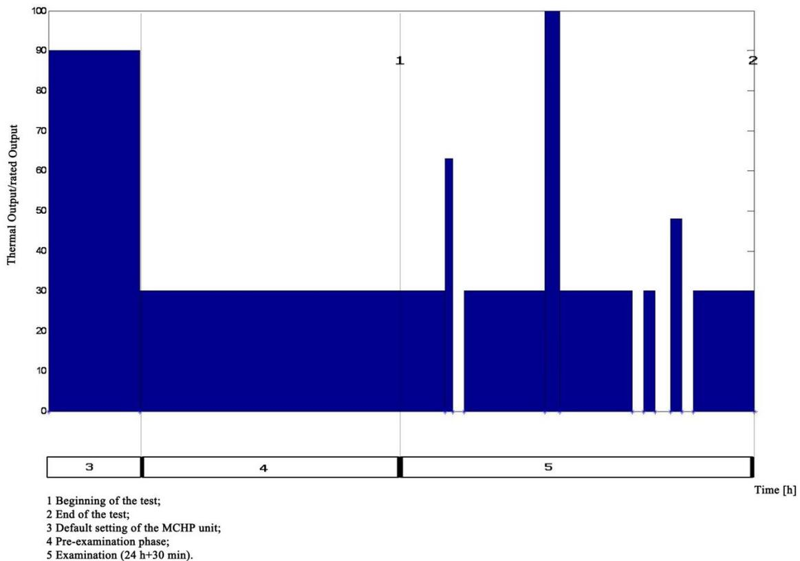
**Fig. 12: Schematic representation of the test process**
