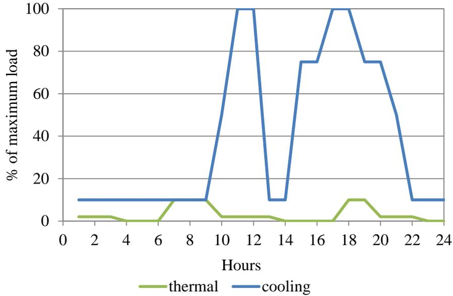
Fig. 3: Summer thermal and cooling load profiles for tri-generation systems
