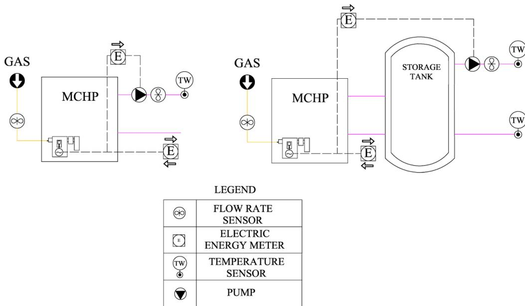
**Fig. 10: Schematic representations of two equipment options with measuring points: left – MCHP without thermal storage; right - MCHP with thermal storage**
