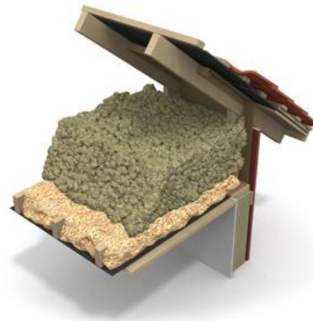
Figure 6.11: Ventilating cold attic with added insulation.
