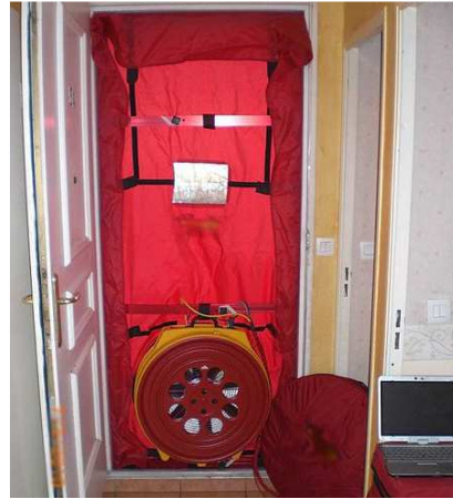
Figure 3.38 Installed ventilator of blower door test (source: Wikipedia).
