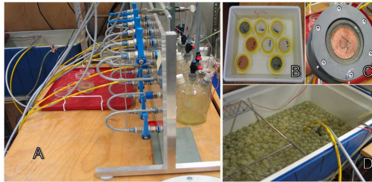
Figure 2.21 Head permeameter apparatus (A); laterally sealed specimens (B); head permeameter with specimen (C); water container (D).
