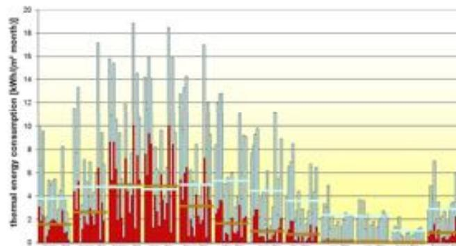
Figure 25: Measured thermal energy consumption for heating and domestic hot water preparation
