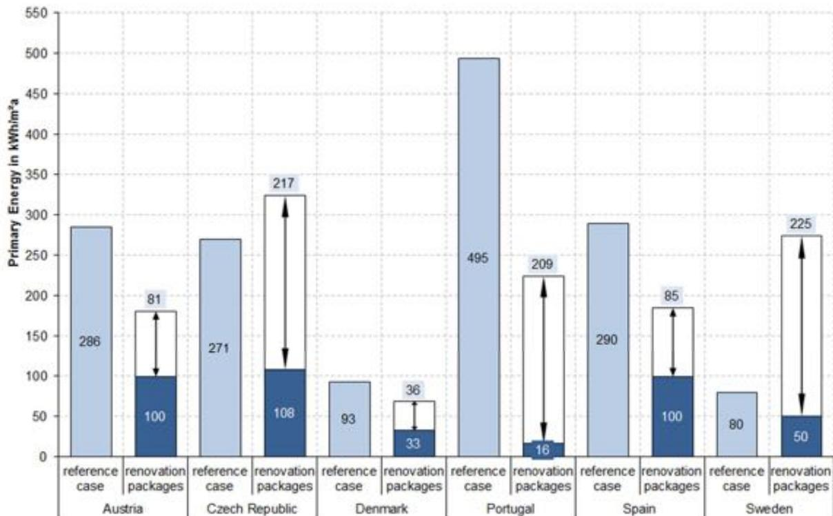
Figure 39: Total Primary Energy of the six Case Studies. The total Primary Energy values of the reference cases are compared to the total Primary Energy values of the investigated renovation packages, shown as lowest value and as range between the lowest and the highest value.
