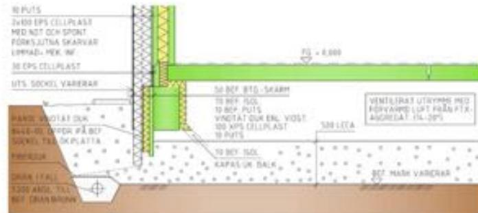
Figure 8: Cross section of exterior wall and floor-foundation construction
