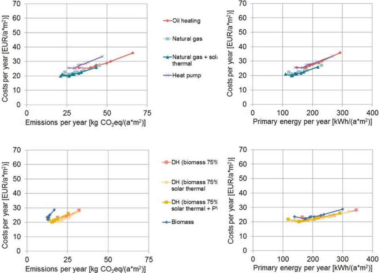
Figure 25: Aggregated comparison of cost effectiveness of energy efficiency renovation measures for different heating systems and related impacts on carbon emissions and primary energy use for the Spanish Case Study
