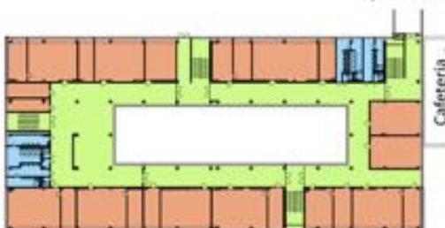
Figure 2: Ground plan of the main block's second floor. Red – classrooms and offices; blue – toilets; green – corridors and staircases.
