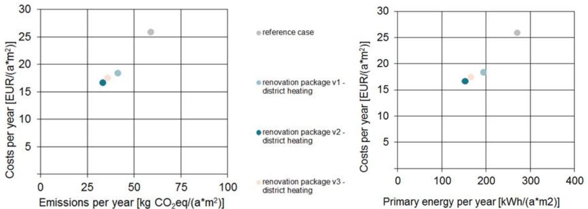
Figure 31: Comparison of four different renovation scenarios, all equipped with district heating, for the Czech Case Study, to investigate the influence of the thermal quality of the building envelope on the annual Life Cycle Costs, carbon emissions and Primary Energy
