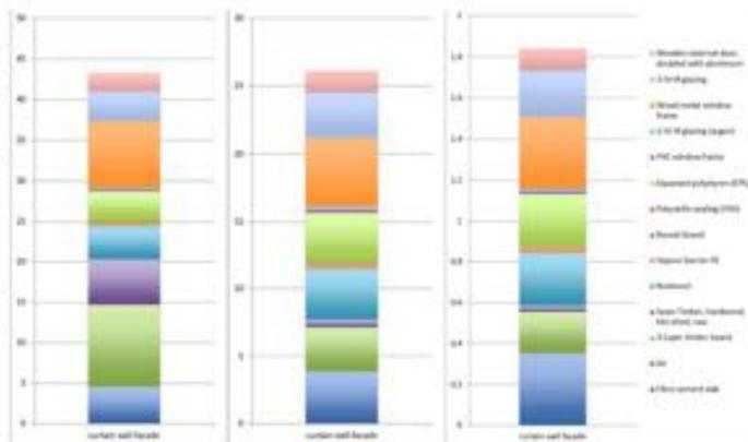
Figure 20: environmental impact of the different materials of the prefabricated façade module
