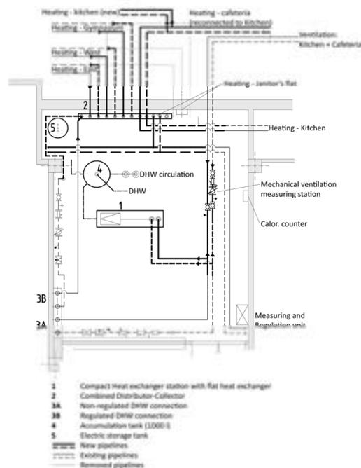
Figure 18: Schema of the boiler room before and after the renovation. [1]
