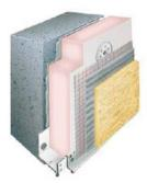
Figure A-4. Insulation composite system for Bldg. 42 with high resistant layers.
