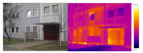
Figure A-3. Thermal photography of Bldg. No. 42.
