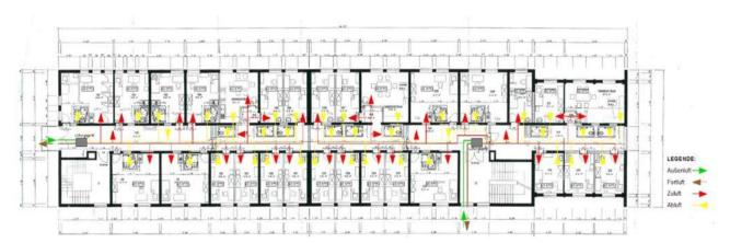
Figure A-2. Scheme of new mechanical ventilation system with fresh (green), inlet (red), outlet (brown) and exhaust air (yellow) applied in Bldg. 43.
