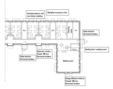
Figure C-4. Floor plan of Bldg. 3 with the energy retrofit measures.
