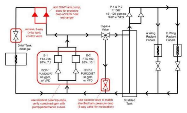
Figure D-10. System diagram of Bldg. 630's closed loop hydronic system (design errors shown in red).
