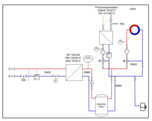
Figure A-7. Scheme of the secondary heating and domestic hot water circuit of Bldg. 3.
