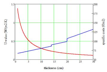
Figure B-3. U-value of external wall (red curve and left vertical scale) and insulation costs (right vertical scale) as function of thickness (heat transfer coefficient = 0.035 W/m<sup>2</sup>K).
