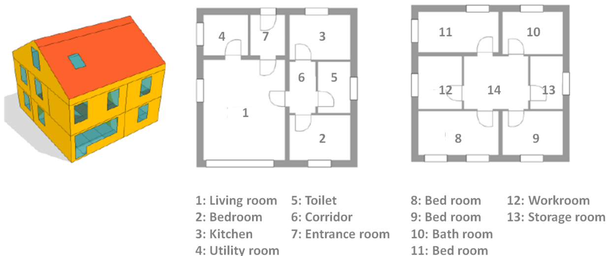
Figure 9.1 Perspective view and floor plan of the ground floor (left) and first floor (right) of the single family house.
