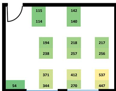
**Figure 4.37:** Illuminance values on task area (only Daylight)
