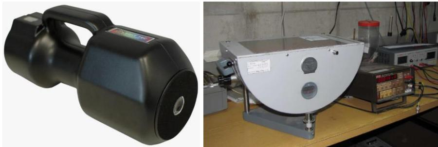
Figure 18: The Light Tec Mini-Diff V2 and a Carl Zeiss in-plane measurement goniometer for the characterization of base materials
