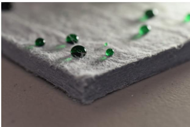
Hydrophobic aerogel fibre mat.
