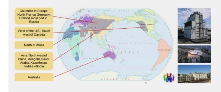
Climate regions potentially suitable for using indirect evaporative cooling technology. Source: Building Energy Research Center, Tsinghua University / Map source: m.onegreen.net
