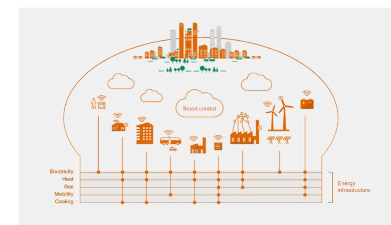
Local energy needs in a positive energy district are minimized by improving energy efficiency, using renewable energy production and smart control. Smart control and energy flexibility are needed to match demand with energy production and storage.
