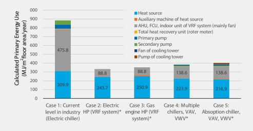
An example of HVAC energy calculations for four energy efficient cases (Cases 2 to 5) compared with the target energy use (criterion of building energy standard compliance for this example office building). Source: EBC Working Group on HVAC Energy Calculation Methodologies for Non-residential Buildings
