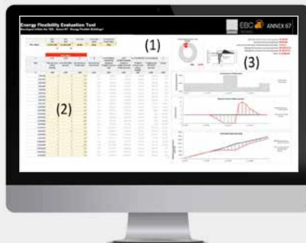
An overview of the interface for the Energy Flexibility Evaluation Tool (FET): (1) overall inputs for timespan, time steps, cost-function / penalty signal and units, (2) input data about a building's load profile, flexible load profile and a cost function based on the time steps, timespan and units, and (3) evaluation charts and characterization.
