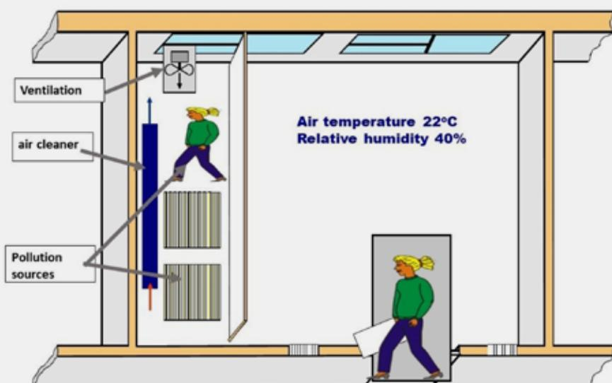
Test of a gas phase air cleaner using measurement of perceived air quality by judges entering the space. Pollution sources include emissions from building products and people.
