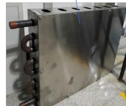
Composite phase change regenerative heat exchanger
