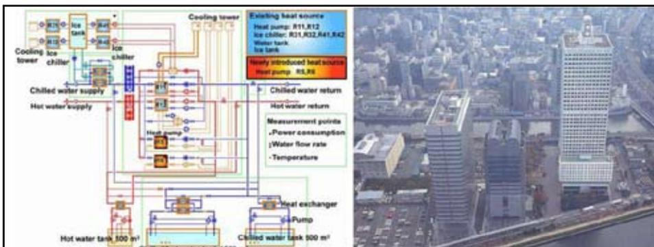
*A generic commissioning tool is under development for the energy plant which supplies chilled/hot water to three commercial buildings.*
