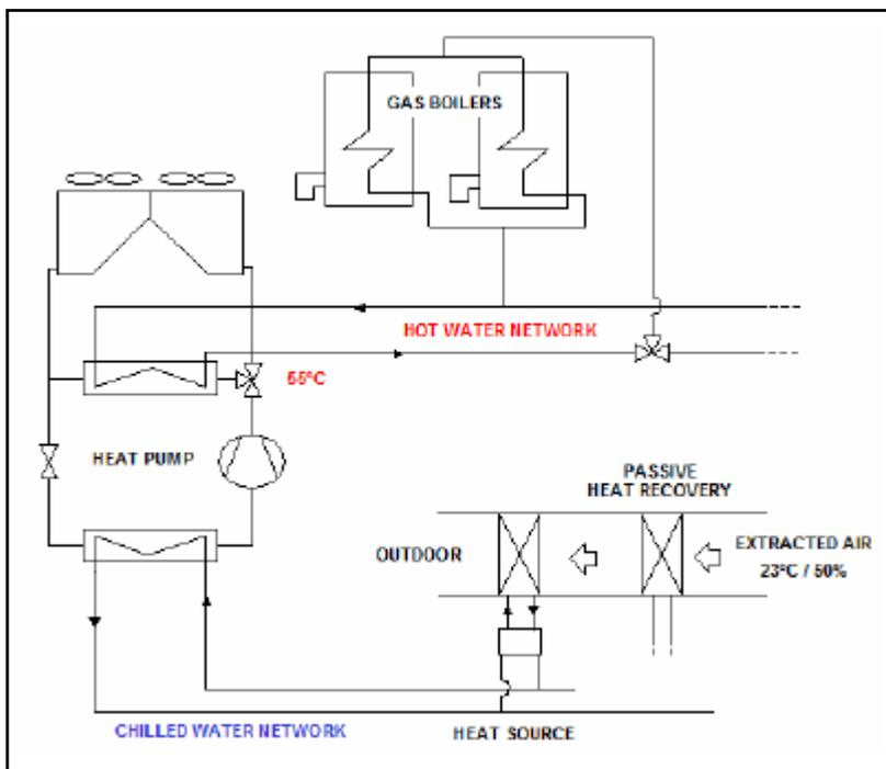
*Heat pumping using the extracted air as a heat source*
