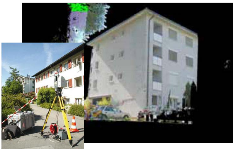
Figure 4. Existing buildings can be laser scanned. The result is a photorealistic 3-D-picture allowing the required measurements to be extracted.
