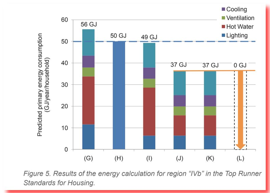
Figure 5. Results of the energy calculation for region "IVb" in the Top Runner Standards for Housing.
