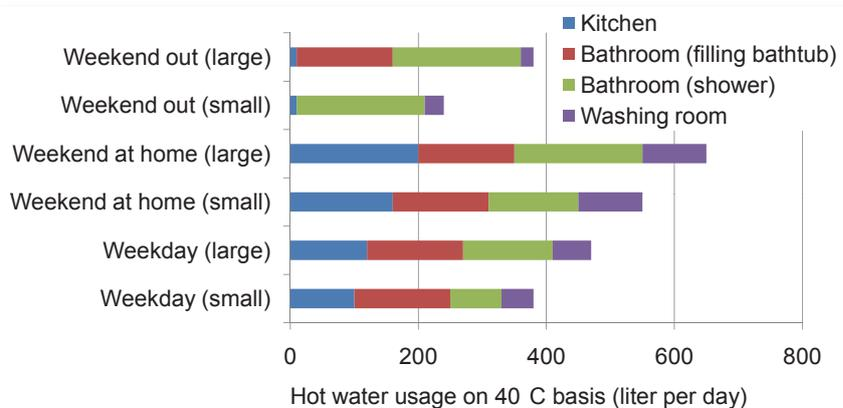
Figure 1. Domestic hot water usage pattern 'Corrected M-1 Mode' for 4-member family.
