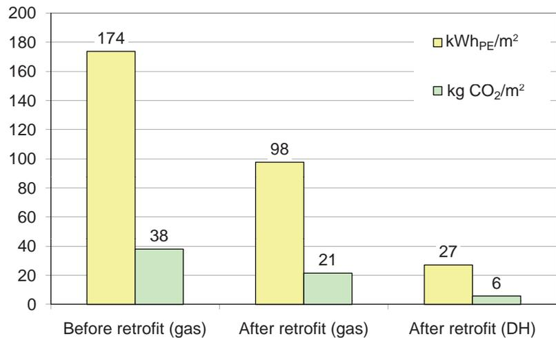
Figure 2. Karlsruhe-Rintheim neighbourhood refurbishment project - primary energy and CO<sub>2</sub> emissions for heating and domestic hot water supply
