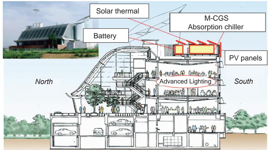
Figure 1. Various advanced technologies combined to achieve an energy efficient building.
