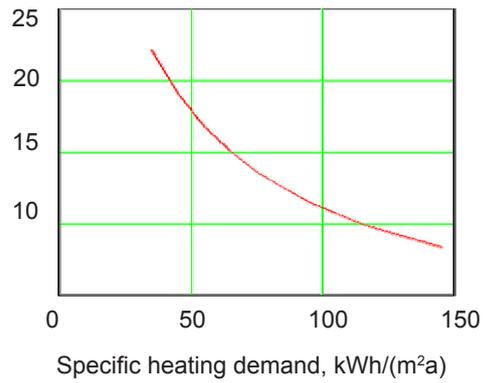
Figure 4. Line density as a function of energy retrofit standard (left) and the resulting specific costs of heat distribution (€/MWh, right). Line density is defined as the amount of thermal energy transported through the neighbourhood distribution grid in MWh/(m a).
