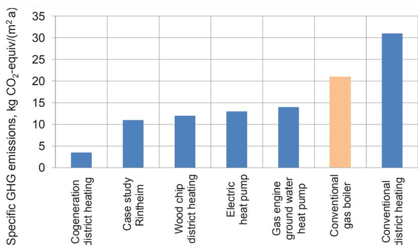
Figure 3. Comparison of optimized building retrofit measures combined with centralised or individual energy supply systems, in terms of GHG emissions (kg CO<sub>2</sub>-equiv/(m<sup>2</sup> a)).
