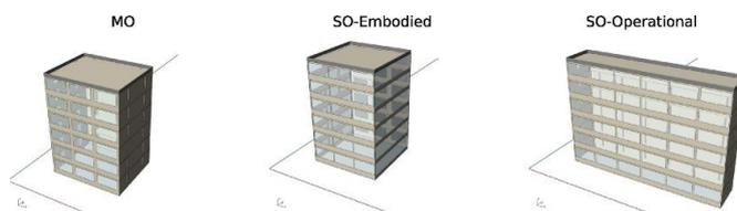
Figure 28: Optimized shape of the case study building depending on the objective (embodied / operational impact) and type of optimization (single-objective / multi-objective).
