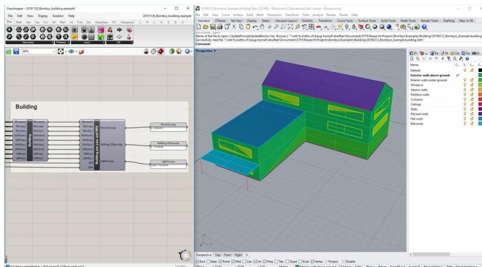
Figure 52: Bombyx plug-in in GH (left) and geometry with pre-defined layers (right).
