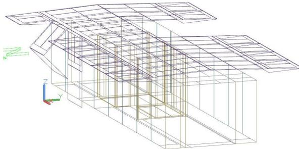
Fig. 7.47: Orthogonal projection of the Rooftop building's geometry model in active state as imported into EnergyPlus, reflecting PV and shutter positioning shown in Fig. 7.46.
