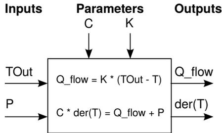
Fig. 6.1: Simple room model with air change model and externally defined heat source.
