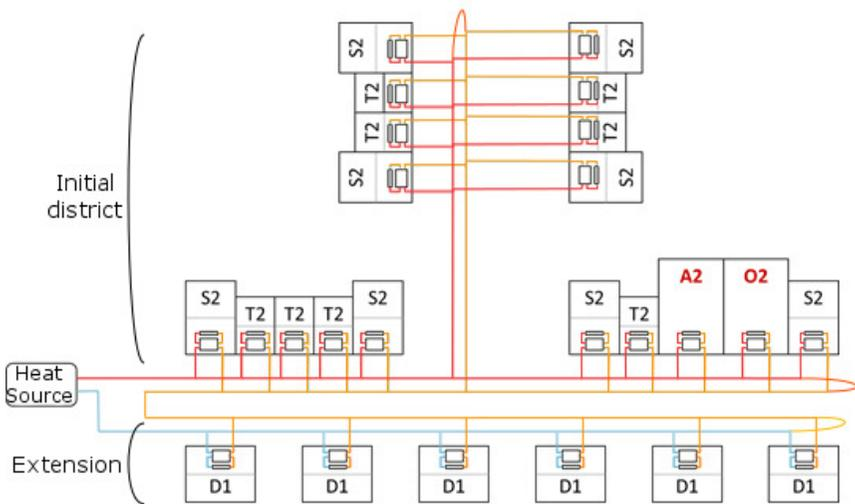
Fig. 10.29: Diagram of the studied district based on the Annex 60 Neighborhood Case. Red lines represent the supply flow, orange lines the intermediate flow, and blue lines the return flow. Buildings A2 and O2, in red, are assumed to belong to the municipality. The curves connecting supply and return lines represent the bypass valves.
