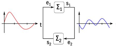
Fig. 6.10: Waveform relaxation algorithm for co-simulation.
