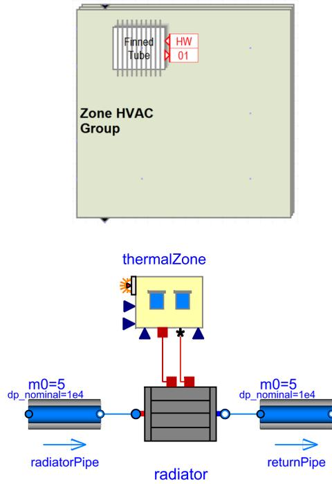
Fig. 7.30: Connection between a radiator and a thermal zone in SimModel and AixLib
