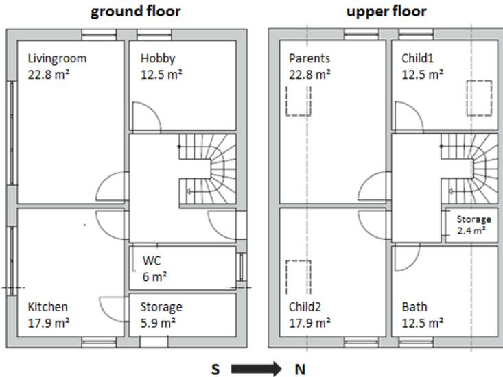
Fig. 9.24: Floor plan for the reference building
