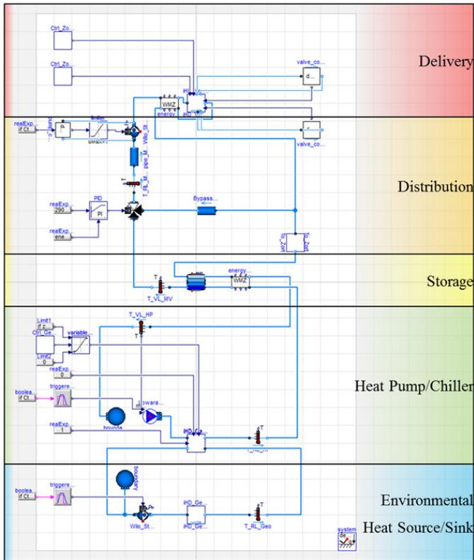
Fig. 9.6: Representation of the geothermal heat pump system of inHaus2 in Modelica
