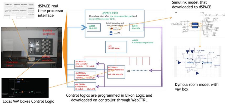
Fig. 11.14: Hardware in the loop workflow.
