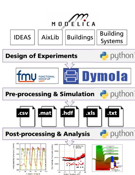
Fig. 8.1: Schematic of typical building simulation workflow to demonstrate use cases for Python based process automation
