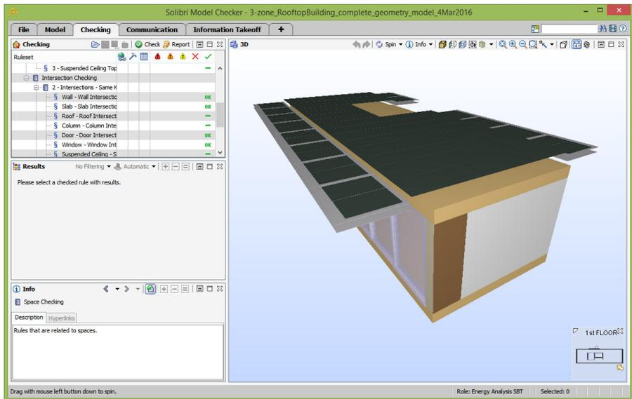
Fig. 7.44: Geometry model of the Rooftop building in Solibri Model Checker.
