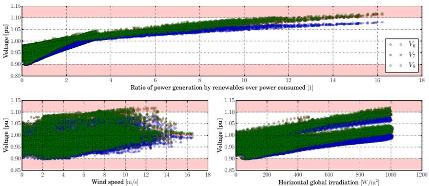
Fig. 10.31: Voltage levels in three different nodes of the neighborhood as a function of power generated by renewables, wind speed and horizontal global irradiation without feedback control.
