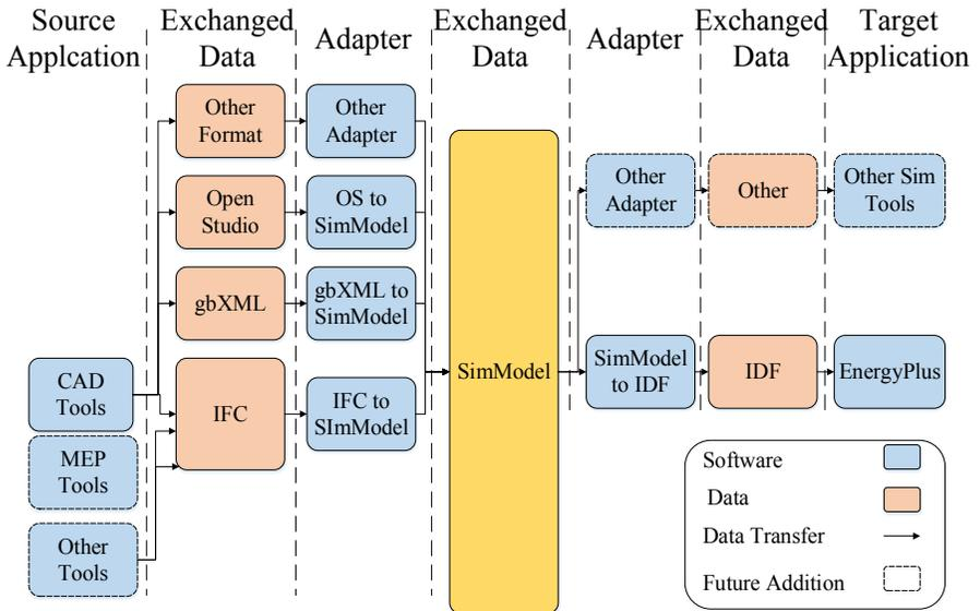
Fig. 7.14: Interoperable data exchange enabled by SimModel. This solution enables re-use of original project data as contained in IFC based BIM (bi-directional mapping) and data from other sources (import only)
