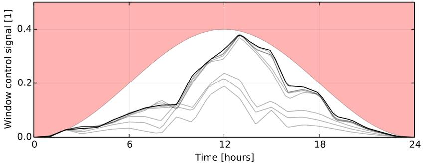
Fig. 9.36: Optimal control signal for the blind (black line) and its successive approximations for different values of  $\mu_i$  (gray lines).
