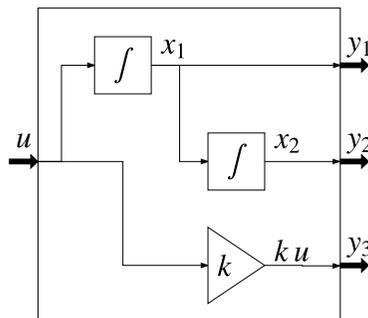
Fig. 14.1: Signal flow diagram that illustrates direct dependency.
