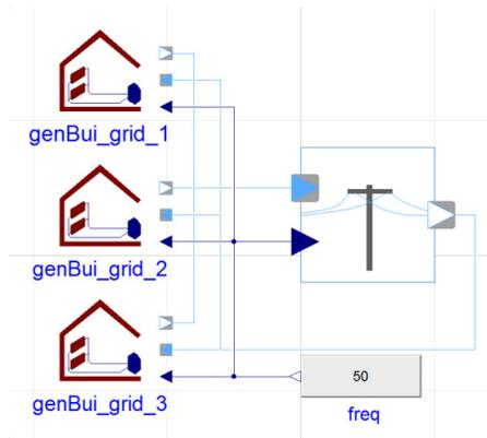
Fig. 10.34: Full simulation test case for 3 grid-connected buildings in Dymola.
