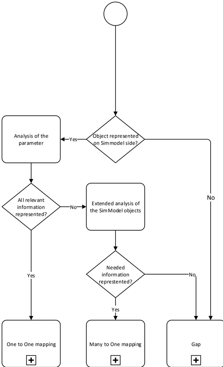
Fig. 7.23: BPMN process diagram for the object mapping
