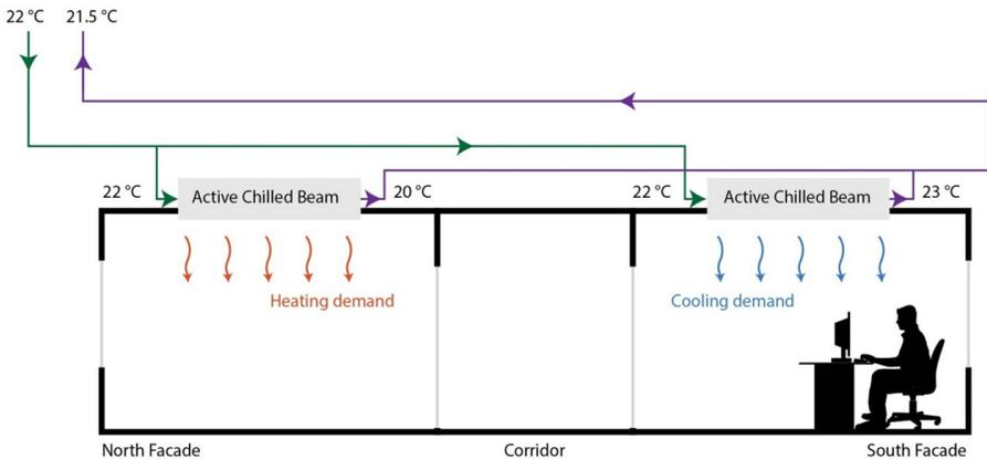
Fig. 9.17: Two-pipe active chilled beam system for simultaneous heating and cooling
