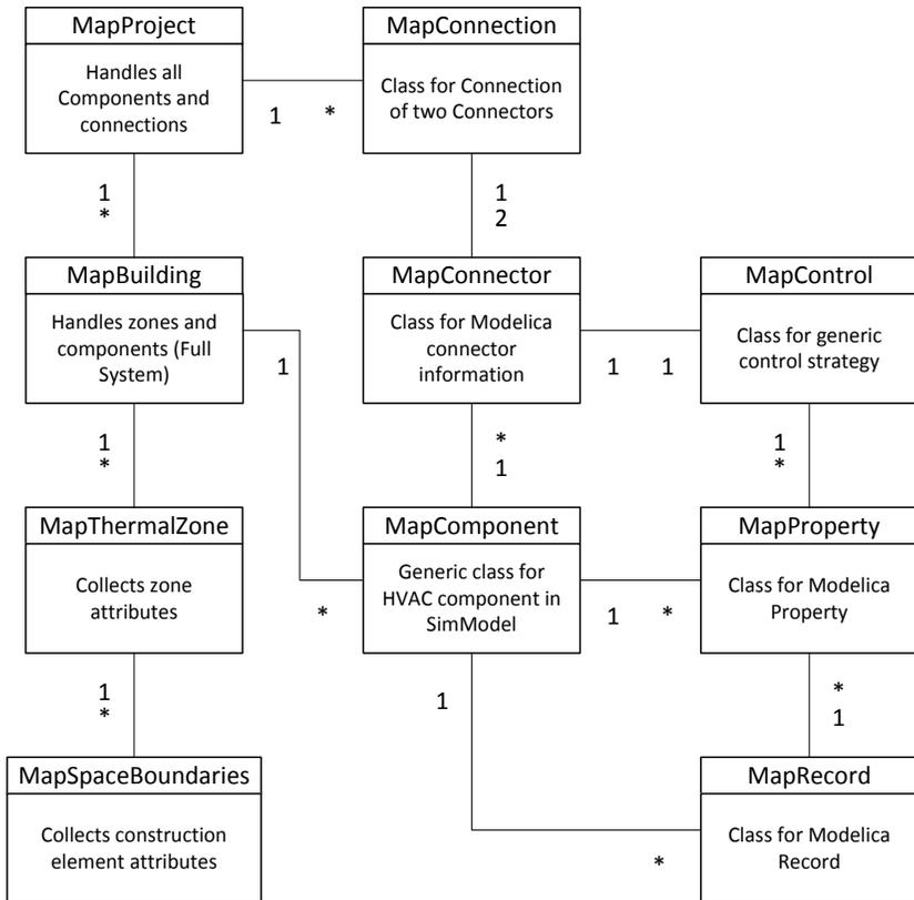
Fig. 7.25: UML diagram for the high-level API.
