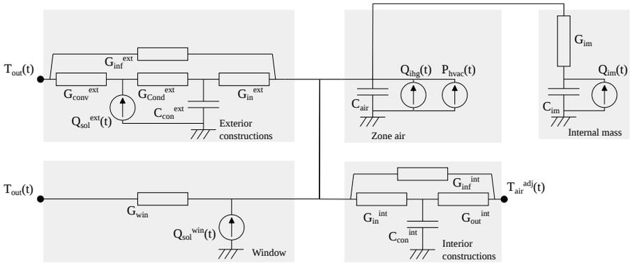
Fig. 9.29: Simplified model of a thermal zone.
