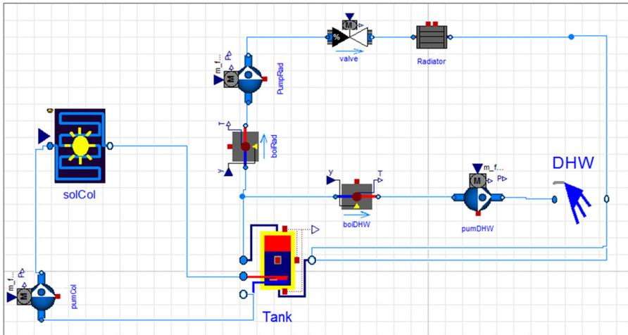
Fig. 9.21: Heating system schematic
