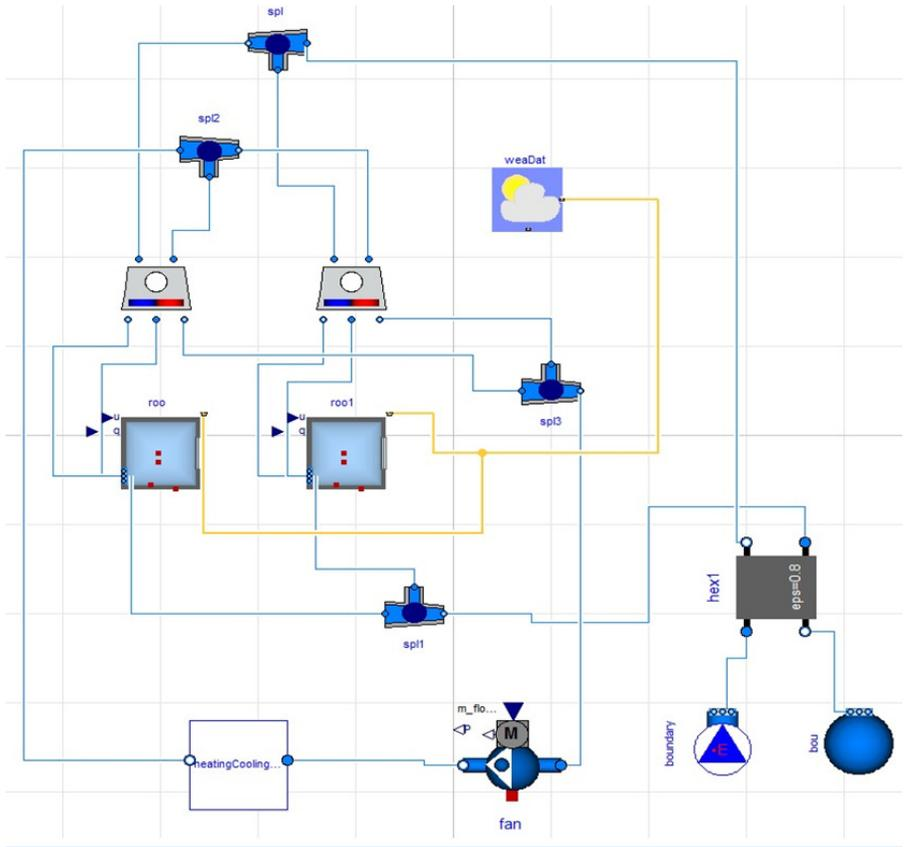
Fig. 9.18: Modelica model of the building system
