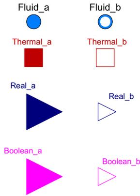
Fig. 7.27: Different connector types in Modelica (graphical representation).
