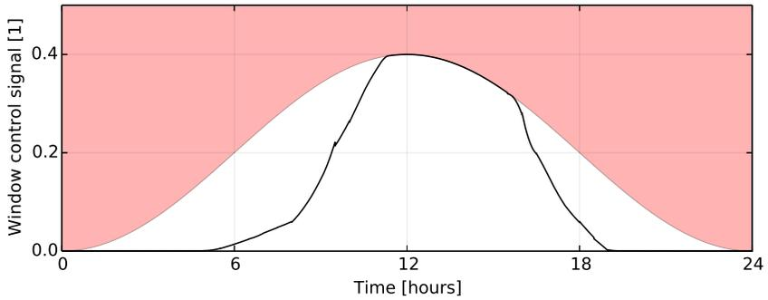
Fig. 9.32: Optimal control signal for the blind (black line).
