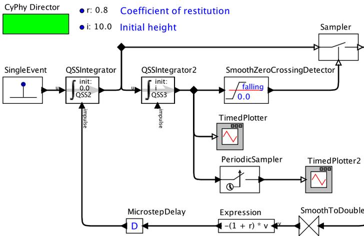
Fig. 6.9: CyPhySim model of a bouncing ball with QSS integration.
