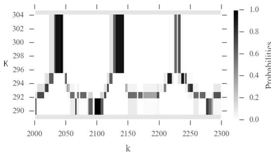
Fig. 11.9: Qualitative state trajectory of the air outlet temperature  $T_{air,out}$  (nominal condition).
