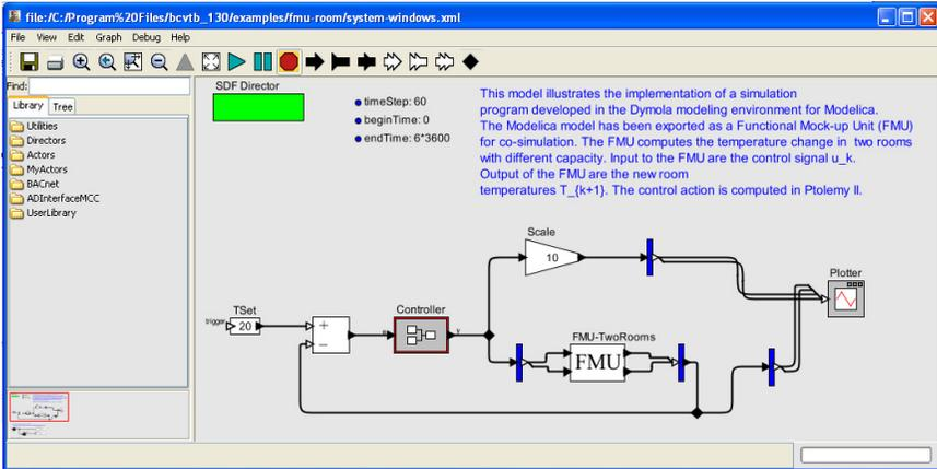
Fig. 6.7: The BCVTB is used to couple a controller implemented in Ptolemy II with a room model implemented in Dymola and exported as an FMU.
