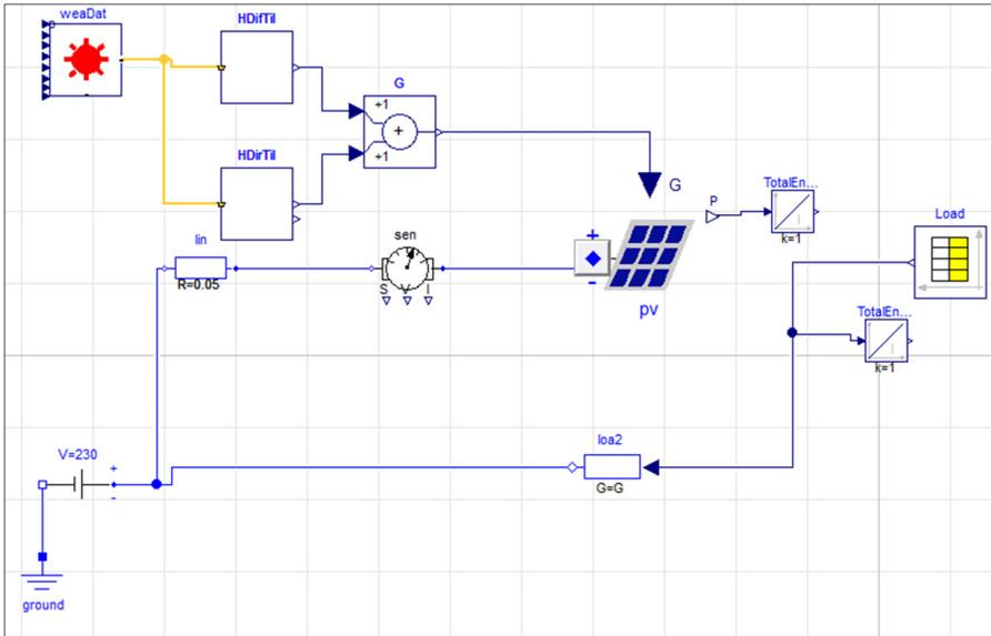
Fig. 9.22: Electric model containing the weather data, PV and the load profile
