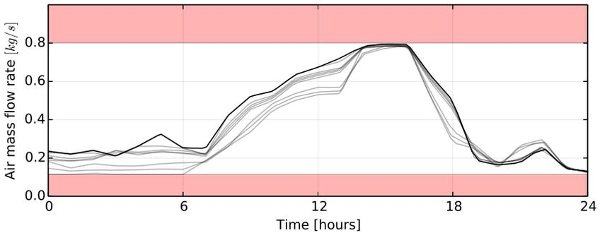
Fig. 9.37: Optimal supply air mass flow rate (black line) and its successive approximations for different values of  $\mu_i$  (gray lines). The red areas indicate the infeasible regions.
