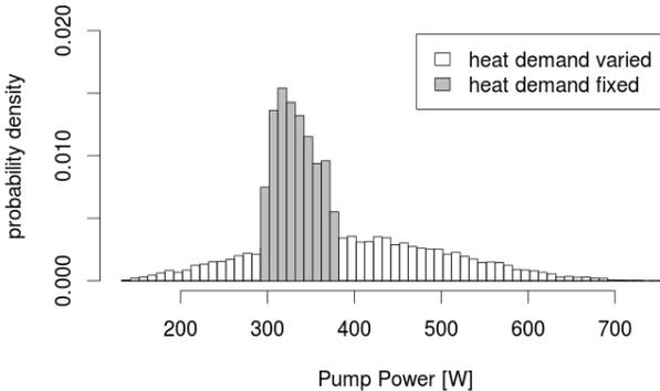
*Fig. 7.8: Distribution of the pump power over all simulation runs. White bars correspond to a varied heat demand according to the building parameter distributions given in [Table 7.1](#). Gray bars correspond to a fixed heat demand and only HVAC parameters are varied according to [Table 7.1](#).*
