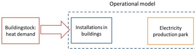
Fig. 9.8: The interaction between the heating and cooling systems in buildings and the electricity production park was studied with an operational model which has information of both systems [Bal13].
