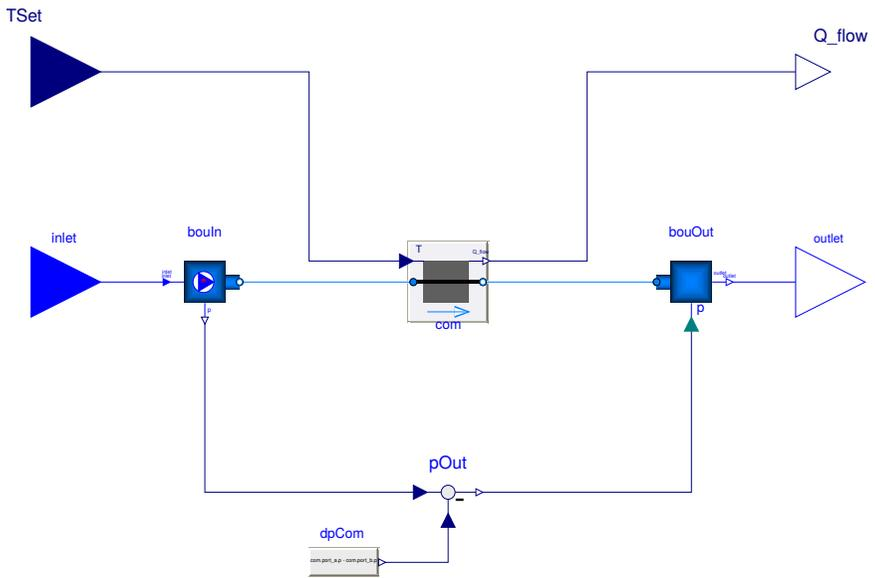
Fig. 6.11: Modelica block that can be used to export a heater that has acausal fluid ports as an FMU.
