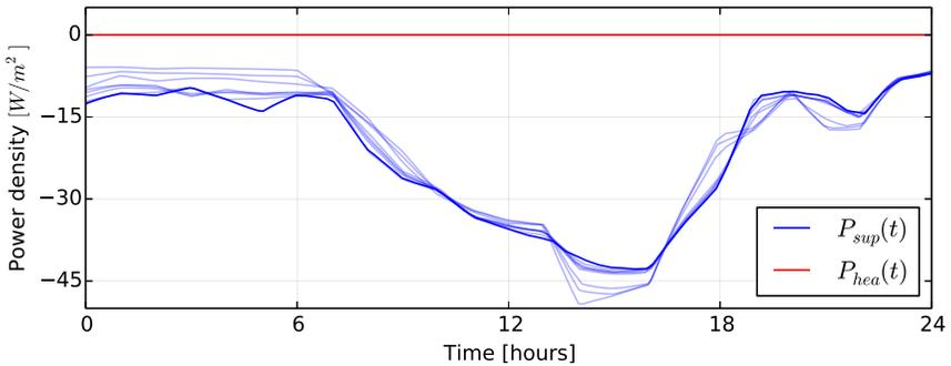
Fig. 9.35: Optimal cooling power provided by the HVAC system through the VAV box (blue line) and its successive approximations for different values of  $\mu_i$  (light blue lines), and optimal heating power provided by the VAV box (red line).
