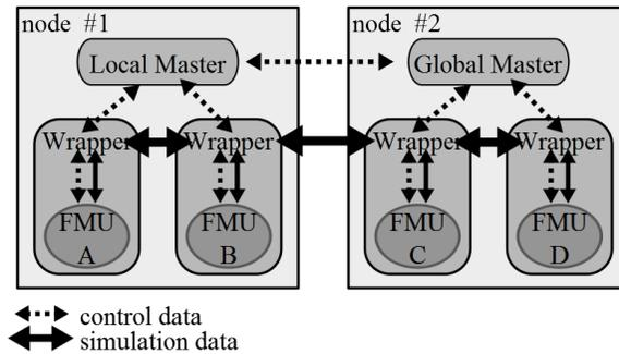
Fig. 6.8: Co-simulation architecture components in DACCOSIM.
