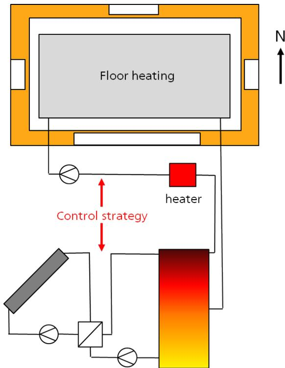
Fig. 9.38: Residential building with its solar heating system
