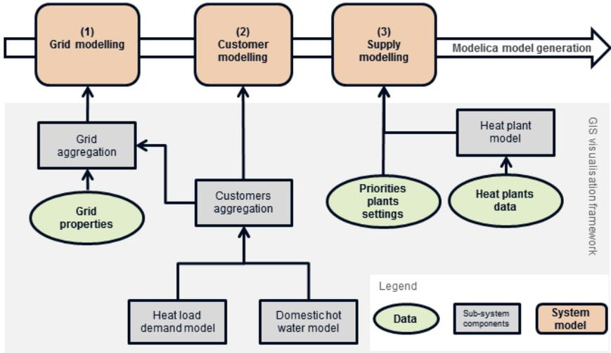
Fig. 10.6: Methodology flow diagram: example for a large district heating network
