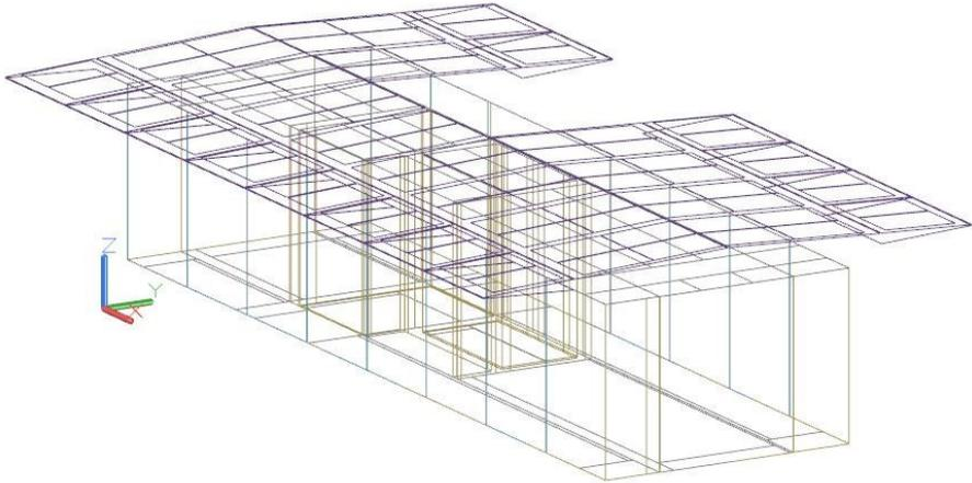
*Fig. 7.45: Geometry model of the Rooftop building in passive state as imported into EnergyPlus, showing space boundaries, PV panels and shutters in their original position.*
