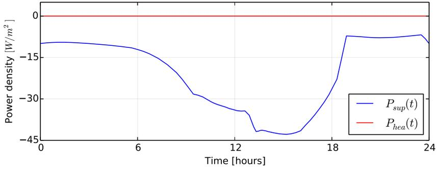
Fig. 9.31: Optimal cooling and heating power provided by the HVAC system through the VAV box.
