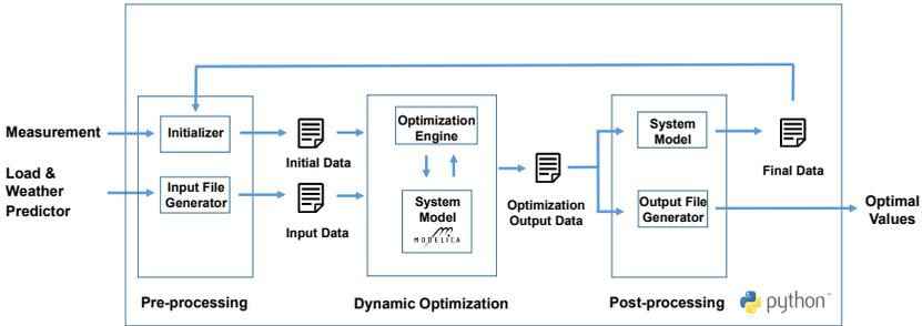
Fig. 11.2: MPC for chiller plants workflow.
