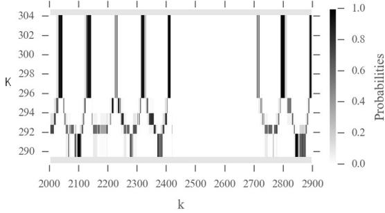
Fig. 11.10: Qualitative state trajectory of the air outlet temperature  $T_{air,out}$  (faulty condition).
