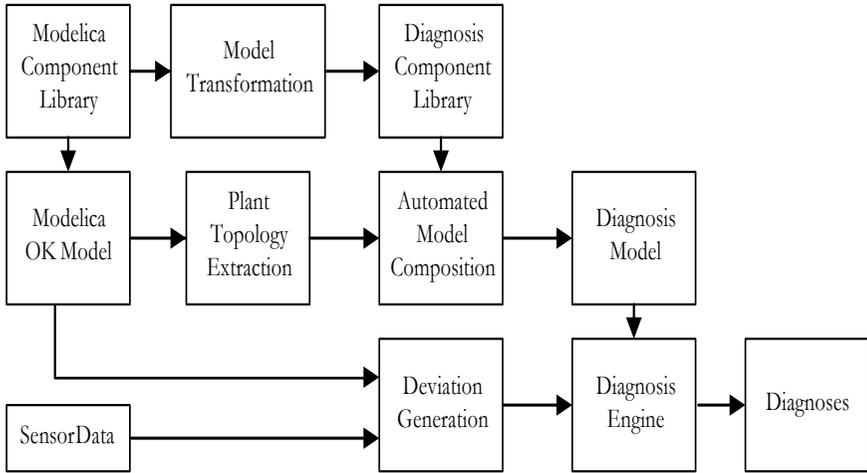
Fig. 11.12: Fault Detection of Air Handling Unit Components in a Qualitative Approach Workflow.
