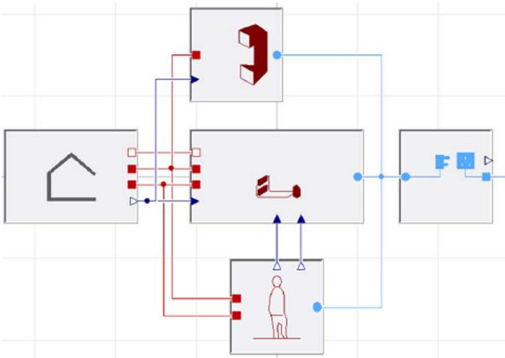
Fig. 9.13: General layout of the Modelica system simulation model, using the IDEAS-library. Left: building structure. Top: air handling unit. Center: heating/cooling production system. Bottom: internal gains due to occupancy. Right: electrical grid.
