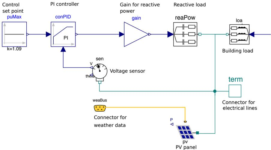
Fig. 10.33: Electrical circuit with reactive power control at the PV inverter.
