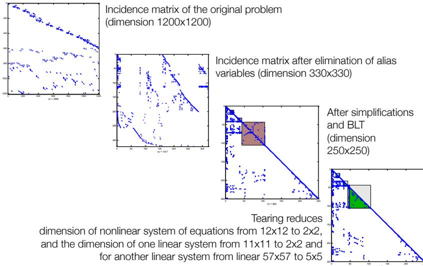
Fig. 5.8: Reduction of the dimension of the system of equations for the case of a mechanical model during the symbolic processing.
