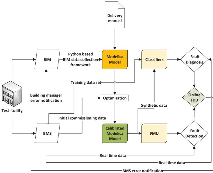
Fig. 11.13: Fault Detection of Air Handling Unit Systems in a Quantitative Approach Workflow.
