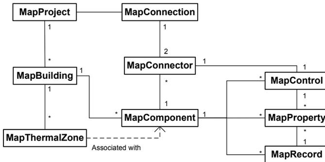
Fig. 7.32: Simplified UML diagram of the Python classes used for applying information from libSimModel API and topology mapping.
