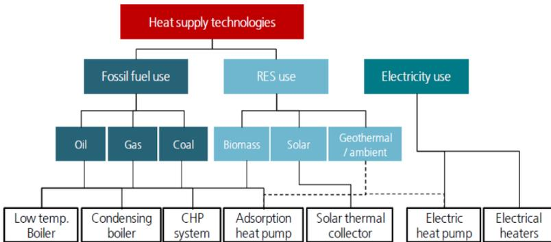
Fig. 10.1: Overview of heating technologies and their respective energy sources. Source [Com16b].
