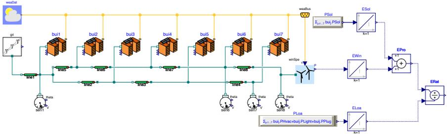
Fig. 10.30: Neighborhood model with renewable energy sources. The yellow lines are weather data, green lines are electrical lines, and dashed blue lines are for post-processing.
