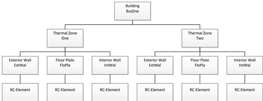
Fig. 5.3: Hierarchical structure of a thermal building model with levels for building, thermal zones, wall elements and RC-elements.
