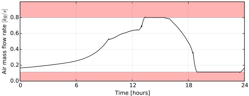
Fig. 9.33: Optimal supply air mass flow rate. The red areas indicate the infeasible regions.
