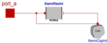
Fig. 5.5: Diagram view of a thermal network for interior walls, consisting of an array of thermal resistances and capacities.
