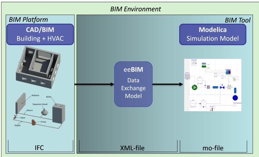
Fig. 7.6: Data transformation from BIM to Modelica
