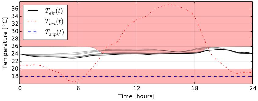
Fig. 9.34: Resulting optimal zone air temperature (black line) and its successive approximations for different values of the penalty function multiplier  $\mu_i$  (gray lines).
