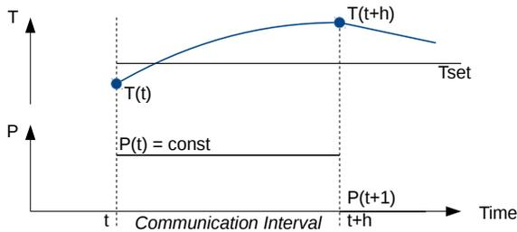
Fig. 6.2: Illustration of room air temperature exceeding the set point temperature due to delayed variable exchange.
