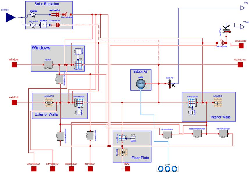
Fig. 5.4: Diagram view of a thermal zone model with three wall elements (exterior walls, interior walls and floor plate), windows and indoor air volume.
