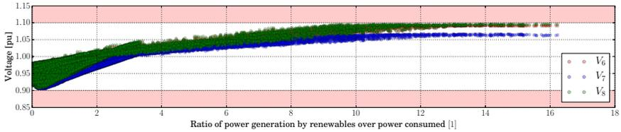
Fig. 10.32: Voltage levels in three different nodes of the neighborhood as a function of power generated by renewables with feedback control that adjust room air temperature setback and reactive power control at all PV inverters.
