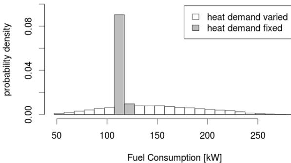
*Fig. 7.7: Distribution of the fuel consumption over all simulation runs. White bars correspond to a varied heat demand according to the building parameter distributions given in [Table 7.1](#). Gray bars correspond to a fixed heat demand and only HVAC parameters are varied according to [Table 7.1](#).*
