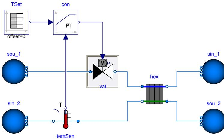
Fig. 5.6: Model with heat exchanger, feedback control and replaceable valve. The gray background rendered around the valve indicates visually that this model can be replaced by another implementation.
