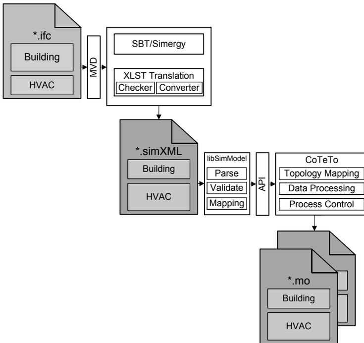
Fig. 7.16: Overview of the transformation tool-chain from IFC to SimXML and Modelica model
