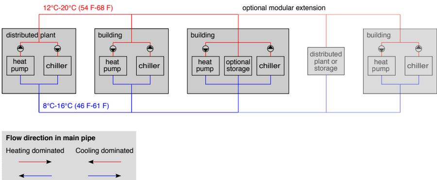
Fig. 10.4: Bi-directional thermal network.
