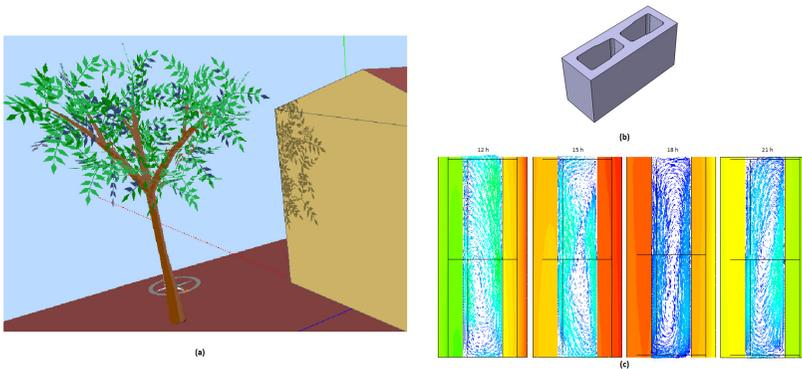
Fig. 6.4: The use of pixel counting technique for accurate and fast evaluation of complex shading (a) at an external surface due to a non-planar tree. (b) The hollowed block used in the wall ANSYS CFX co-simulation and (c) the preliminary results.
