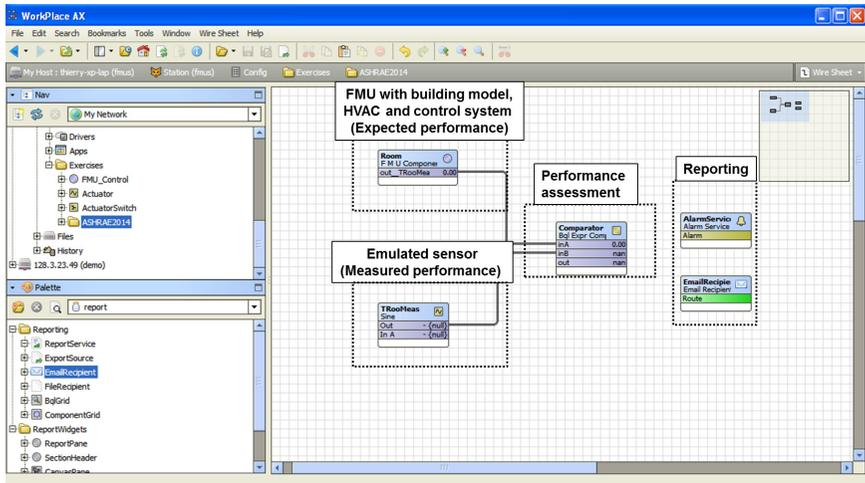
Fig. 6.3: Simulation-based performance monitoring in which an FMU is imported in NiagaraAX.
