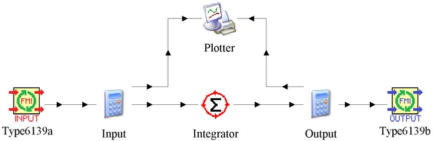
Fig. 6.6: Example of a TRNSYS model containing blocks of Type6139 for FMU export.
