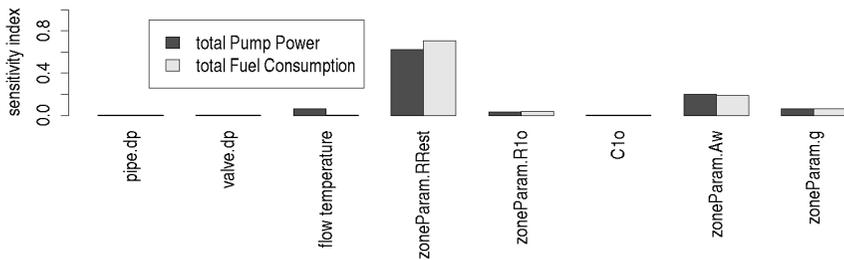
*Fig. 7.9: Sensitivity indices for the outputs fuel consumption and pump power with respect to the varied input parameters. The variation of the building parameters has much more effect on the outputs than the variation of the parameters concerning the HVAC layout.*
