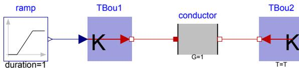
*Fig. 5.2: Thermal conductor with varying temperature boundary conditions.*
