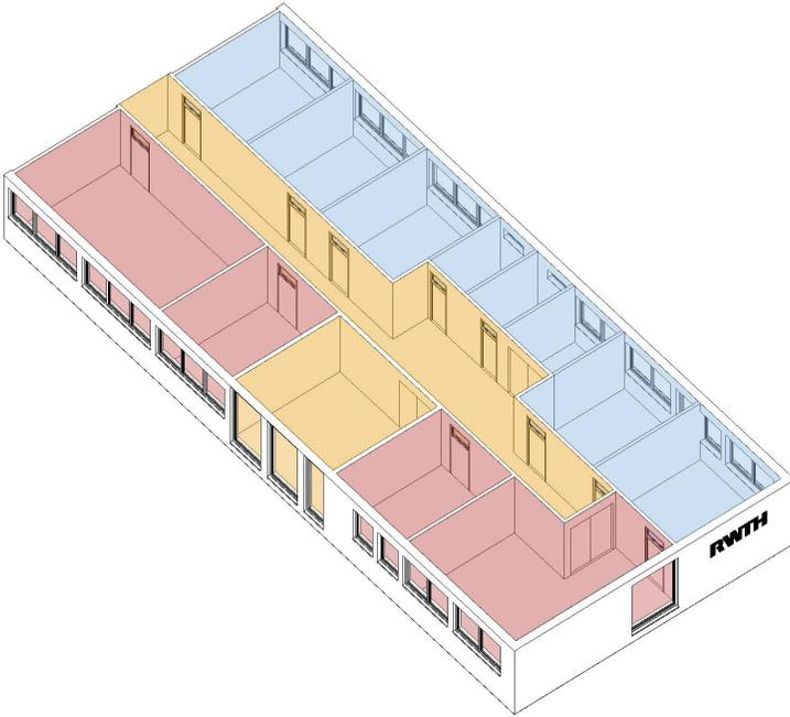
*Fig. 7.42: Thermal zones for the western and eastern offices and for the corridor, defined in Revit 2016.*
