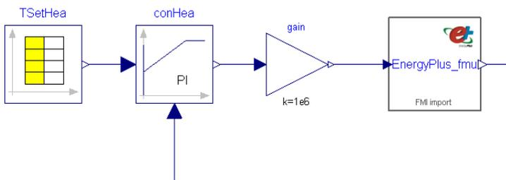
Fig. 6.5: An EnergyPlus room model has been exported as an FMU. This FMU is coupled to a controller implemented in a Modelica simulation environment.
