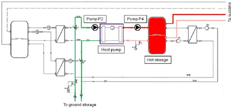
Fig. 9.12: Production unit in heating mode
