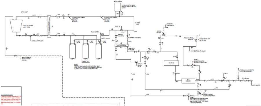
Fig. 9.15: Schematic of the HVAC and domestic water system
