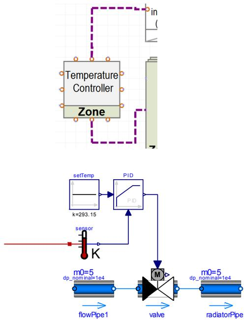
Fig. 7.31: Temperature controlled valve in SimModel and AixLib.
