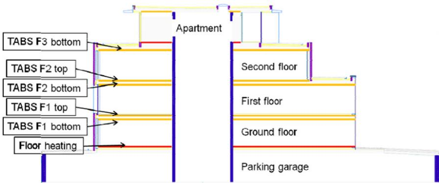
Fig. 9.11: Scheme of the thermally activated building components (floor heating: red, TABS: yellow)
