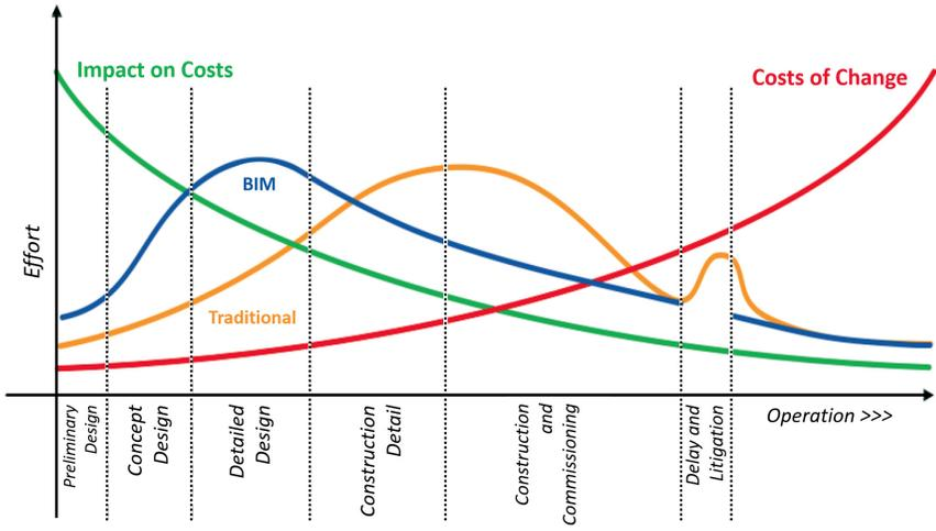
Fig. 7.1: Comparison between BIM-based workflow and traditional workflow (Adapted from [EHLP13]).
