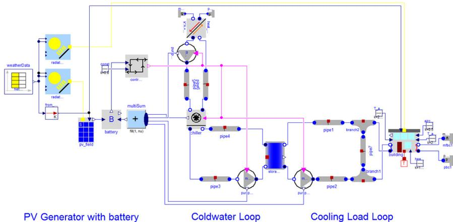
Fig. 9.3: Plant diagram of the PV cooling system, based on the Modelica BuildingSystems library
