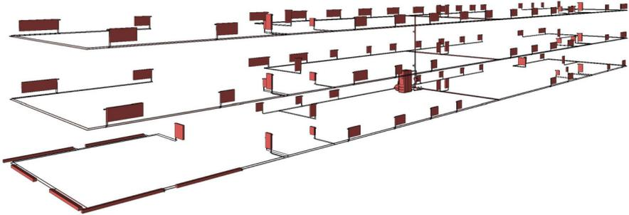
Fig. 7.41: Whole heating system of use case five, modelled with Revit 2016.
