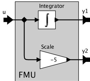
Fig. 4.1: FMU for which output  $y_1$  does not have a direct dependency on input  $u$  but output  $y_2$  does.
