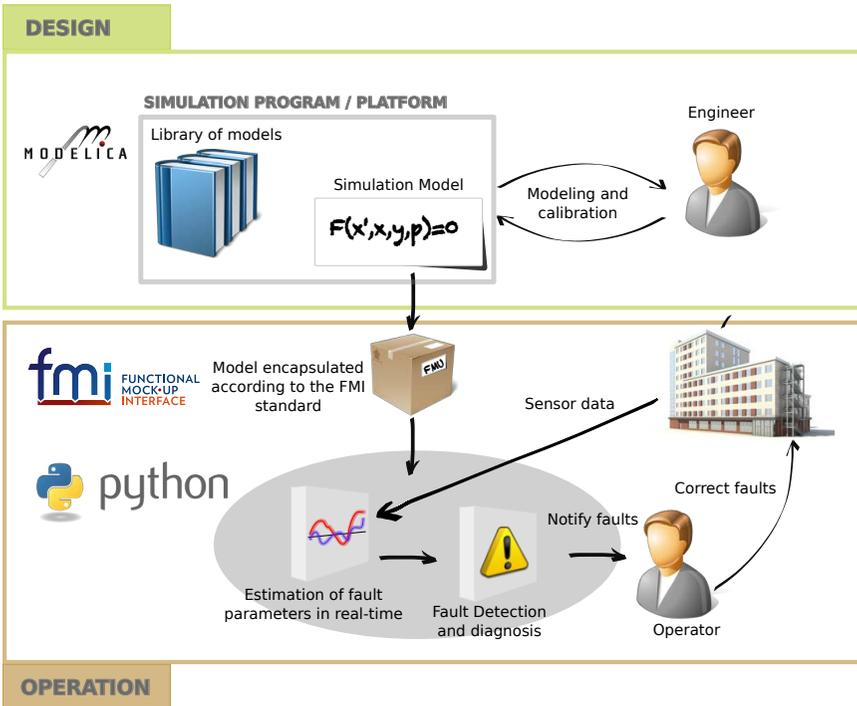
Fig. 11.4: Model-based fault detection using state estimation techniques compliant with the FMI standard.
