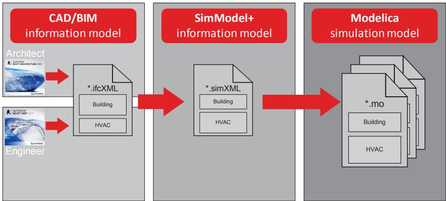
Fig. 7.5: Overview of the transformation process from IFC to Modelica models using different Modelica libraries.
