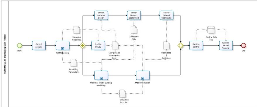
Fig. 11.3: MPC for energy control of underground public spaces workflow.
