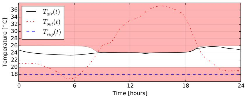
Fig. 9.30: Optimal room air temperature (black line), thermal discomfort zone (red area), outside temperature (red dotted) and supply air temperature (blue dashed).
