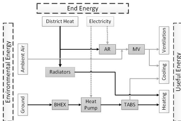
Fig. 9.5: HVAC Schematic of inHaus2: AR-Adsorption Refrigeration, MV-Mechanical Ventilation, BHEX-Borehole Heat Exchanger
