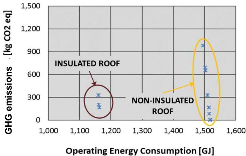
**Figure 22:** Embodied GHG emissions against Final Operating Energy Consumption of the 10 optimal solutions in Mediterranean climate
