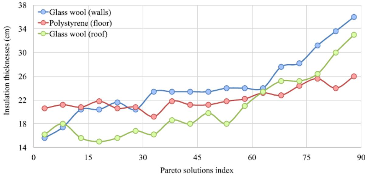
**Figure 5:** Evolution of the insulation thicknesses for decreasing GHG emissions (Pareto solutions)
