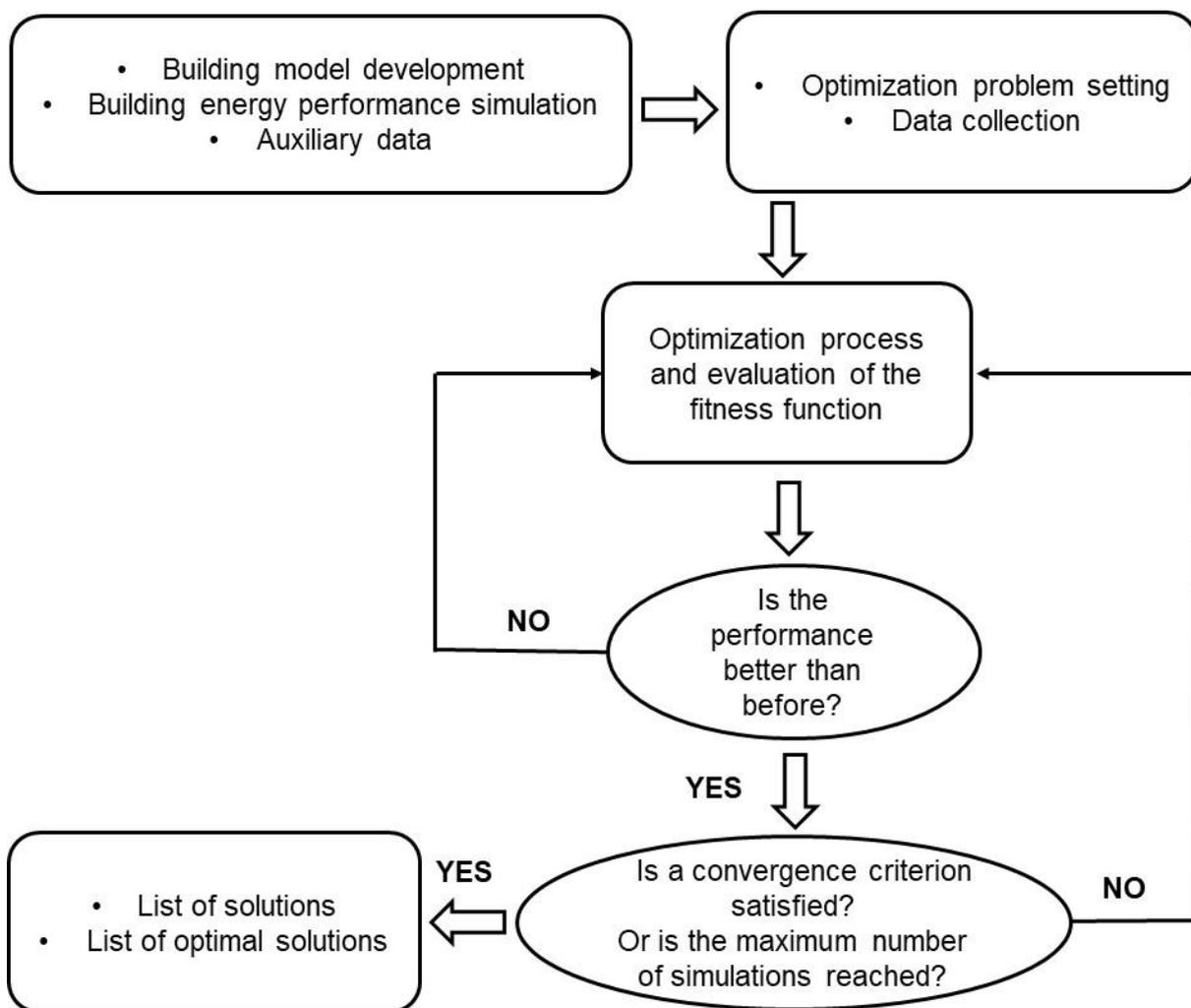
**Figure 1:** General workflow for the optimisation process of buildings
