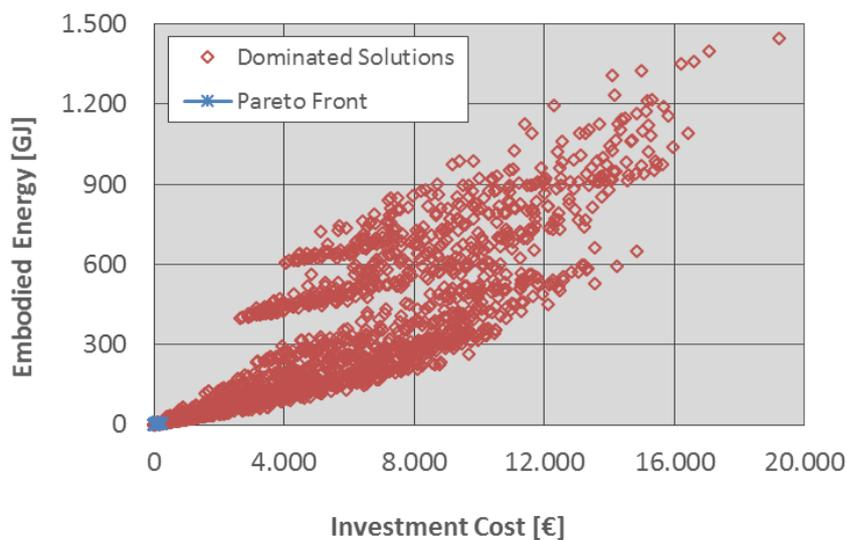
**Figure 23:** Values of the embodied PE and investment cost objective functions for the 2016 assessed buildings (red circles) and for the optimal solutions in the Pareto front (blue crosses) in Mediterranean climate
