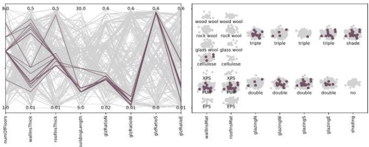
**Figure 7:** Optimal values of variables in the multi-objective optimisation study
